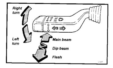
Headlamp Flasher: The headlamp flasher is operative at all times. If the lever is pulled towards the steering wheel against spring pressure, the headlamp main beams will light.
