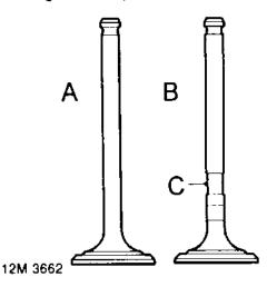
NOTE: Two types of exhaust valve may be fitted, standard valves, A in illustration or carbon break valves, B in illustration. Carbon break valves may be identified by the machined profile C on the valve stem. To prevent exhaust valves from sticking, standard valves should be replaced with carbon break valves during engine overhaul.
