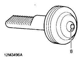
8. Remove and discard screw securing piston to rack, remove and discard piston and seal assembly.
