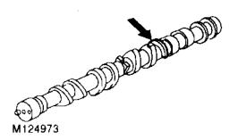
CAUTION: Camshafts fitted to later engines incorporate a reluctor ring, these camshafts are not interchangeable with those fitted to early engines. Commencing engine numbers for the modified camshafts are listed in Information.
