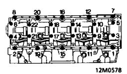
Using sequence shown, progressively slacken 22 bolts securing camshaft carrier to cylinder head until valve spring pressure is released; remove bolts.
