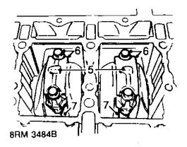
4. Rotate crankshaft to bring Numbers 2 and 3 pistons to BDC.
