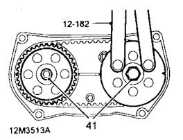
41. Restrain each timing gear in turn using tool 12-182 and tighten bolts to 65 Nm.
