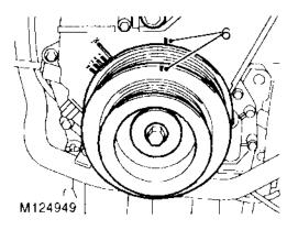
Check that timing mark on crankshaft pulley is aligned with mark on timing belt lower cover.
