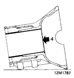
CAUTION: If original cylinder liners are to be refitted, use a felt tipped pen to make suitable alignment marks between liner. and cylinder block. Do not etch or stamp liners.
