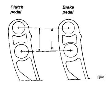
7. Refit in reverse order to removal, adjusting the brake pedal pushrod as detailed in sub-section JI.7 and the clutch pedal in a similar manner. The throttle pedal upstop should be adjusted as follows:
