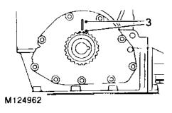
Check that crankshaft gear timing marks are aligned with flange on oil pump - 90° BTDC.
