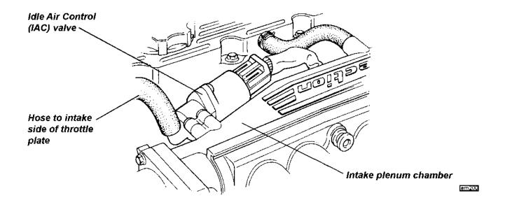
To remove the valve, unplug the harness connector and remove the two Torx screws securing the valve body to the plenum adaptor. Withdraw the valve and discard the 'O' ring.
