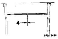
Check new ring fitted gap 20 mm from top of cylinder liner bore:
