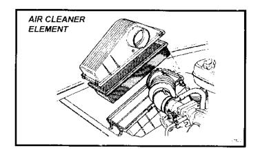
A disposable folded paper type air cleaner element is fitted in a housing at the left hand side of the engine bay. To replace the filter element, leave the hose attached, and release the four over-centre clips securing the top cover of the air filter housing. Raise the cover and ensure that the filter element remains in the lower housing before swinging the cover aside. Lift out the element and clean the inside of the filter housing and cover, including the joint line recess.
