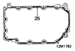
25. Apply a 2 mm wide x 0.25 mm thick continuous bead of sealant, Part Number GUG 705963GM to sump flange as shown then spread to an even film using a roller.
