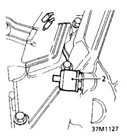
Remove reverse light switch; discard sealing washer.
