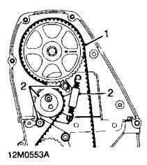
1. Remove and discard camshaft timing belt.
