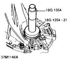
25. Fit new differential oil seals in gear case.
