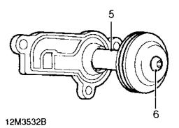
5. Slide piston end of rack through seal.
