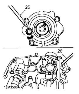
26. Using a screwdriver, rotate control shaft as far as possible in an anti-clockwise direction, viewed from front of camshaft carrier.
