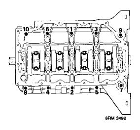
7. Lubricate main journals with engine oil. Fit bearing ladder to block, fit bolts ensuring that flanged head bolt is fitted at position 10. Tighten bolts in sequence shown to 5 Nm then in same sequence to 30 Nm.
