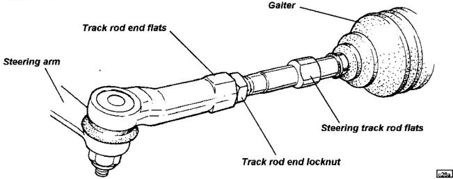
Note that in order to preserve the required bump steer characteristic and steering symmetry, the effective length of each track rod must remain equal - adjust each track rod by a similar amount:
