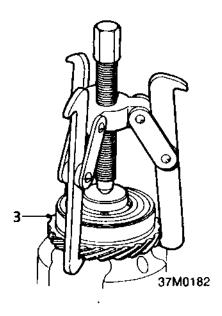
Remove speedometer drive gear using a suitable three legged puller and thrust button.
