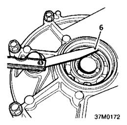
6. Using feeler gauges measure and record clearance between circlip and bearing outer face.
