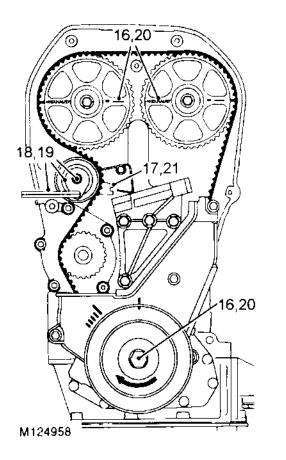
Using crankshaft pulley bolt, rotate crankshaft 2 turns clockwise and align camshaft gear timing marks.
