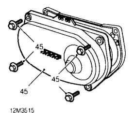
45. Fit rear timing belt cover, fit and tighten screws to 10 Nm.
