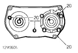
20. Fit rear timing belt backplate, fit and tighten bolts to: M5 bolts - 6 Nm M6 bolts - 10 Nm.
