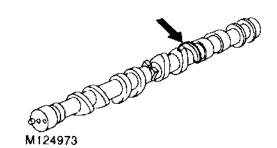
NOTE: Later engines are fitted with modified camshafts which incorporate a reluctor ring and the procedure for removing cylinder head bolts differs from early engines. Commencing engine numbers for the modified camshafts are listed in information.
