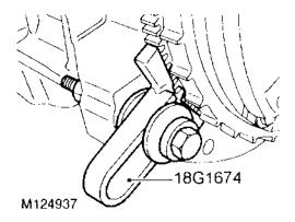
7. Fit flywheel locking tool 18G 1674, tighten bolt.
