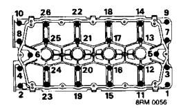
4. Fit camshaft carrier, fit and progressively tighten bolts, in sequence shown, to 10 Nm.
