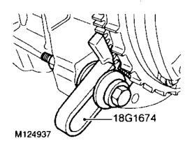
8. Fit flywheel locking tool 18G 1674, tighten bolt.
