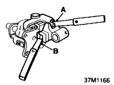
NOTE: Modified interlock assembly illustrated. This assembly may be fitted as a replacement to early gearboxes but modified interlock assemblies fitted to gearboxes having Serial Number prefixes C4BP and C6BP have uprated springs and must not be interchanged with modified interlock assemblies fitted to other gearboxes.
