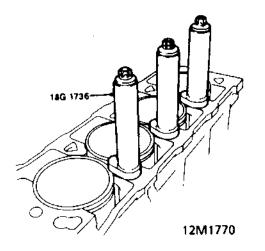
Assemble cylinder liner retainer clamps 18G 1736 to cylinder head bolts. Position retainer clamps on cylinder liners ensuring clamps do not protrude over liner bores. Screw cylinder head bolts into oil rail and tighten sufficiently to retain clamps.
