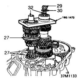
27. Move synchro sleeve to engage 1st and 4th gears.
