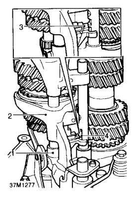
To prevent any further movement of the 3rd/4th synchro sleeve (5) and engagement of 4th gear, the spring on the lock plate (3) moves the lock plate into the machined groove (7) above the abutment (4).
