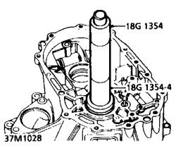
5. Fit a new input shaft oil seal in differential housing using tools 18G 1354 and 18G 1354-4.
