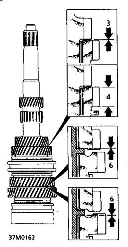
Using feeler gauges, measure clearance between 2nd and 3rd gears.
