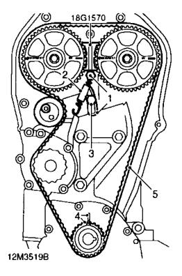
NOTE: K16 non VVC engine illustrated. On VVC engines, tensioner spring and pillar bolt are supplied with replacement timing belt.
