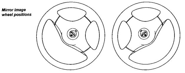
3. Secure the steering wheel before road testing the car and marking the actual 'straight ahead' position of the steering wheel which should deviate from the ideal position by less than 5°. Final alignment is achieved by asymmetric adjustment of the track rods, retaining the overall toe-out setting.
