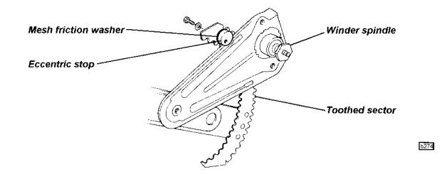
4. To adjust the fully up position of the glass, the eccentric stop on the toothed sector of the winder mechanism must be rotated as necessary. A mesh friction washer is fitted between the eccentric and the sector to help retain adjustment.
