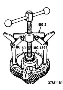
1. Remove bearings using tools 18G 2, 18G 2/3 and 18G 1397; discard bearings.
