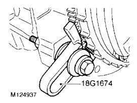
5. Fit flywheel locking tool 18G 1674, tighten bolt.
