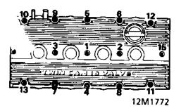
Fit camshaft cover on to camshaft carrier, fit bolts and tighten in sequence shown to 10 Nm.
