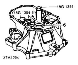
Fit input shaft bearing into differential housing using tools 18G 1354 and 18G 1354-6.
