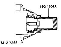
19. Fit new front and rear VVC housing oil seals using tool 18G 1604A.
