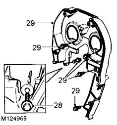
NOTE: Timing belt rear cover fitted to engine with 5 bolt front engine mounting illustrated.
