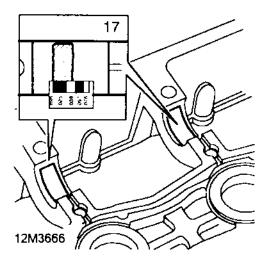
17. Measure widest portion of Plastigage on each inlet camshaft journal on camshaft carrier: Inlet camshaft bearing journal clearances:
