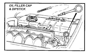
Topping Up: If topping up is necessary, remove the oil filler cap from the cam cover, and in order to allow the crankcase to ventilate, remove the dipstick. Add a suitable quantity of a recommended engine oil (see 'Recommended Lubricants') taking care not to spill any oil onto engine or electrical components; use a funnel if necessary.
