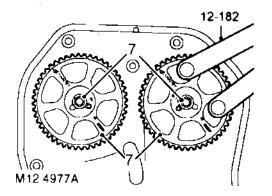
Fit camshaft gears to their respective camshafts ensuring that drive gear pins are located in correct slot in drive gears, hold gears using tool 12-182, fit and tighten bolts to 65 Nm.
