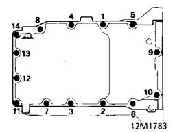
32. Using sequence shown, tighten 14 bolts to: M8 x 25 - 25 Nm M8 x 60 - 30 Nm
