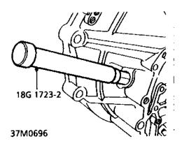
5. Outer bush: Using tool 18G 1723-2, drift outer bush into differential housing.
