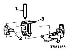
NOTE: A modified interlock assembly having 2 springs has been introduced; this assembly may be fitted as a replacement to early gearboxes.
