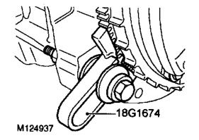
1. Fit flywheel locking tool: Flywheel without reluctor ring use 18G 1571. Flywheel with reluctor ring use 18G 1674.
