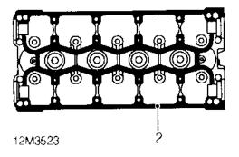
2. Apply continuous, thin beads of sealant, Part Number GUG 705963GM to paths on cylinder head as shown then spread to an even film using a roller.
