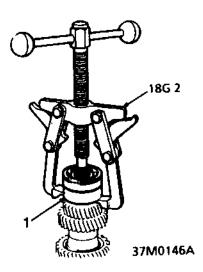
1. Remove bearings using tool 18G 2, note type of bearing fitted; discard bearings.
