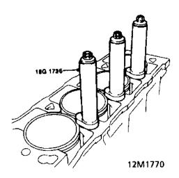
22. Assemble cylinder retainer clamps 18G 1736 to cylinder head bolts. Position retainer clamps on cylinder liners ensuring that clamps do not protrude over liner bores. Screw cylinder head bolts into oil rail and tighten sufficiently to retain clamps.
