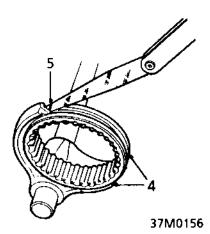
Assemble each selector fork to its respective synchro sleeve.
