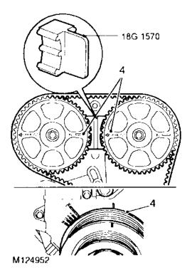
Rotate crankshaft clockwise to align camshaft gear timing marks - 90° BTDC.
