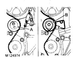
NOTE: Two types of timing belt tensioner are fitted to K16 engines, type A is a manual tensioner fitted to some K16 non VVC and all VVC engines. Type B is an automatic tensioner fitted to some K16 non VVC engines. Commencing engine numbers for the automatic tensioner are listed in information. The tensioners and their timing belts are not interchangeable.
