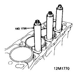
23. Assemble cylinder liner retainer clamps 18G 1736 to cylinder head bolts. Position retainer clamps on cylinder liners ensuring clamps do not protrude over liner bores. Screw cylinder head bolts into oil rail and tighten sufficiently to retain clamps.
