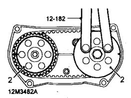
Using tool 12-182, rotate inlet camshaft rear timing gear until timing marks on both rear gears are facing outwards.
