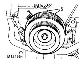
5. Check that timing mark on crankshaft pulley is aligned with mark on timing belt lower cover.
