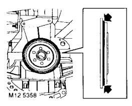
**33.** Apply a 1.5 mm continuous bead of sealant, Part No. GAC 8000 to replacement oil seal as shown.
