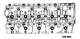
8. Tighten cylinder head bolts progressively in sequence shown to 20 Nm.
