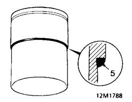
5. Apply a 2.0 mm thick continuous bead of sealant from kit, Part Number GGC 102 around shoulder of cylinder liner.
