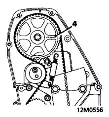
Rotate crankshaft clockwise to align carnshaft gear timing marks with top face of cylinder head - 90° BTDC. CAUTION: Do not use camshaft gear, gear retaining bolt or timing belt to rotate crankshaft.
