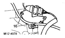
16. Remove 2 bolts securing multiplug bracket to camshaft carrier, remove bracket.
