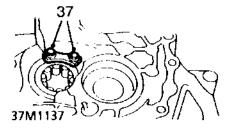
Remove and discard 2 Patchlok bolts securing output shaft bearing retaining plate - if fitted; remove plate.
