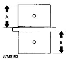
7. If clearance of either gear exceeds service limit measure length of appropriate side of spacer collar A or B. Length A = 4th gear side
