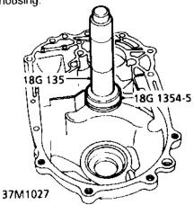
4. Fit a new output shaft bearing in differential housing using tools 18G 1354 and 18G 1354-5.
