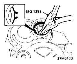
6. Using tool 18G 1392, release circlip retaining output shaft bearing.
