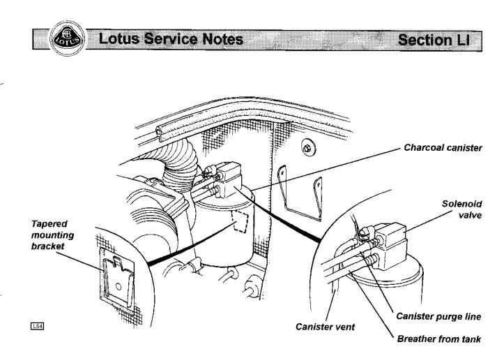
Fuel vapour from the top of the fuel tank filler neck is routed via a roll-over valve (to prevent fuel spillage if the car is inverted) mounted on a bracket integral with the filler neck, to the canister port labelled 'tank'. A central tube in the canister connects this port to the underside of the charcoal bed, below which is a reservoir to collect any liquid fuel.
