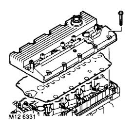
NOTE: Camshaft cover fitted to early engines illustrated.
