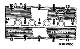
3. Fit camshaft cover on to camshaft carrier, fit 13 bolts at positions 1 and 4 to 15. Fit pillar bolts at positions 2 and 3. Tighten all bolts, in sequence shown, to 10 Nm.
