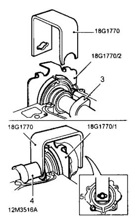
2. Rotate front and rear VVC control sleeves until timing plates 18G 1770/1 - front and 18G 1770/2 - rear can be inserted through the housing and into the control sleeve slot.
