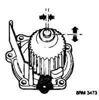
1. Check for movement of pump spindle in bearing and for coolant leakage from seal.
