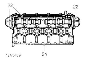
CAUTION: During the following operations, it is essential to ensure that front and rear inlet camshafts are retained in their respective VVC assemblies. If camshafts are removed from their VVC assemblies, then complete assembly must be replaced; it is not permissible to refit camshafts to VVC assemblies.
