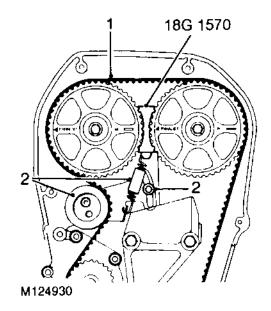
1. Remove and discard camshaft timing belt.
