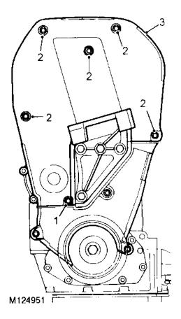
1. Stacken but do not remove bolt securing bottom of timing belt upper front cover.
