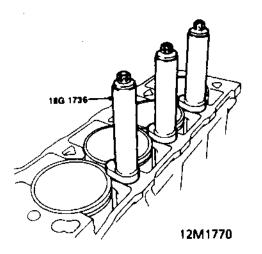
33. Assemble cylinder liner retainer clamps 18G 1736 to cylinder head botts. Position retainer clamps on cylinder liners ensuring clamps do not protrude over liner bores. Screw cylinder head botts into oil rail and tighten sufficiently to retain clamps.
