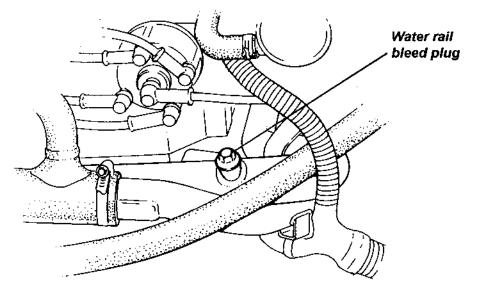
Using radiator pressure test equipment, pressurise the header tank to circulate the coolant. When neces-3. sary, refill the header tank and repeat. When a steady stream of coolant flows from the bleed port, replace the screw and washer and tighten.
