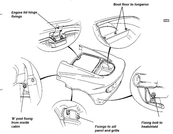
4. From inside the cabin, remove the full width trim panel from the rear bulkhead. From the access thus provided, remove the fixing securing the front end of the clamshell to the 'B' post above the engine bay air intake.
