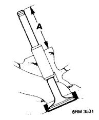
5. Check valve stem fitted height A:
