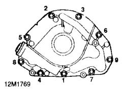
Fit oil pump, fit new Patchlok bolts, M6 x 20 bolt at position 3. Tighten in sequence shown to 10 Nm.
