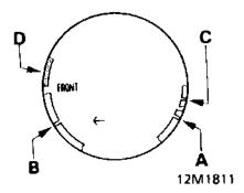
3. Ensure rings are free to rotate, position compression ring gaps A and B at 120° to each other and away from thrust side - left hand side of piston when viewed from front. Position oil control ring gap C and spring gap D at 30° on opposite side of gudgeon pin axis.
