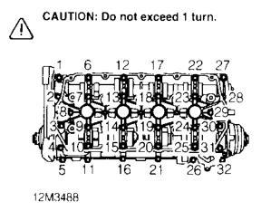
21. Using sequence shown, progressively slacken and noting the position of 4 longest bolts, remove 32 bolts securing camshaft carrier to cylinder head.
