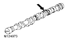
CAUTION: In order to commonise exhaust camshafts between VVC and non VVC engines, modified exhaust camshafts incorporating a reluctor ring are fitted to later engines, these camshafts are not interchangeable with those fitted to early engines. Commencing engine numbers for the modified camshafts are listed in Information.
