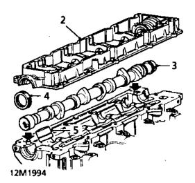
2. Remove camshaft carrier.
