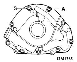
3. Noting fitted position of M6 x 20 bolt 'A,' remove and discard 9 bolts securing oil pump to cylinder block.
