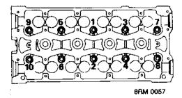
Tighten cylinder head bolts progressively in sequence shown to 20 Nm.
