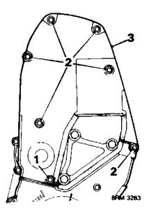
1. Slacken bottom bolt securing timing belt upper front cover.
