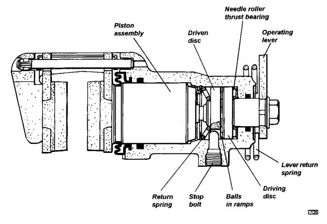
For the auto adjustment system to function correctly, it is essential that each caliper parking brake lever is allowed to return fully when the brake is released, and is not prevented from doing so by maladjustment of the parking brake cable. To check that the caliper levers are fully returned; with the parking brake 'off', measure the distance between the cable abutment and caliper lever as shown.
