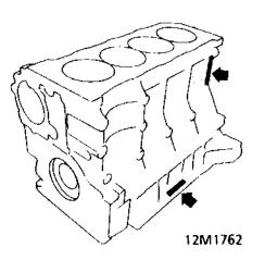
The engine number will be found stamped either on the LH side of the bearing ladder or cast on the rear LH side of the cylinder block.
