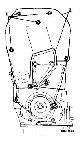
1. Slacken bottom bolt and remove 5 screws securing timing belt upper front cover.
