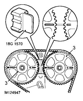
NOTE: VVC camshaft timing gear marks are shown in the inset on the illustration.
