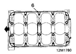
Apply a continuous bead of sealant, Part Number GUG 705963GM to paths shown on cylinder block then spread to an even film using a roller.
