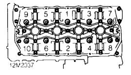
Tighten cylinder head bolts progressively in sequence shown to 20 Nm. Use a felt tip pen and mark position of radial mark on each bolt head. Tighten bolts in sequence shown through 180°
