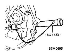
4. Inner bush: Using tool 18G 1723-1, drift inner bush into differential housing.
