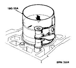
Fit ring clamp 18G 55A to each piston in tum and with 'FRONT' mark on piston to engine front, push piston into bore until flush with top face of cylinder liner. Remove ring clamp.
