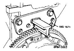
4. Fit flywheel locking tool 18G 1571, secure with 2 bolts.
