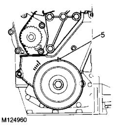
5. Check that timing mark on crankshaft pulley is aligned with mark on timing belt lower cover.
