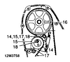
14. Slacken tensioner backplate screw and tension timing belt by applying finger pressure to tensioner backplate.
