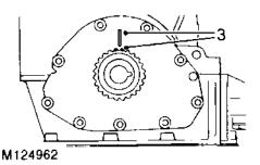
3. Check that crankshaft gear timing marks are aligned with flange on oil pump - 90° BTDC.
