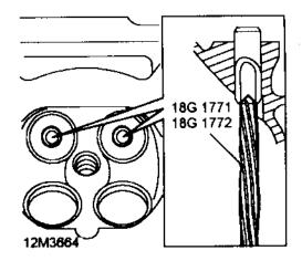
Remove carbon deposits from exhaust valve guides using tool: K8 - 18G 1772 K16 - 18G 1771
