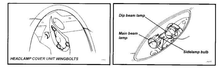
Headlamp bulbs may be replaced after disconnecting the cables (Dip; blue/yellow, black. Main; blue/ black, black) and releasing the spring clip. Both the 55W H1 dip beam bulb, and the 55W H7 main beam bulb incorporate orientation features which must be correctly located on re-fitting. The holder for the T4W bayonet fitting sidelamp bulb may be twisted to release from the main beam headlamp.
