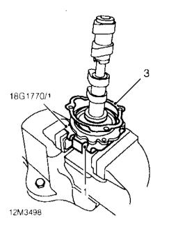
Secure VVC housing and camshaft in a soft-jawed vice with camshaft positioned upwards.
