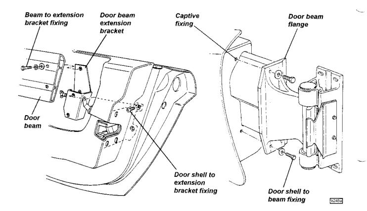
When refitting the door, take care not to scratch the glass if this is contained in the door. Insert the two rear bolts securing the beam to the latch bracket, but do not tighten until the three fixings securing the front of the shell to the beam flange have been fitted and tightened.
