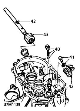
40. Remove detent cap bolt and washer, recover detent spring and ball.
