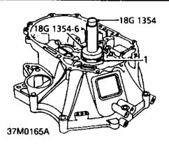
1. Fit a new input shaft bearing in differential housing using tools 18G 1354 and 18G 1354-6.
