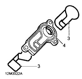
3. Using the fingers only, fit labyrinth seals each side of hydraulic control unit seal plate.
