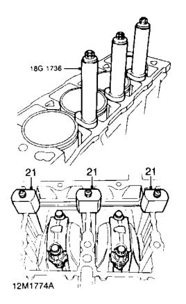
21. Fit cylinder liner retainer clamps 18G 1736 using nylon nuts supplied to retain the clamps. Ensure that feet of clamps do not protrude over cylinder bores. Tighten bolts sufficiently to retain clamps.
