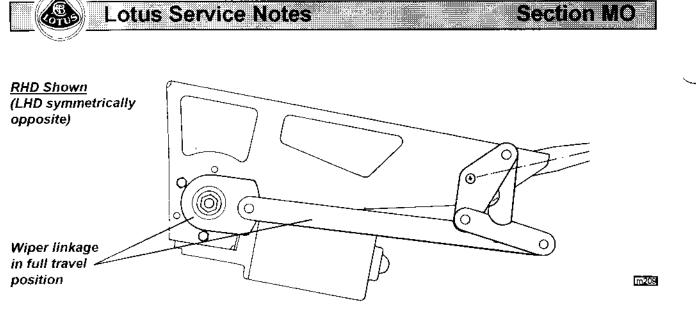
6. Re-assemble in the reverse order to removal, torque tightening the bracket bolts to 20 Nm.
