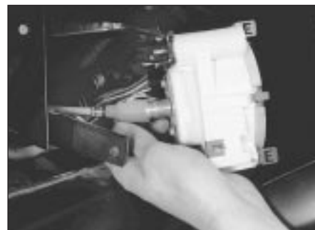
15.28a Detach the speedometer cable ...
