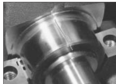
17.7 Plastigage in place on main bearing journal
