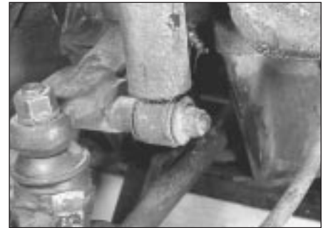
11.2b . . . and lower mounting
