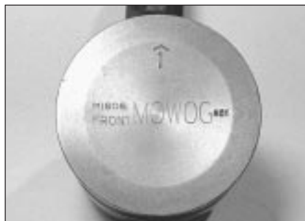
11.19 Identification markings on the piston crown
