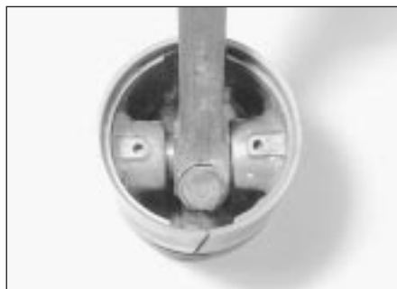
11.22 Gudgeon pin clamped in place by a pinch-bolt (848 cc)
