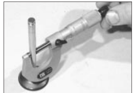
8.17 Measuring the valve stem diameter
