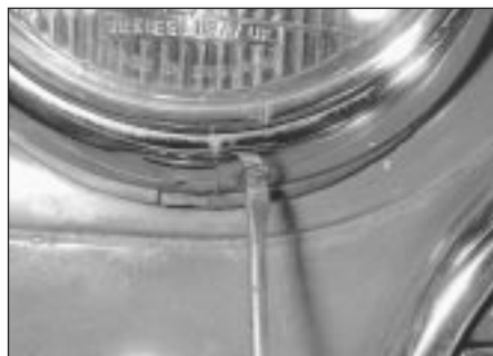
5.2b On non-Clubman models, undo the outer rim securing screw . . .
