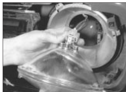
5.5 Detach the electrical connector and lift away the light unit
