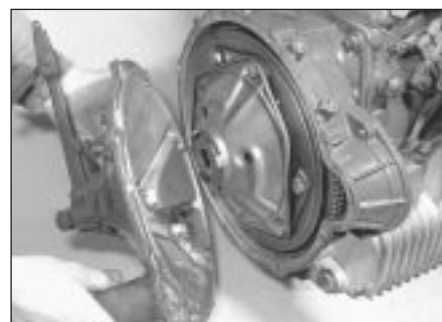
5.3 Removing the flywheel housing cover
