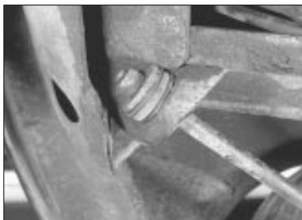
7.2 Tie-bar front mounting
