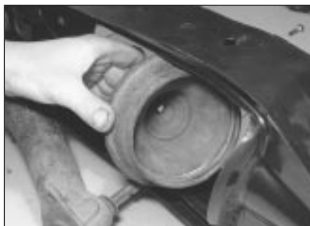
15.4 . . . and rubber cone spring
