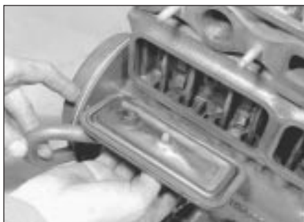
9.1 Removing the tappet side covers
