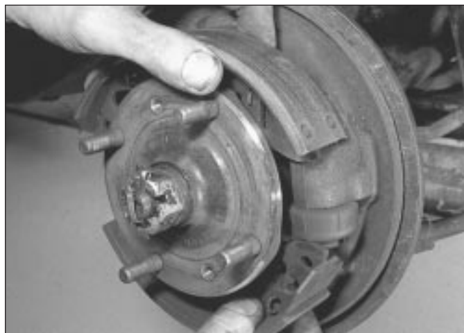
5.4b . . . and then from the piston end
