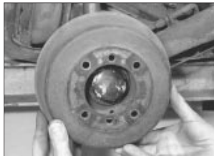
4.3 . . . and withdraw the drum
