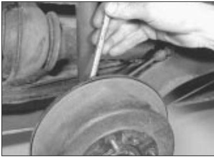
3.9 Adjusting the rear brakes
