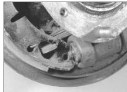
5.7c . . . and rear shoe from the handbrake lever and wheel cylinder
