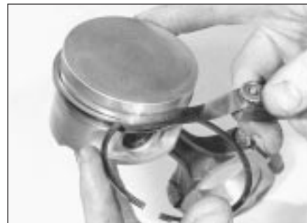
11.17 Measuring the piston ring-to-groove clearance
