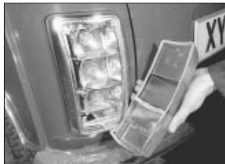
5.35a Rear light cluster lens removed for bulb renewal - Saloon models
