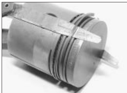
11.8 Using feeler blades to aid removal of the piston rings
