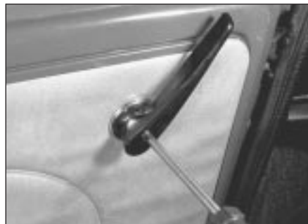
6.2a Remove the door lock remote control handle . . .
