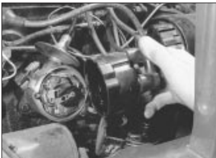
5.1 Removing the distributor cap
