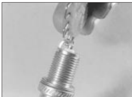
33.11 Adjusting a spark plug electrode gap
