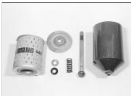
13.9 Components of the cartridge type oil filter
