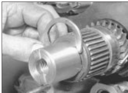
5.31b ... and the C-shaped washer
