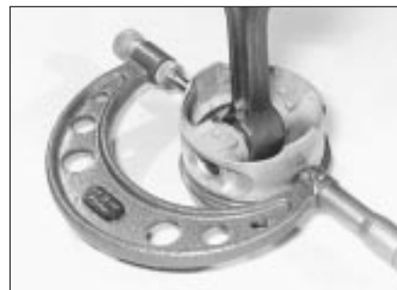
11.16 Measuring the piston diameter
