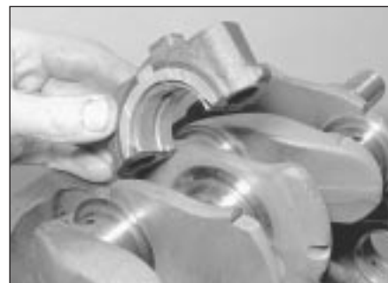
12.8 Main bearing cap with thrustwashers in position
