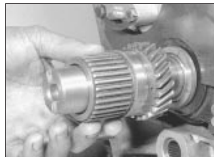
5.30 Slide on the primary gear ...
