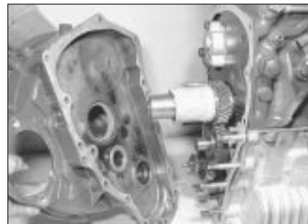
5.35 Refitting the flywheel housing
