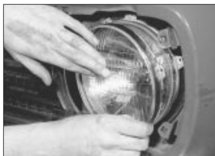
5.4b . . . and lift off the inner rim
