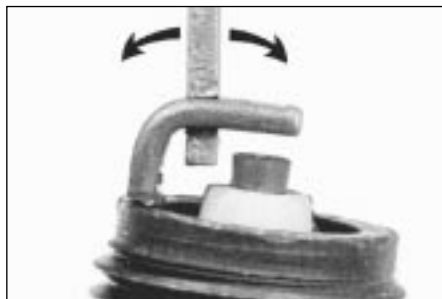
Adjusting spark plug gap
