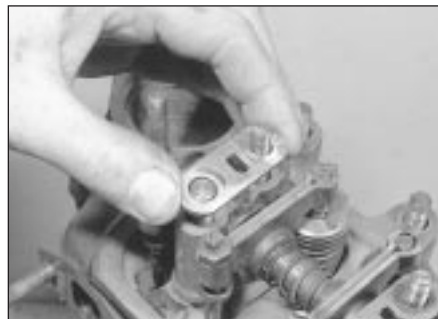
7.15a Recover the pedestal plate (where fitted) . . .
