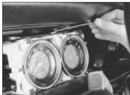
15.27b ... and upper retaining screws
