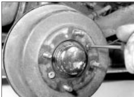
4.2c Remove the brake drum retaining screws . . .
