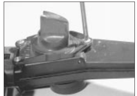
3.12 Removing the air cleaner intake duct adapter
