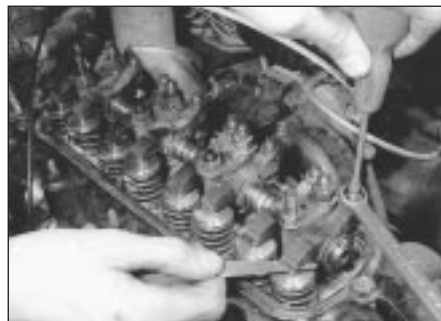
4.5 Adjusting the valve clearances
