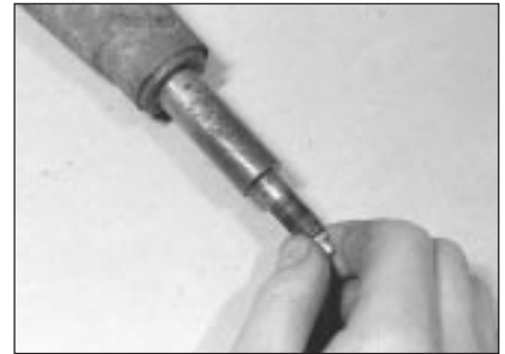
19.12c . . . then slide out the pivot shaft
