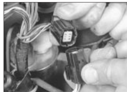
8.4 Disconnecting the exhaust system Lambda sensor wiring connector
