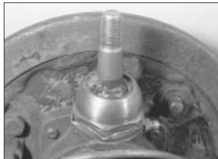
5.12d Bend up the lockwasher ...
