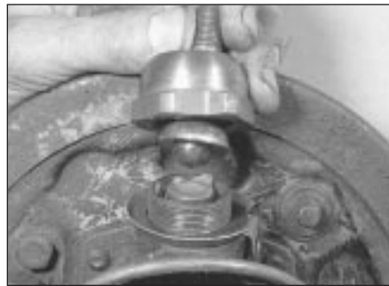
5.12a Refit the ball-pin and nut ...
