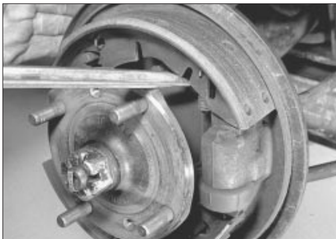
5.4a Remove the front brake shoes from the wheel cylinder pivot end first . . .
