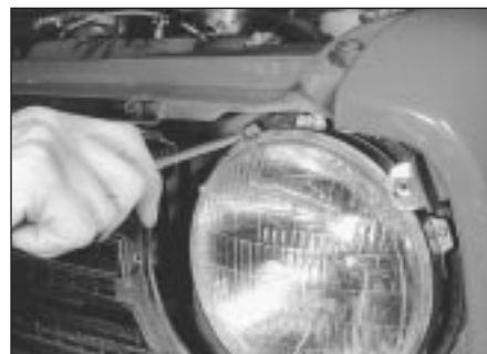
5.4a Unscrew the inner rim securing screws . . .
