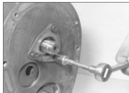
9.3 Undo the camshaft locating plate bolts and lift off the plate
