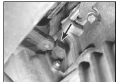
11.4 Crankshaft sensor location (arrowed) on manual transmission models - viewed from underneath
