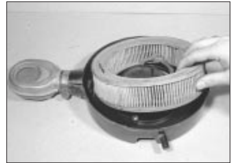
30.6b . . . and lift out the element
