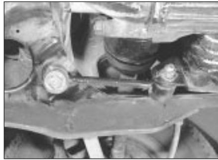
12.30 Lower engine tie-bar attachments
