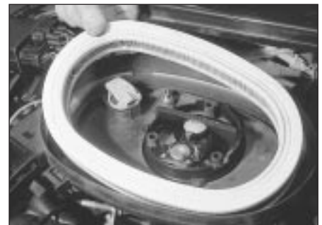
30.13b Lift off the lid and remove the element
