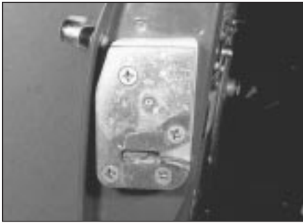
10.4 ... and the door lock retaining screws
