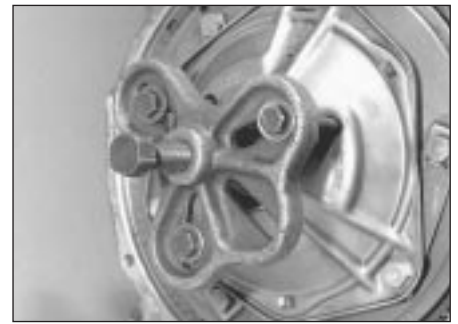
5.9 Using a commercially available puller to release the flywheel taper
