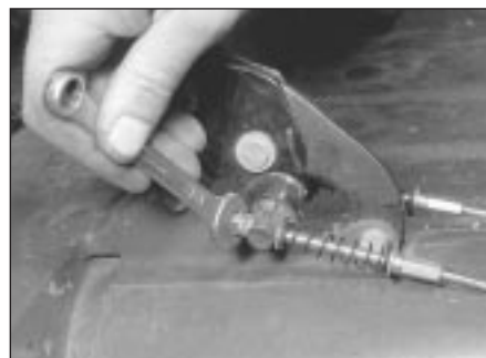
21.3 Remove the handbrake cable adjusting nuts
