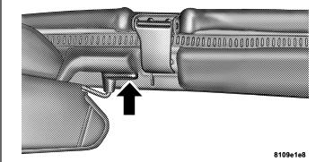
3. Remove the two Torx<sup>®</sup> head screws holding each side bar to the windshield frame. Shift the side bar inboard to clear windshield pillar molding when removing the side bar.
