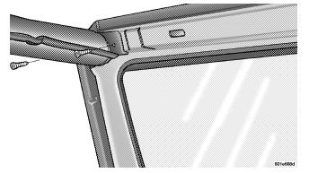
**NOTE:** Store all of the mounting bolts in their original threaded holes and tighten for safekeeping.
