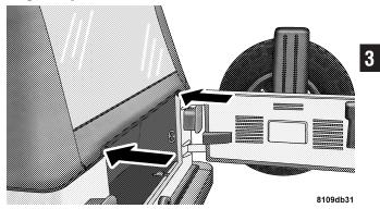
13. Tuck the lower retainers on the rear window under the tailgate clips.
