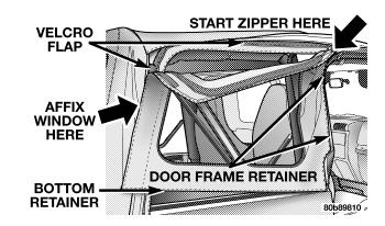
20. Tuck in the bottom retainers on the quarter windows into the bodyside retainer, beginning from the rear and working to the front of the vehicle. Repeat this step for the other side.
