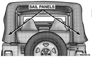
7. Tuck the sail panel retainer into the bodyside retainer. Begin working from the rear tailgate opening and work to the corner.
