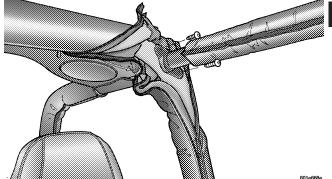
Do not loosen or remove the adjusting bolts on the side of the side bars. These bolts are set at the factory to properly fit the side bar to the vehicle.
