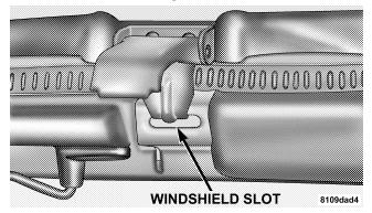
**NOTE:** Grasp the drip rail retainers on each side and untrap them from the door frame. Do not tuck the drip rails into the door frame at this time.
