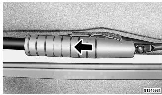
4. Grasp the header and lift the top back. Make sure the material is folded back as shown. Secure latches to plastic retainer on header.
