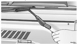
7. Remove the black round headed windshield Torx<sup>®</sup> head screw on each side of the base of the windshield.
