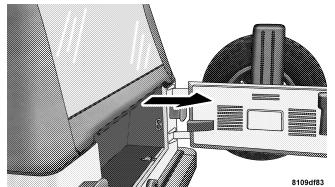
• Remove the rear window entirely. This is done by unzipping the window by bringing both the right zipper and left zipper tabs all the way to the end of the zipper track at the bottom left corner. Both zipper tabs will remain on the zipper track attached
