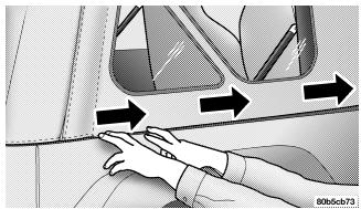
21. Locate the black retainer bar that was set aside, and the rear window. Remove and discard the end caps. Slide
