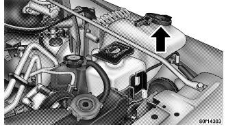
The fluid reservoir in the engine compartment should be checked for fluid level at regular intervals. Fill the reservoir with windshield antifreeze (not radiator antifreeze) rated not to freeze at  $-25^{\circ}$ F (-31°C). Operate the system for a few seconds to flush out the residual water.
