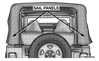
10. Completely release the hooks on the rear side of the windshield. Grasp the side bow behind the header and lift top back.
