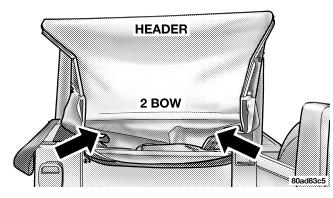
15. After the top is folded down, ensure that the drip rail retainers are tucked in inward as shown. This is to avoid unnecessary wear to the fabric.
