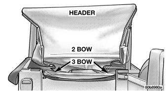
2. Move to the side of the vehicle and pull the side bow forward and down. Be sure the check straps are not tangled around the 2 bow. You will see the 3 bow rise from the rear of the vehicle.
