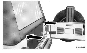
24. Tuck the lower retainers on both sides of the rear window under the tailgate clips. Reinstall the left sail panel if it was untucked to get the rear window zipper started.
