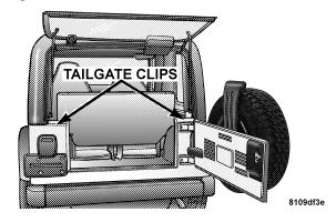
6. Pull the retainer bar straight out from the tailgate clips.
