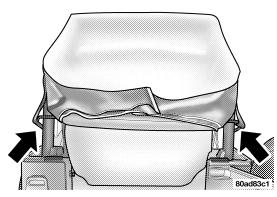
**NOTE:** If your vehicle is equipped with a Dual Top, prevent connector damage by ensuring that the hard top wire harness is folded back and secured to the main harness, using the attached Velcro<sup>®</sup> strap.
