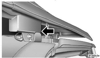
**NOTE:** Check to make certain the check straps are not tangled on any of the other top hardware. This will prevent the top from being put all the way up.
