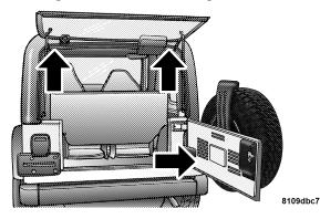
6. Locate the wiring harness at the rear left side corner of the vehicle.
