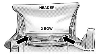
14. After the top is folded down, ensure that the drip rail retainers are tucked in inward as shown. This is to avoid unnecessary wear to the fabric.
