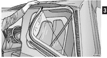
10. Tuck the bottom retainer on the quarter window into the bottom retainer, beginning from the rear and working to the front of the vehicle. Repeat this step for the other side.
