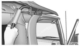
12. As you begin to lower the top, wrap the sail panels so that they rest on the roof of the vehicle.
