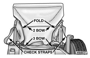
13. Tuck the top material between the 2 bow and the header.
