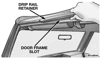
**NOTE:** Do not tuck the drip rails into the door frame at this time.
