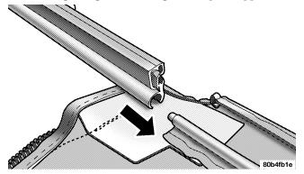
22. Zip the rear window beginning from the left using both zipper ends. Run the upper zipper around the window to the right side leaving the lower zipper end at the start on the left.
