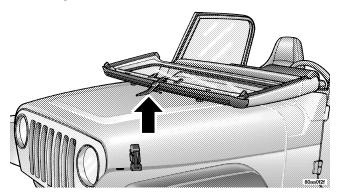
**Raising The Windshield And Replacing Side Bars** To raise the windshield, install the windshield wipers, and install the side bars use these same steps in reverse.
