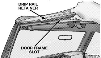
**NOTE:** Do not tuck the drip rail retainers into the frame at this time.
