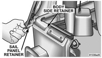
**NOTE:** This may be difficult due to fabric tension. If difficulty is experienced with fabric tension, place your hand on top of the 3 bow and gently pull down to help tuck in the sail panels.
