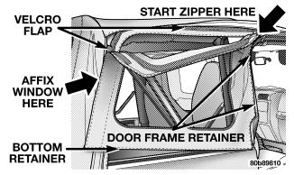
9. After the door frame retainer has been completely tucked in, finish zipping in the window. Then affix the Velcro<sup>®</sup> flaps around the window.
