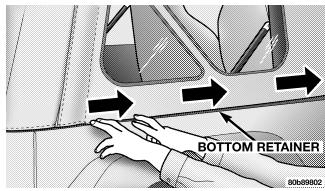
11. Zip in the rear window beginning from the left using both zipper ends. Run the upper zipper around the window leaving the lower zipper in at the start.
