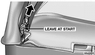
23. Tuck in the retainer bar ends into the tailgate clips on each side of the tailgate opening.
