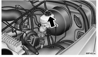
Be sure to clean the top of the master cylinder area before **7** removing the cap. If necessary, add fluid to bring the fluid level up to the requirements described on the brake fluid reservoir. With disc brakes, fluid level can be expected to fall as the brake pads wear. Brake fluid level
