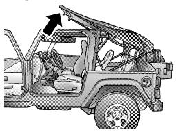
11. As you begin to lower the top, wrap the sail panels so that they rest on the roof of the vehicle.
