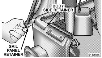
8. To install the quarter window, affix the rear corner of the window temporarily to the Velcro<sup>®</sup>. Start and zip the zipper only about 1 inch (2.5 cm). At this time it is necessary to tuck in the door frame retainer.
