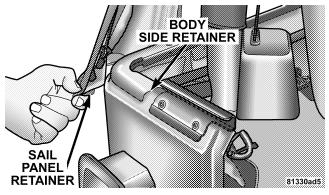
**NOTE:** This may be difficult due to fabric tension. If difficulty is experienced with fabric tension, place your hand on top of the 3 bow and pull down to help tuck in the sail panels.
