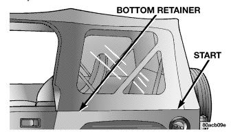
8. Finish unzipping the window and untuck from the door frame retainer at the front of the window, repeat this step on the other side.
