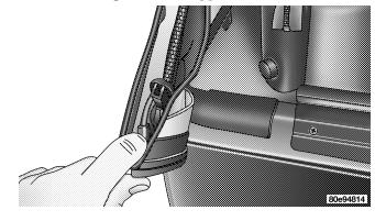
**NOTE:** To assist in getting the zipper started, lay the bar inside the vehicle on the right wheel well, uninstall half of the left sail panel from the bodyside retainer, beginning near the tailgate open to expose zipper ends.
