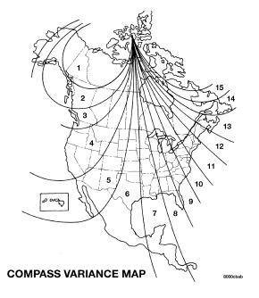
To set the variance: Turn the ignition ON, and press and hold the center button for 3 to 6 seconds. The last variance zone number will be displayed. Each press of the center button will select a new variance zone. When the proper zone is selected, wait 5 seconds to resume normal operation.
