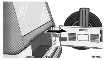
6. Remove the rear window entirely. This is done by unzipping the window, bringing both the right zipper and the left zipper tabs all the way to the end of the zipper track at the bottom left corner. Both zipper tabs
