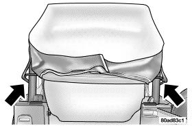
**NOTE:** If your vehicle is equipped with a Dual Top, prevent connector damage by ensuring that the hard top wire harness is folded back and secured to the main harness, using the attached Velcro<sup>®</sup> strap.
