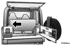
7. Disconnect the washer hose and install the tethered cap.
