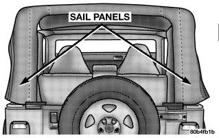
7. Align the sail panel retainer to the edge of the bodyside retainer at the rear. Tuck the sail panel into the bodyside retainer beginning from the rear and working to the corner. Tuck the retainer around the corner and continue forward. **NOTE:** This may be difficult due to fabric tension. If difficulty is experienced with fabric tension, place your hand on top of the 3 bow and gently pull down to help tuck in the sail panel retainers.
