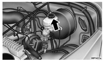
Be sure to clean the top of the master cylinder area before removing the cap. If necessary, add fluid to bring the fluid level up to the requirements described on the brake fluid reservoir. With disc brakes, fluid level can be expected to fall as the brake pads wear. Brake fluid level
