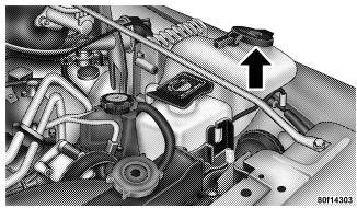
The fluid reservoir in the engine compartment should be checked for fluid level at regular intervals. Fill the reservoir with windshield antifreeze (not radiator antifreeze) rated not to freeze at -25°F (-31°C). Operate the system for a few seconds to flush out the residual water.
