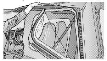
10. Tuck the bottom retainer on the quarter window into the bottom retainer, beginning from the rear and working to the front of the vehicle. Repeat this step for the other side. 11. Zip in the rear window beginning from the left using both zipper ends. Run the upper zipper around the window leaving the lower zipper in at the start.
