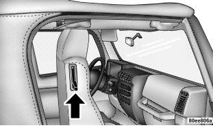
Front Seat Tilt Lever Fold And Tumble Rear Seat To expand the cargo area:
