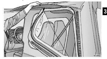
10. Tuck the bottom retainer of the quarter window into the bottom retainer, beginning from the rear and working to the front of the vehicle. Repeat this step for the other side. 11. To assist in getting the zipper started, lay the retainer bar inside the vehicle on the wheel wells and uninstall half of the left sail panel from the bodyside retainer beginning at the tailgate to expose zipper ends.
