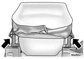
13. Make sure the sides of the top are folded inward as the top continues to fold, and check straps are clear of the vehicle.
