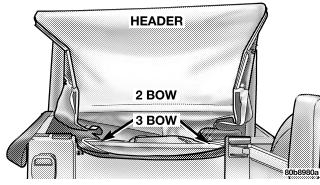
4. Engage the hooks on each side of the header into the windshield slots and fully engage the header latches.
