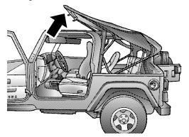
11. As you begin to lower the top, wrap the sail panels so that they rest on the roof of the vehicle.
