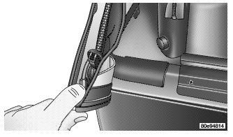
12. Zip in the rear window beginning from the left using both zipper ends. Run the upper zipper around the window leaving the lower zipper at the start.
