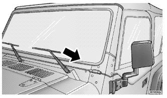
**Vehicle Identification Number NOTE:** It is illegal to remove the VIN plate.
