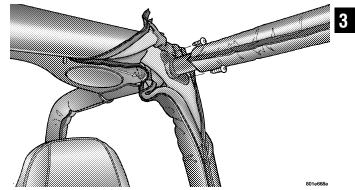
Do not loosen or remove the adjusting bolts on the side of the side bars. These bolts are set at the factory to properly fit the side bar to the vehicle.
