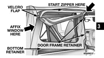
20. Tuck in the bottom retainers on the quarter windows into the bodyside retainer, beginning from the rear and working to the front of the vehicle. Repeat this step for the other side.
