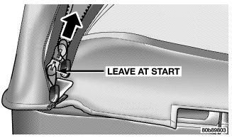
23. Tuck in the retainer bar ends into the tailgate clips on each side of the tailgate opening.
