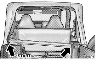
13. Tuck the retainer bar into the tailgate clips.
