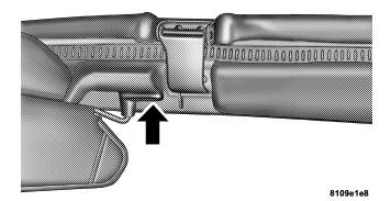
3. Remove the two Torx<sup>®</sup> head screws holding each side bar to the windshield frame. Shift the side bar inboard to clear windshield pillar molding when removing the side bar.
