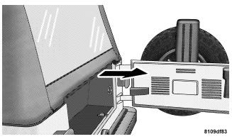
• Remove the rear window entirely. This is done by unzipping the window by bringing both the right zipper and left zipper tabs all the way to the end of the zipper track at the bottom left corner. Both zipper tabs will remain on the zipper track attached to the top. Pull up on the window to disengage zipper end. Stow the windows carefully to avoid scratching.
