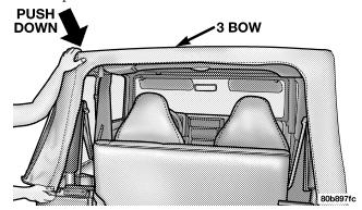
8. To install the quarter windows, affix the upper rear corner of the window temporarily using the Velcro<sup>®</sup>. Next, start the zipper about 1 inch (2.5 cm) at the upper forward corner of the window. At this time it is necessary to tuck in the door frame retainer.
