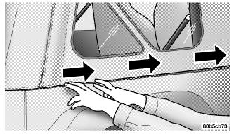
21. Locate the black retainer bar that was set aside, and the rear window. Remove and discard the end caps. Slide the retainer bar over the receiver at the bottom inside of the rear window with the bulky seal away from you. **NOTE:** To assist in getting the rear window zippers started, lay the bar inside the vehicle on the wheel wells and uninstall half of the left sail panel from the bodyside retainer, beginning near the tailgate to expose zipper ends.
