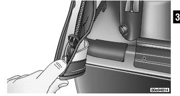
**NOTE:** To assist in getting the zipper started, lay the bar inside the vehicle on the right wheel well, uninstall half of the left sail panel from the bodyside retainer, beginning near the tailgate open to expose zipper ends.
