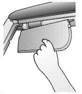
4. Open the header latches and engage the hook on each side into the windshield slot.
