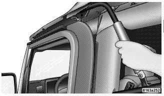
12. As you begin to lower the top, wrap the sail panels so that they rest on the roof of the vehicle.
