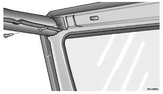
**NOTE:** Store all of the mounting bolts in their original threaded holes and tighten for safekeeping.
