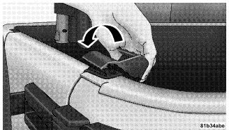
7. Move to the rear of the vehicle and gently pull the sail panels over the rear roof bow.
