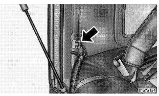
9. Remove the hard top from the vehicle. Place on a soft surface to prevent damage.
