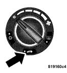
Press this button to choose between outside air intake or recirculation of the air inside the vehicle. A lamp will illuminate when you are in "Recirculate" mode. Only use the "Recirculate" mode to temporarily block out any outside odors, smoke, or dust and to cool the interior rapidly upon
