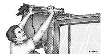
18. Gently slide the side bows off the door frame track and lower the top down into the vehicle.
