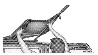
5. Fold back the front section of the top, and gently rest the header on top of the rear portion of the deck.
