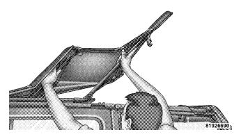
14. Fold back the front section of the top, and gently rest the header on top of the rear portion of the deck.
