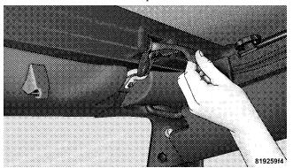
6. If the swing gate brackets were removed, install them by hooking the rear edge of the bracket on the interior
