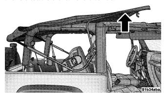
15. Tuck the fabric and the check straps between the bows and as far inward as possible. This will keep any portion of the top from flapping outside of the vehicle.
