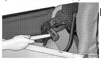
5. Unzip the zipper on the sport bar cover to expose the pivot brackets. Remove the brackets using a #T30 Torx® head driver. Recover and re-zip the sports bar cover. Store pivot brackets and screws in a safe place.
