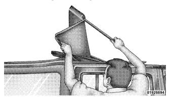
15. Fold the top material so that the plastic retainers form a "W" as shown. Enter the vehicle, and move the material into two folds.
