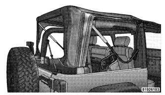
8. Partially install the sail panel retainers into the body side channel, leaving the last three (3) inches towards the
