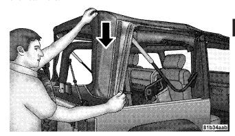
9. To install the side windows, affix the window temporarily by attaching to the Velcro® in the rear corner. Start the zipper but close only about 1 inch (2.5 cm).
