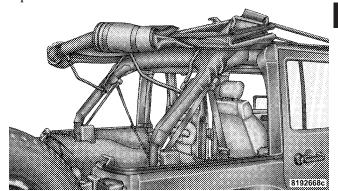
12. The swing gate brackets do not need to be removed unless the hard top is being installed. To remove the swing gate brackets, pull the front of the bracket forward while rolling the entire bracket back in towards the vehicle to disengage.
