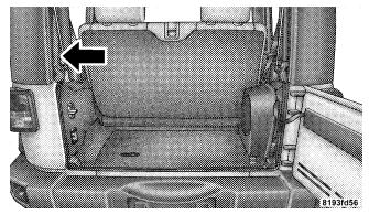
7. Disconnect the washer hose and install the tethered cap.
