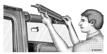
6. Loosely install both knobs beginning with the front knob (long knob). Then, install the middle knob (short knob) through the front and rear door frames and screw into the top of the b-pillar.
