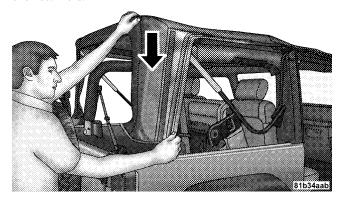
14. To install the side windows, affix the window temporarily by attaching to the Velcro® in the upper rear corner. Start the zipper but close only about 1 inch (2.5 cm).
