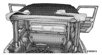
12. The swing gate brackets do not need to be removed unless the hard top is being installed. To remove the swing gate brackets, pull the front of the bracket forward while rolling the entire bracket back in towards the vehicle to disengage.
