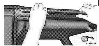
19. Close the header latches and return the sun visors to their secured position.
