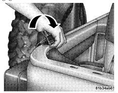
13. Completely release the latches from the loops on the windshield frame.
