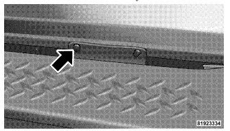
2. Remove one (1) bolt from underside of vehicle.
