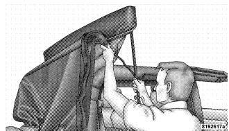
4. Before attaching the header latches, be sure that the top retainers above the door are not trapped between the top and the door frame.
