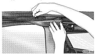
10. Insert the front retainer of the window into the door channel, making sure the retainer is fully seated and
