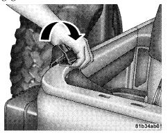
13. Grasp the front side bow behind the header, and lift the top.
