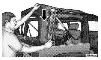
**NOTE:** When releasing the sail panel retainers, it is helpful to pull down on the rear roof bow.
