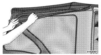
12. Insert the retainer along the bottom edge of the window into the bottom side channel, beginning at the
