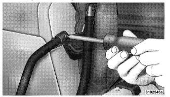
4. Using a rubber mallet, carefully tap the knuckles from the left and right metal pivot brackets. Remove the soft top from the vehicle and store in a clean, dry location.
