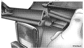
19. Install the rear window by starting both zipper ends at the lower left corner of the rear window opening. Ensure that the zippers are properly started and aligned before zipping to prevent damage.
