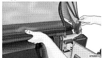
17. Apply downward pressure on the top corner of the rear soft top bow (3 bow), then complete attaching the sail panel retainers into the body side channel.
