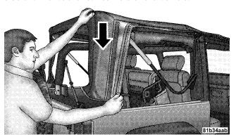
**NOTE:** When releasing the sail panel retainers, it is helpful to pull down on the rear roof bow.
