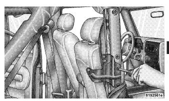
b. Lay the soft top into the rear of the vehicle with the bows pointing forward and the curved portion of the bows facing upward.
