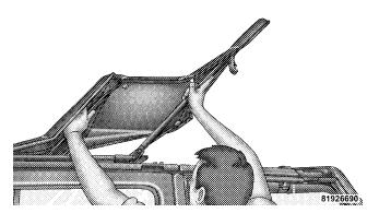
9. Before attaching the header latches, be sure the top retainers above the doors do not get trapped between the top and the door frame. Also, make certain the feet at both ends of the 2 bow (forward most bow) seat properly
