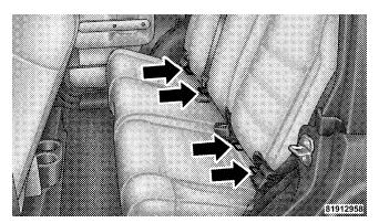
**Latch Anchorages (4 Door Models)** In addition, there are tether strap anchorages behind each rear seating position located on the back of the seat.
