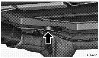
4. Turn rear fasteners (knobs) (located on overhead speaker bar assembly) counter-clockwise until they can be removed.
