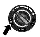
Press this button to engage the air conditioning. A lamp will illuminate when the air conditioning system is engaged
