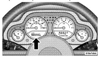
The compass/trip computer, when the appropriate conditions exist, will show the following messages in the odometer display:
