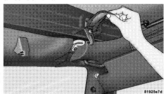
14. Grasp the side bow behind the header, lift the top, and fold toward the rear of the vehicle.
