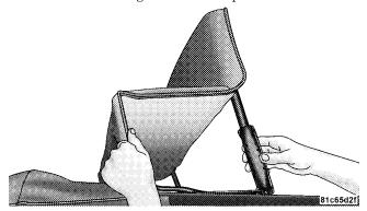
6. Locate straps to secure side bows. Wrap straps around bows as shown. Repeat on the other side.
