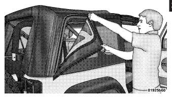
9. Once unzipped, remove side window retainers from the door channel and body side channel. Repeat this step on the opposite side.
