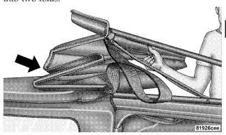
16. Release the side bows by pressing down on the latch above the front of the rear door. Push the top rearward to disengage. Repeat this step on the other side.
