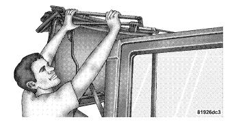
18. Before lowering the top, open the swing gate to prevent possible damage to the rear center high-mounted brake lamp. Gently slide the side bows off the door frame track and lower the top down into the vehicle.
