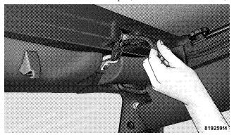
11. If the swing gate brackets were removed, install them by hooking the rear edge of the bracket on the interior side of the body channel. Then, rotate it rearward and
