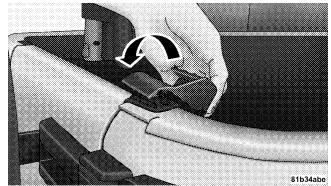
9. Move to the rear of the vehicle and gently pull the sail panels over the rear roof bow.
