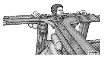
5. Place one hand on the upper rear and one hand on the upper front of the rear door frame. Pull the frame towards you with your rear hand to remove the frame from the vehicle.
