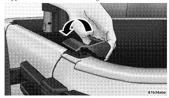
12. Move to the rear of the vehicle and gently pull the sail panels over the rear roof bow (4-bow).
