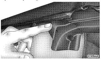
25. Close the header latches and return the sun visors to their secured position.
