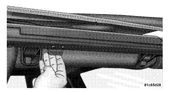
16. Before lowering the top, open the swing gate to prevent possible damage to the rear center high-mounted brake lamp. Move to the front of the vehicle. Grasp the side bow behind the header and lift the top, folding it toward the rear of the vehicle.
