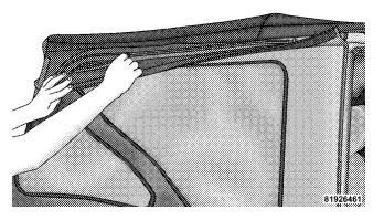
14. Insert the retainer along the bottom edge of the window into the bottom side channel, beginning at the front and working to the rear of the vehicle. Finish by closing the zipper completely and attaching the Velcro® along the top and rear of the window. Repeat this step for the opposite side.
