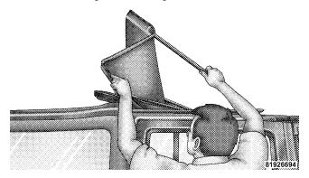
6. Fold the top material so that the plastic retainers form a "W" as shown. Enter the vehicle, and move the material into two folds. Ensure that the straps are securely stowed.
