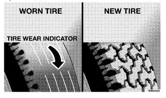
These indicators are molded into the bottom of the tread grooves and will appear as bands when the tread depth becomes 1/16 inch (2 mm). When the indicators appear in two or more adjacent grooves, the tire should be replaced.
