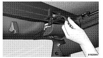
8. If the swing gate brackets were removed, install them by hooking the rear edge of the bracket on the interior side of the body channel. Then, rotate it rearward and over the channel until it snaps onto the exterior part of the rail. To be properly located, the bracket must only be clipped to the shortened rail edge.
