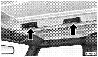
3. Turn rear L-shaped lock (located above shoulder belt anchorage).
