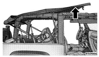
17. Tuck the fabric and the check straps between the bows and as far inward as possible. This will keep any
