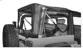
10. Partially install the sail panel retainers into the body side channel, leaving the last 3 in (7.6 cm) towards the rear window loose (on both sides). Pulling down on the rear roof bow (3–bow) will aid to reach the channel with the retainers.
