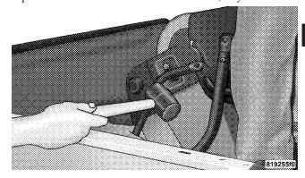
5. Unzip the zipper on the sport bar cover to expose the pivot brackets. Remove the brackets using a #T30 Torx® head driver. Recover and re-zip the sports bar cover. Store pivot brackets and screws in a safe place.
