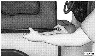
18. Locate the black swing gate bar. Slide the swing gate bar over the receiver at the bottom inside of the rear window. The spongy part of the seal should be down and pointed outward to seal with the swing gate when closed.
