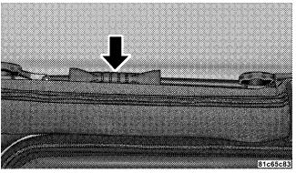
4. Standing on the side of the vehicle, lift the top by the side bow and the 2-bow (middle bow) up and over the sports bar until the header rests on the top of the windshield frame.
