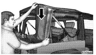
14. To install the side windows, affix the window temporarily by attaching to the Velcro® in the upper rear corner. Start the zipper but close only about 1 in (2.5 cm).
