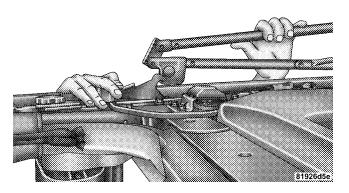
17. Grasp the folded side bows and slide the top along the door frame track to the rear door frame.
