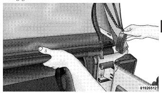
22. Complete the installation of the sail panel by inserting the rest of the retainer into the body channel.
