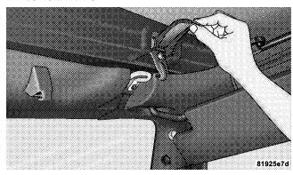
4. Grasp the front side bow behind the header, and lift the top.
