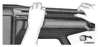
21. Close the header latches and return the sun visors to their secured position.
