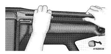
24. Ensure plastic retainer is tucked in properly at B-pillar, not pinching the seal.
