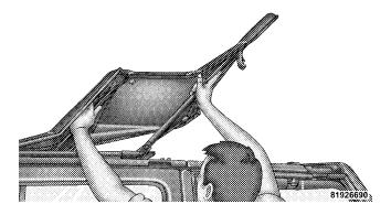
14. Fold back the front section of the top, and gently rest the header on top of the rear portion of the deck.
