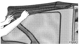
17. Insert the retainer along the bottom edge of the window into the bottom side channel, beginning at the front and working to the rear of the vehicle. Finish by closing the zipper completely and attaching the Velcro® along the top and rear of the window. Repeat this step for the opposite side.
