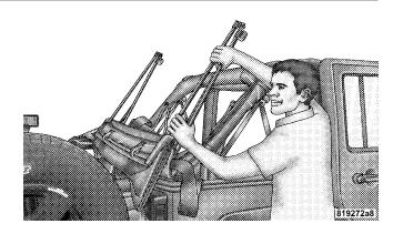
5. Insert the slider feature of the knuckles into the door frame tracks and slide the top forward.
