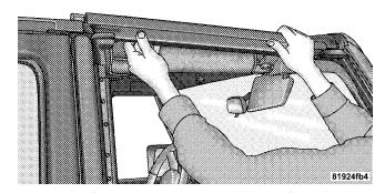
3. Pull the frame towards you with your front hand to remove the frame from the vehicle.
