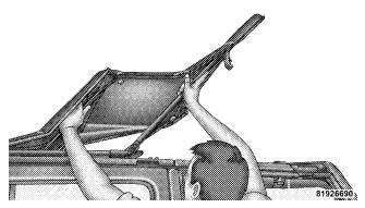
9. Before attaching the header latches, be sure the top retainers above the doors do not get trapped between the top and the door frame. Also, make certain the feet at both ends of the 2–bow (forward most bow) seat properly
