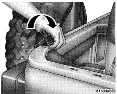
13. Grasp the front side bow behind the header, and lift the top.
