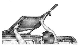
5. Fold back the front section of the top, and gently rest the header on top of the rear portion of the deck.
