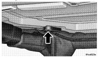
4. Turn rear fasteners (knobs) (located on overhead speaker bar assembly) counterclockwise until they can be removed.
