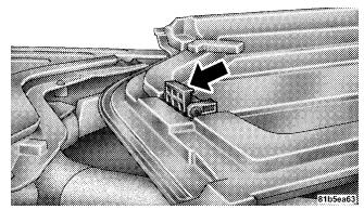
**NOTE:** The front panel(s) must be positioned properly to ensure sealing. Set the panels on the windshield frame so that there is no overhang. Also, make sure that the panels are sitting flush with the body.
