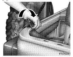
13. Completely release the latches from the loops on the windshield frame. If your vehicle is not equipped with the Sunrider package, proceed to Step 16.
