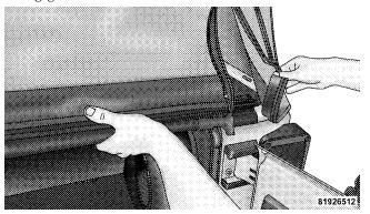
19. Apply downward pressure on the top corner of the rear soft top bow (3–bow), then complete attaching the sail panel retainers into the body side channel.
