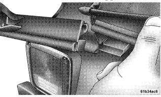
15. Install the rear window by starting both zipper ends at the lower left corner of the rear window opening. Ensure that the zippers are properly started and aligned before zipping to prevent damage.
