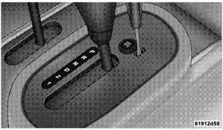
Brake/Transmission Interlock Manual Override
