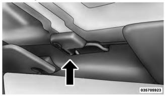
3. Turn the rear L-shaped lock (located above the shoulder belt anchorage).
