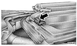
**NOTE:** The front panel(s) must be positioned properly to ensure sealing. Set the panels on the windshield frame so that there is no overhang. Also, make sure that the panels are sitting flush with the body.
