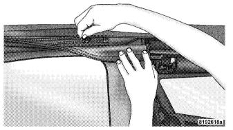
14. Insert the front retainer of the window into the door channel, making sure the retainer is fully seated and properly positioned on the door frame. Failure to do so can result in wind and water leaks or damage to the window.
