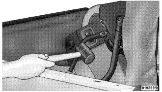
5. Unzip the zipper on the sport bar cover to expose the pivot brackets. Remove the brackets using a #T30 Torx<sup>®</sup> head driver. Recover and re-zip the sports bar cover. Store the pivot brackets and screws in a safe place.
