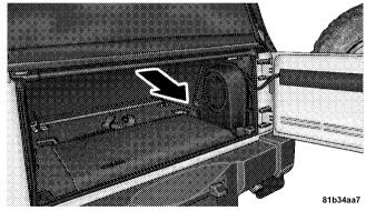
• Unzip the rear window starting at the right lower corner of the window. Pull the zipper up, across the top and down to the left lower corner. **Zipper pulls will stay on the rear window**. Pull down on the rear window to disengage it from the zipper on the top cover. Stow the windows carefully to avoid scratching.
