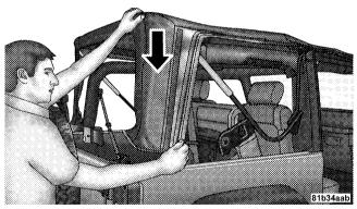
11. To install the side windows, affix the window temporarily by attaching to the Velcro<sup>®</sup> in the rear corner. Start the zipper but close only about 1 in (2.5 cm).
