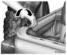
13. Completely release the latches from the loops on the windshield frame. If your vehicle is not equipped with the Sunrider<sup>®</sup> package, proceed to Step 16.
