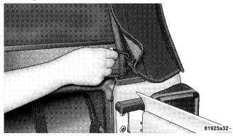
7. Undo the Velcro<sup>®</sup> that runs along the top and rear edge of the side window.
