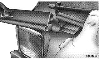
17. Install the rear window by starting both zipper ends at the lower left corner of the rear window opening. Ensure that the zippers are properly started and aligned before zipping to prevent damage.
