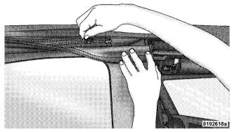
12. Insert the front retainer of the window into the door channel, making sure the retainer is fully seated and properly positioned on the door frame. Failure to do so can result in wind and water leaks or damage to the window.
