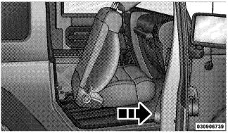
**Easy Entry Seat With Combination Lever** — If Equipped 1. To return the seat to a sitting position, rotate the seatback upright until it locks.
