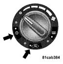
For maximum cooling, select either the Panel or Bi-Level position using the mode control. Then, press the "A/C" and the "Recirculation" buttons so that both lights are illuminated, and set the temperature control to its coolest setting.
