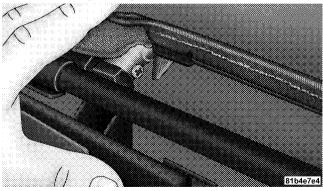
10. Open the header latches and engage the hook on each side onto the windshield loops (do not close the latches).
