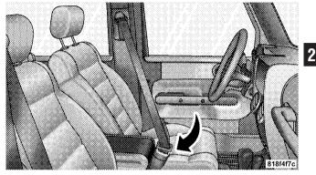
Inserting Latch Plate into Buckle
