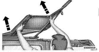
14. Fold back the front section of the top, pulling the fabric rearward. Gently rest the header on top of the rear portion of the deck.
