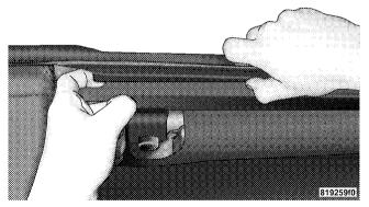
3. Release the header latches from the loops on the windshield frame.
