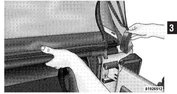
20. Complete the installation of the sail panel by inserting the rest of the retainer into the body channel.
