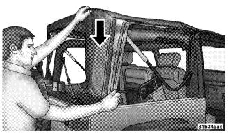
13. To install the side windows, affix the window temporarily by attaching it to the Velcro<sup>®</sup> in the upper rear corner. Start the zipper but close only about 1 in (2.5 cm).
