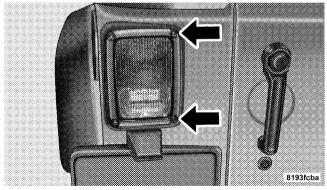
2. Separate the housing from the body by pushing the lamp inboard while pulling the lamp away from the body.
