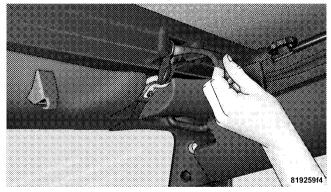
8. If the swing gate brackets were removed, install them by hooking the rear edge of the bracket on the interior side of the body channel. Then, rotate it rearward and over the channel until it snaps onto the exterior part of the rail. To be properly located, the bracket must only be clipped to the shortened rail edge.
