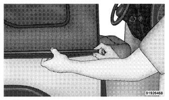
14. Locate the black swing gate bar. Slide the swing gate bar over the receiver at the bottom inside of the rear window. The spongy part of the seal should be down and pointed outward to seal with the swing gate when closed.
