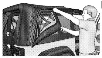
9. Once unzipped, remove the side window retainers from the door channel and body side channel. Repeat this step on the opposite side.
