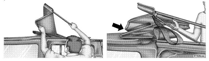
16. Release the side bows by pressing down on the latch above the front of the rear door. Push the top rearward to disengage. Repeat this step on the other side.
