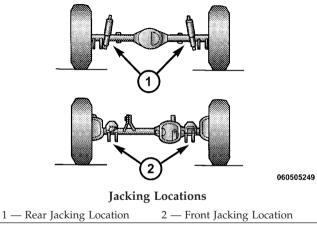
5. Raise the vehicle by turning the jack screw to the right. Raise the vehicle only until the tire just clears the surface and enough clearance is obtained to install the spare tire. Minimum tire lift provides maximum stability.
