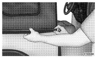
16. Locate the black swing gate bar. Slide the swing gate bar over the receiver at the bottom inside of the rear window. The spongy part of the seal should be down and pointed outward to seal with the swing gate when closed.
