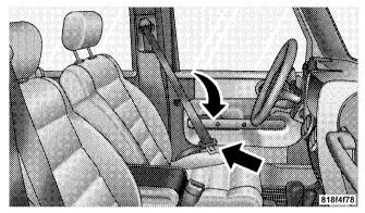
**Pulling Out the Lap/Shoulder Belt Latch Plate** 3. When the belt is long enough to fit, insert the latch plate into the buckle until you hear a "click."
