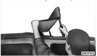
5. Locate the straps to secure the side bows. Wrap the straps around the bows as shown. Repeat on the other side.
