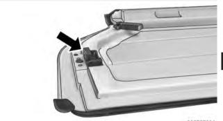
**NOTE:** The front panel(s) must be positioned properly to ensure sealing. Set the panels on the windshield frame so that there is no overhang. Also, make sure that the panels are sitting flush with the body.
