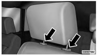
Removing Head Restraint
