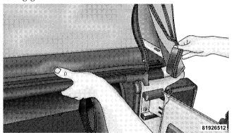
17. Apply downward pressure on the top corner of the rear soft top bow (3–bow), then complete attaching the sail panel retainers into the body side channel.
