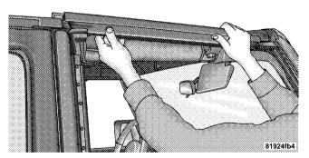
3. Pull the frame toward you with your front hand to remove the frame from the vehicle.
