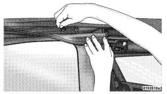
13. Insert the front retainer of the window into the door channel, making sure the retainer is fully seated and properly positioned on the door frame. Failure to do so can result in wind and water leaks or damage to the window.
