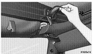
3. Grasp the front side bow behind the header, and lift the top.
