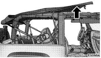
16. Tuck the fabric and the check straps between the bows and as far inward as possible. This will keep any portion of the top from flapping outside of the vehicle.
