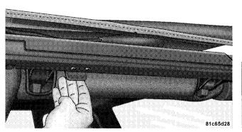
15. Before lowering the top, open the swing gate to prevent possible damage to the rear center high-mounted brake light. Move to the front of the vehicle. Grasp the side bow behind the header and lift the top, folding it toward the rear of the vehicle.
