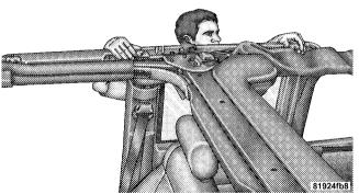
5. Place one hand on the upper rear and one hand on the upper front of the rear door frame. Pull the frame toward you with your rear hand to remove the frame from the vehicle.
