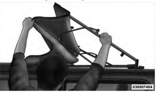
5. Fold the top so that the material forms a "W" as shown. Enter the vehicle and move the material into two folds.
