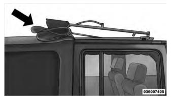
6. Secure the top by using the two provided straps. Each strap will wrap around the side bow and Velcro® to itself; use one strap on each side of the vehicle.
