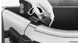
11. Ensure that the straps are positioned correctly before pulling the sail panels over the rear roof bow (4–bow).
