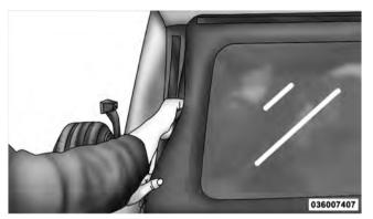
15. Locate the black swing gate bar. Slide the swing gate bar over the receiver at the bottom inside of the rear window. The spongy part of the seal should be down and pointed outward to seal with the swing gate when closed.
