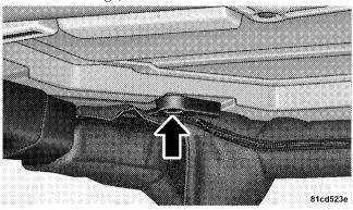
5. Unlatch the header panel latch located at the top of the windshield.
