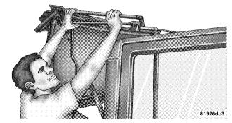
17. Gently slide the side bows off the door frame track and lower the top down into the vehicle.
