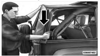
3. Rotate the header forward.
