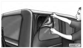
2. Release header latches from the windshield frame.
