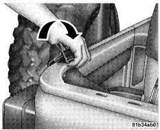
12. Grasp the front side bow behind the header, and lift the top.
