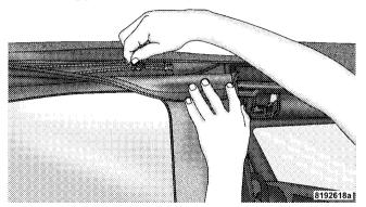
11. Insert the front retainer of the window into the door channel, making sure the retainer is fully seated and properly positioned on the door frame. Failure to do so can result in wind and water leaks or damage to the window.
