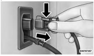
**NOTE:** If necessary, pliers can be used to lightly squeeze grips while disconnecting the washer hose.
