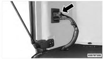
6. Locate the wire harness on the left rear inside corner of 7. Release the red locking tab by pushing upward.
