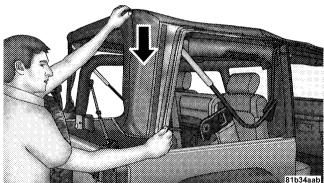
10. To install the side windows, affix the window temporarily by attaching to the Velcro® in the rear corner. Start the zipper but close only about 1 in (2.5 cm).
