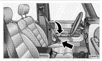
Pulling Out the Lap/Shoulder Belt Latch Plate
