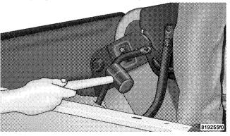
5. Unzip the zipper on the sport bar cover to expose the pivot brackets. Remove the brackets using a #T30 Torx® head driver. Recover and re-zip the sports bar cover. Store the pivot brackets and screws in a safe place.
