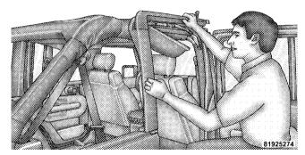
3. Position the top of the door frame against the metal sport bar and press onto the side bar making sure not to
