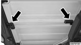
4. Turn the rear L-shaped lock (located above the shoulder belt anchorage).
