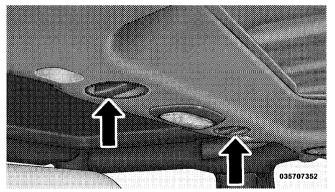
3. Turn the center L-shaped locks (two) from the center of the roof panel.
