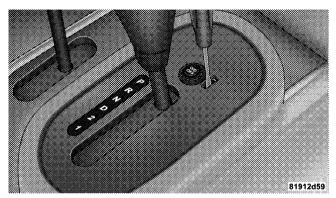
**Brake/Transmission Interlock Manual Override**6. Press the shifter release button and shift into NEU-TRAL.
