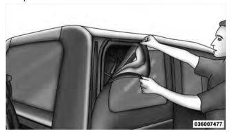
8. Once unzipped, remove the side window retainers from the door channel and body side channel. Repeat this step on the opposite side.
