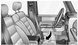
Inserting Latch Plate into Buckle
