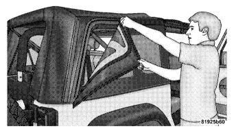
8. Once unzipped, remove the side window retainers from the door channel and body side channel. Repeat this step on the opposite side.
