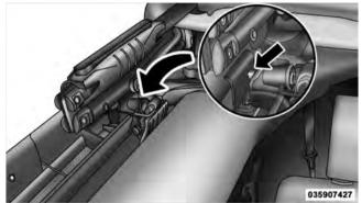
6. Open the header latches and engage the hook on each side onto the windshield loops (do not close the latches).
