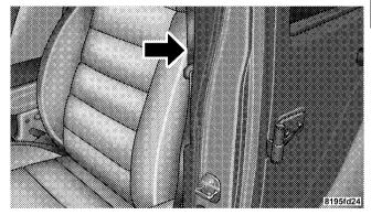
Supplemental Seat-Mounted Side Airbag Location **NOTE:** Airbag covers may not be obvious in the interior trim; but they will open during airbag deployment.
