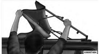
14. Fold the top so that the material forms a "W" as shown. Enter the vehicle and move the material into two folds.
