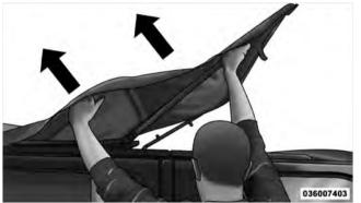
13. Fold back the front section of the top, pulling the fabric rearward. Gently rest the header on top of the rear portion of the deck.
