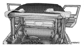
11. The swing gate brackets do not need to be removed unless the hard top is being installed. To remove the swing gate brackets, pull the front of the bracket forward while rolling the entire bracket back in toward the vehicle to disengage.
