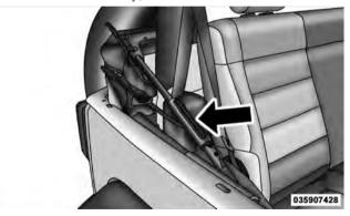
4. Standing on the side of the vehicle, lift the top by the side bow and the 2–bow (middle bow) up and over the sports bar until the header rests on the top of the windshield frame.
