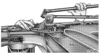
16. Before lowering the top, open the swing gate to prevent possible damage to the rear center high-mounted brake light. Grasp the folded side bows and slide the top along the door frame track to the rear door frame.
