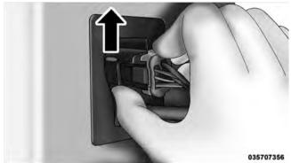
8. To remove the wiring harness press the side tab and pull to disconnect.
