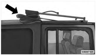
6. Secure the top by using the two provided straps. Each strap will wrap around the side bow and Velcro<sup>®</sup> to itself; use one strap on each side of the vehicle.
