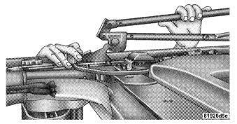
18. Before lowering the top, open the swing gate to prevent possible damage to the rear center high-mounted brake light. Grasp the folded side bows and slide the top along the door frame track to the rear door frame.
