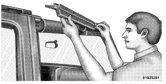
6. Clip the front of the door rail over the side bar making sure that the material for the side bar cover is not pinched by the door frame.
