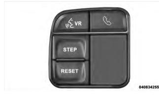
**Compass/Temperature Control Buttons** Press and release the STEP button on the steering wheel to access the options in the Compass display. **NOTE:** The system will display the last known outside temperature when starting the vehicle and may need to be driven several minutes before the updated temperature is displayed. Engine temperature can also affect the displayed temperature; therefore, temperature readings are not updated when the vehicle is not moving.
