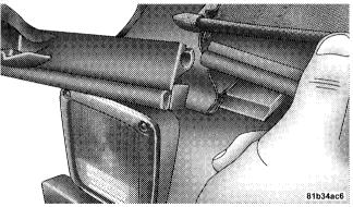
14. Install the rear window by starting both zipper ends at the lower left corner of the rear window opening. Ensure that the zippers are properly started and aligned before zipping to prevent damage.
