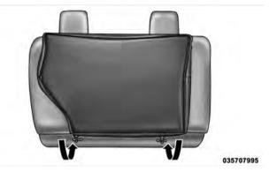
Wrap the upper strap around the rear head restraints and loop the strap through the buckle. Pull on the strap to tighten the Freedom bag securely against the rear seat.
