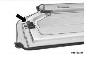
**NOTE:** The front panel(s) must be positioned properly to ensure sealing. Set the panels on the windshield frame so that there is no overhang. Also, make sure that the panels are sitting flush with the body.
