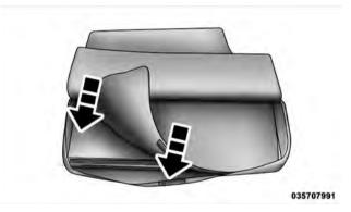
Insert the left-side Freedom panel into the bag with the Ulatches facing upward.
