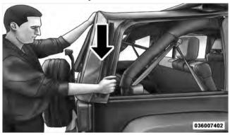
3. Rotate the header forward.
