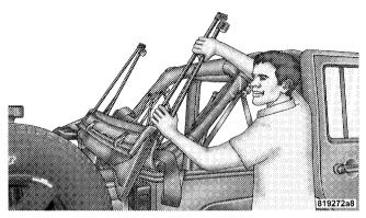
20. Tuck the fabric and the check straps between the bows as far inside as possible. This will keep any portion of the top from flapping outside of the vehicle.
