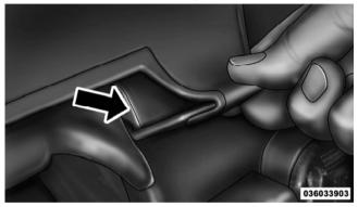
18. Apply downward pressure on the top corner of the rear soft top bow (3–bow), then complete attaching the sail panel retainers into the body side channel.
