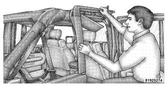
3. Position the top of the door frame against the metal sport bar and press onto the side bar making sure not to pinch the material of the sports bar covers and to ensure it is properly positioned on the seal above the front of the rear door.
