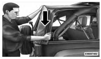
12. To install the side windows, affix the window temporarily by attaching it to the Velcro<sup>®</sup> in the upper rear corner. Start the zipper but close only about 1 in (2.5 cm).
