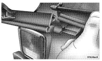
16. Install the rear window by starting both zipper ends at the lower left corner of the rear window opening. Ensure that the zippers are properly started and aligned before zipping to prevent damage.
