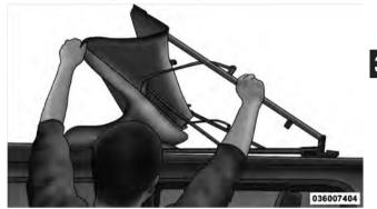
5. Fold the top so that the material forms a "W" as shown. Enter the vehicle and move the material into two folds.
