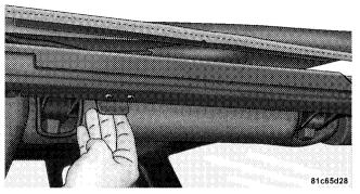
17. Before lowering the top, open the swing gate to prevent possible damage to the rear center high-mounted brake light. Move to the front of the vehicle. Grasp the side bow behind the header and lift the top, folding it toward the rear of the vehicle.
