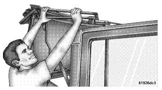
6. Ensure that the top locks into the Sunrider<sup>®</sup> locking mechanisms that are located above the front of the rear doors.
