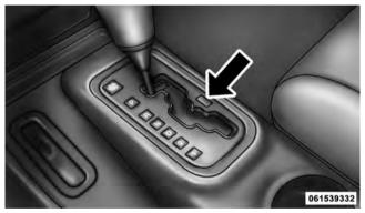
Shift Lever Override Access Cover 4. Press and maintain firm pressure on the brake pedal. 5. Using the screwdriver or similar tool, reach into the opening and press and hold the shift lever override.
