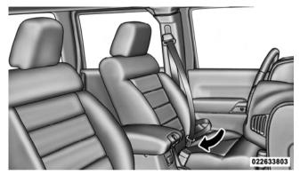
**Inserting Latch Plate Into Buckle**
