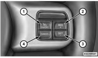
$\begin{array}{ll} 1 - \text{ON/OFF} & 2 - \text{RES} + \\ 4 - \text{CANCEL} & 3 - \text{SET} - \end{array}$
