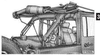
13. The swing gate brackets do not need to be removed 14. Grasp the front side bow behind the header, and lift unless the hard top is being installed. To remove the swing gate brackets, pull the front of the bracket forward while rolling the entire bracket back in toward the vehicle to disengage.
