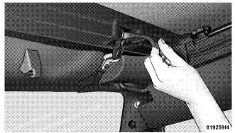
7. If the swing gate brackets were removed, install them by hooking the rear edge of the bracket on the interior side of the body channel. Then, rotate it rearward and over the channel until it snaps onto the exterior part of the rail. To be properly located, the bracket must only be clipped to the shortened rail edge.
