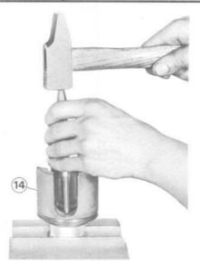
If the nylon stop has been removed refit, it, in the interior of the tulip 14:
