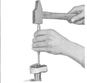
Make three equidistant punch marks, spreading the splines on the shaft towards the hub of the bearing pack, using a centre punch.
