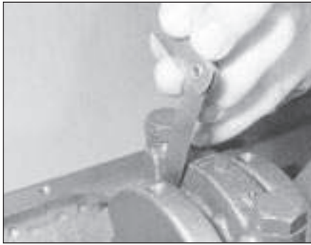
15.9 Using feeler blades to check crankshaft endfloat
