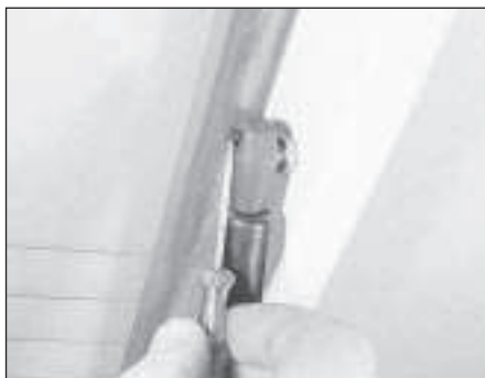
15.5 Releasing tailgate strut retaining clip
