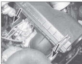
2.5 KE-Jetronic air cleaner retaining bolts (arrowed)
