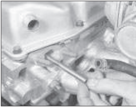
5.9 Removing the fuel pump push-rod
