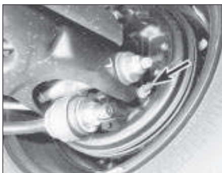
8.5 Handbrake adjustment plunger location (arrowed) on backplate
