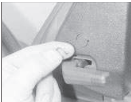
19.5a Remote control mirror handle circlip
