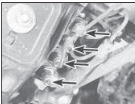
21.8 Hydraulic pipe and hose unions (arrowed) at the pipe bracket on the transmission support crossmember
