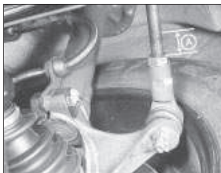
20.3 Steering tie-rod outer balljoint showing exposed threads (A) on tie-rod
