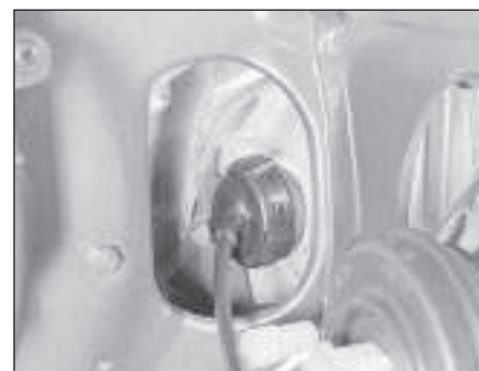
5.8 Front indicator bulbholder accessible through inner wing panel aperture
