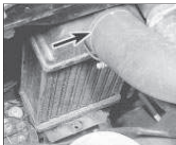
22.3 Intercooler upper air hose attachment (arrowed)
