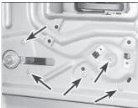
14.40b Regulator retaining rivet location (arrowed)
