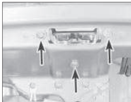
16.3 Tailgate lock retaining screws (arrowed)
