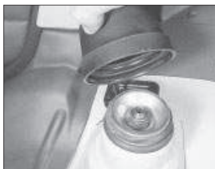
10.3 Rear shock absorber top mounting
