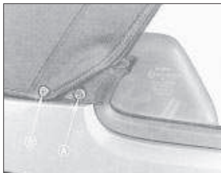
22.5 Protection cover screw (A) and tensioning screw (B) - Cabriolet models
