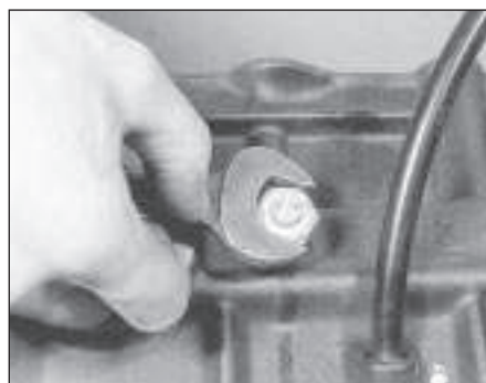
12.25 Unscrew the oil pressure switch
