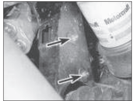
20.3b Drivebelt cover retaining nuts (arrowed) - models up to 1987
