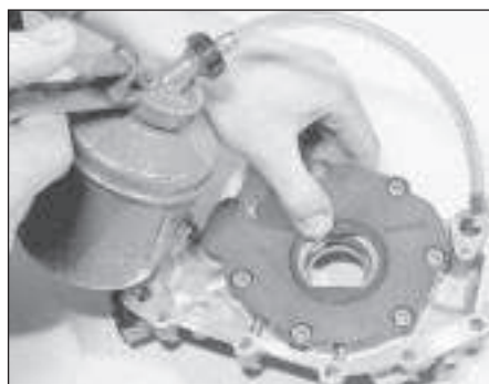
15.12 Priming the oil pump prior to fitting
