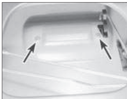
13.3 Door exterior handle retaining screws (arrowed)
