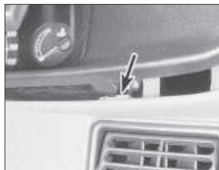
9.8 Bezel lower retaining clip (arrowed) - 1986 models onwards
