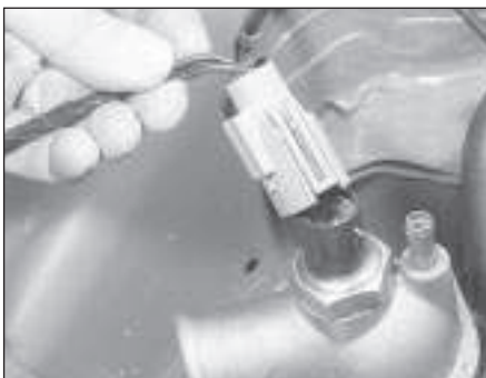
11.49a Disconnecting the cooling fan thermal switch . . .
