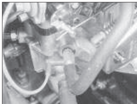
7.9 Vacuum hose attachments at the inlet manifold - 1.4 litre carburettor engine
