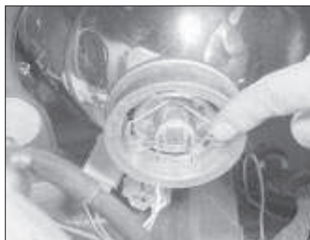
5.2 Releasing headlamp bulb spring clip arms
