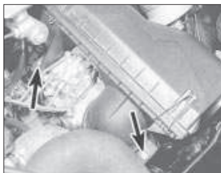
11.66 Air cleaner retaining bolts (arrowed) on RS Turbo models
