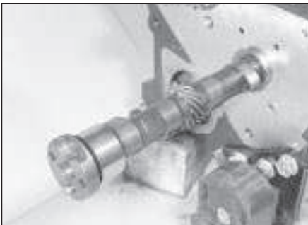
12.33 Withdrawing the camshaft from the front of the engine
