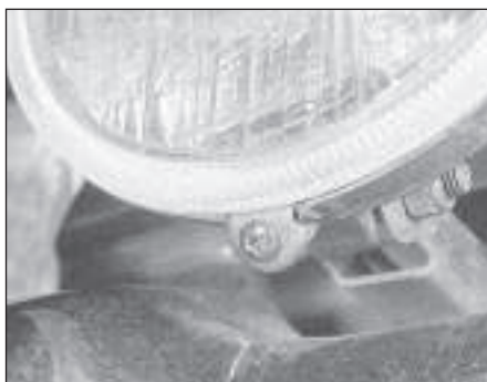
5.16 Front auxiliary lamp lens retaining screw
