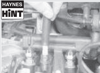
15.10a Measuring the spark plug gap with a wire gauge . . .
