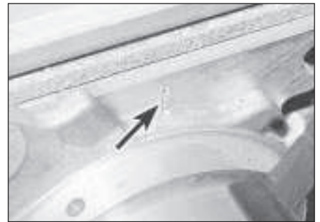
5.45b Distributor mounting flange and cylinder head punch marks (arrowed) - CVH engines (electronic breakerless system - later type distributor shown)
