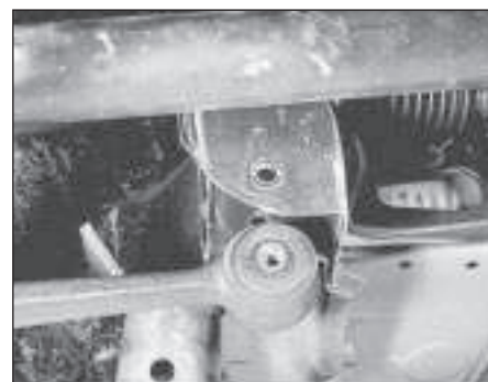
3.3 Suspension lower arm disconnected at inboard end
