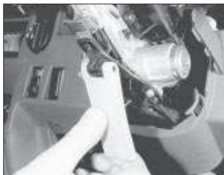
25.8 Removing the bonnet release lever
