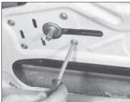
14.40a Removing the regulator retaining screws
