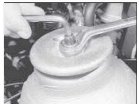
7.4c . . . and strut retaining nut on post-1983 models
