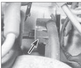
21.1 Waste gate solenoid control valve location (arrowed)
