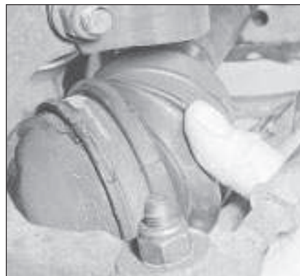
29.3 Checking driveshaft outer joint rubber bellows
