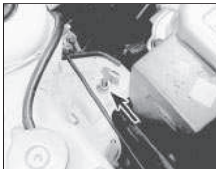
11.29a Rear right-hand engine mounting attachment (arrowed) at side member . . .
