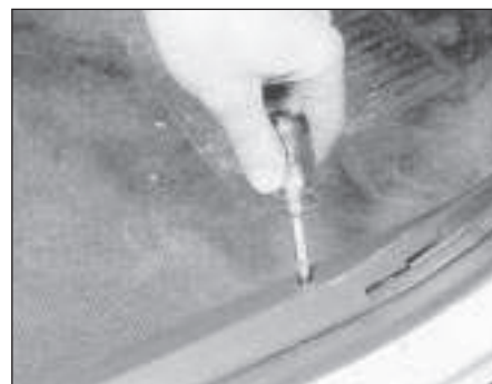
32.7 Removing a sill scuff plate securing screw
