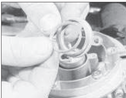
10.7 Removing the seal from the injector retaining collar - 1.4 CFI engine
