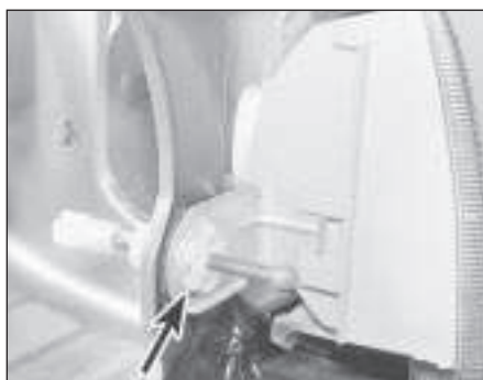
7.9a Release the adjuster by turning the collar (arrowed)
