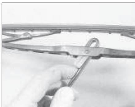
17.2 Disconnecting wiper blade from arm
