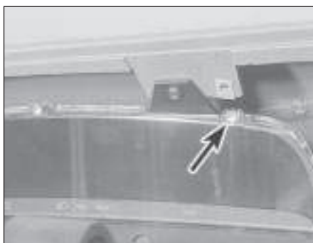
9.9a Instrument panel upper retaining screw (arrowed)
