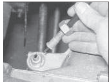
11.50 Disconnecting the speedometer cable - HCS engine
