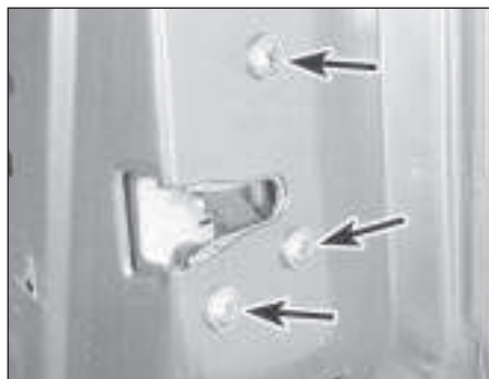
13.14 Door lock retaining screws (arrowed)
