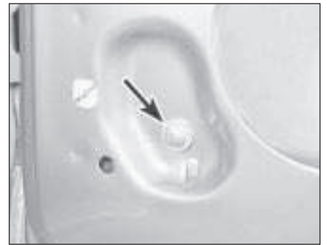
14.5 Glass run extension retaining screw (arrowed)
