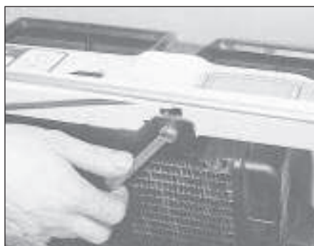
3.5a Undo the radiator upper bolts . . .
