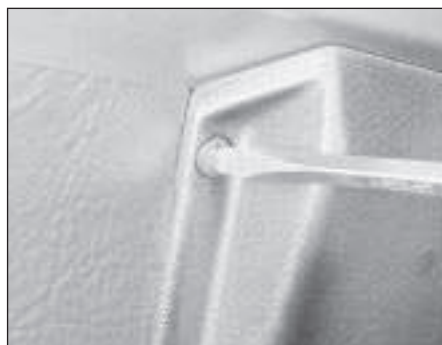
32.25 Releasing a tailgate moulded cover fastener
