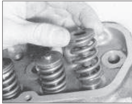
13.39 Remove the valve spring retainer and spring . . .
