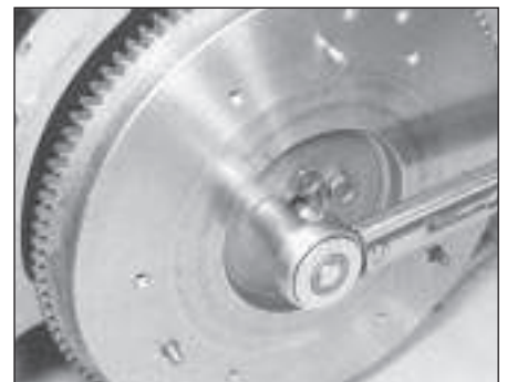
15.18b . . . then refit and secure the flywheel
