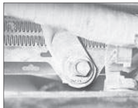
2.20b . . . to gain access to the fan shroud bolts on 1986 RS Turbo models
