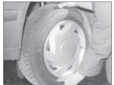
18.3 Rocking the roadwheel to check steering/suspension components
