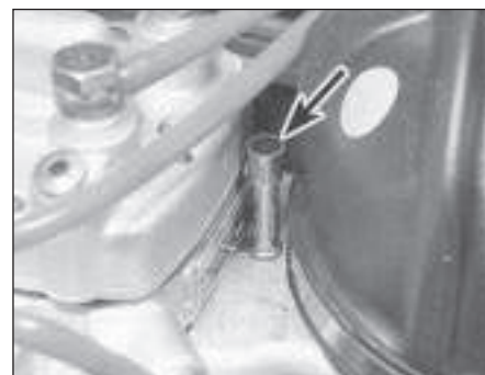
10.21 K-Jetronic system mixture adjustment screw location (arrowed)
