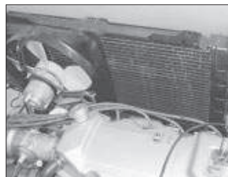
3.5b . . . and lift out the unit complete with fan - pre-1986 models (except RS Turbo)
