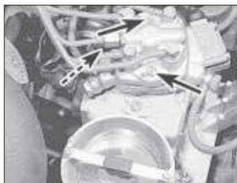
11.11 KE-Jetronic fuel distributor retaining screws (arrowed)
