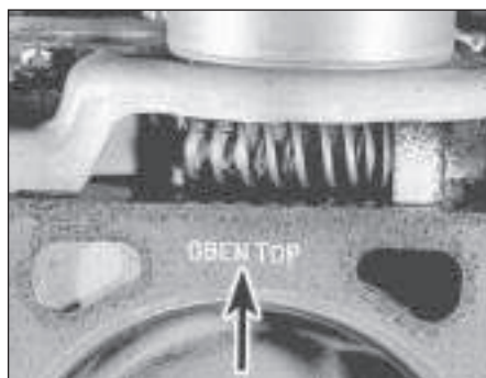
7.22 The upper surface of the cylinder head gasket is marked OBEN-TOP (arrowed)
