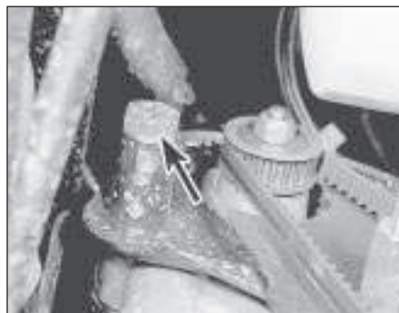
20.5 Modulator adjuster bolt (arrowed)
