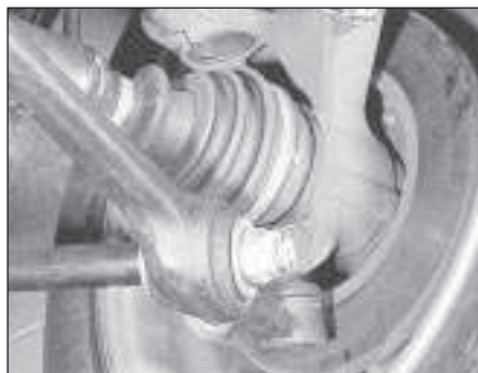
5.4 Anti-roll to lower arm retaining nut
