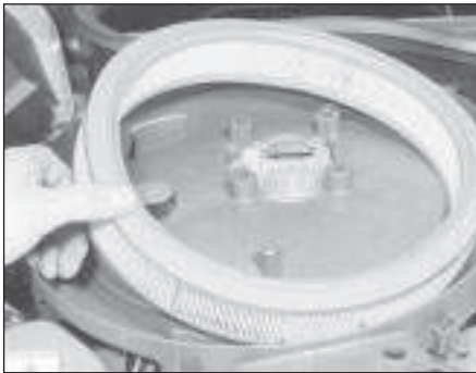
34.3 Removing the air cleaner element
