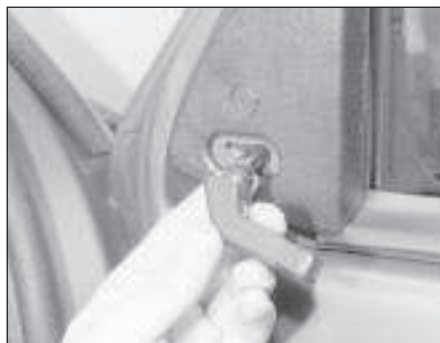
19.5b Removing the remote control handle
