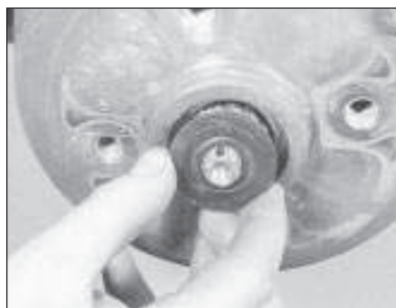
5.3d . . . and remove the thrustwasher
