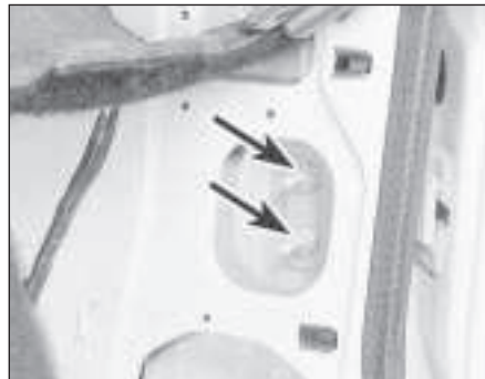
12.7a Front door lower hinge nuts (arrowed)
