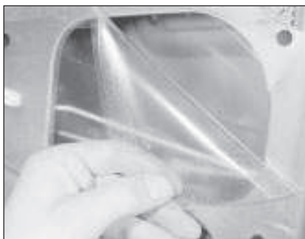
13.2 Peel back the waterproof sheet for access to the door handle
