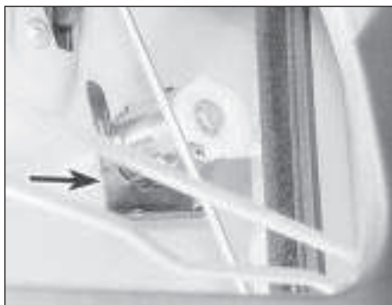
13.13 Door lock cylinder retaining clip (arrowed)
