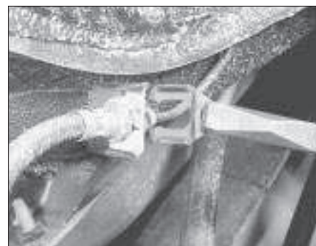
15.1 Removing a flexible hose spring anchor clip
