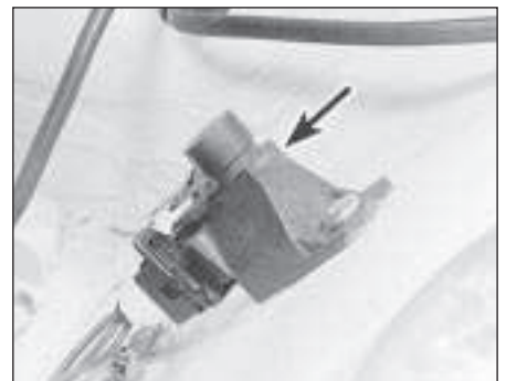
17.1 Mixture (CO) adjustment potentiometer (arrowed) - 1.6 EFI engine
