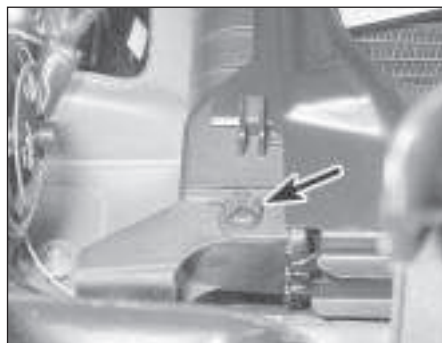
33.3 Radiator drain plug location (arrowed)
