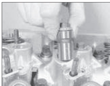
13.42 Fitting a cam follower to its bore
