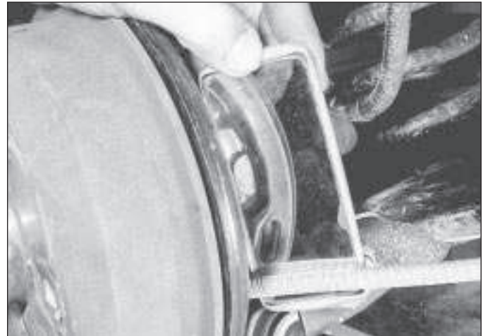
17.1b Checking rear brake lining wear with a mirror
