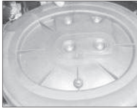
34.1b . . . and air cleaner retaining screw locations on 1.4 litre CVH engine
