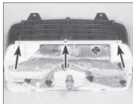
10.11b Instrument panel assembly upper retaining screws - 1986 models onwards
