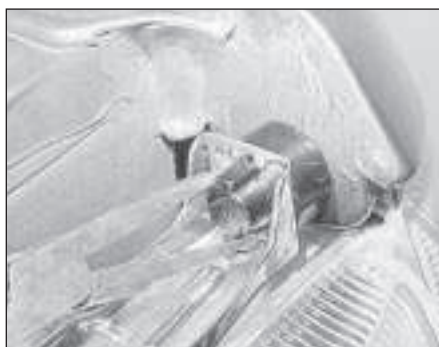
7.3a Releasing the headlamp side plastic retaining clip head
