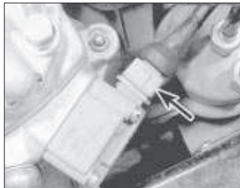
15.5 Pressure actuator wiring multi-plug (arrowed)
