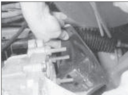
11.65b Removing the mounting bracket - HCS engine
