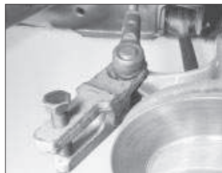
20.6 Releasing tie-rod balljoint using separator tool
