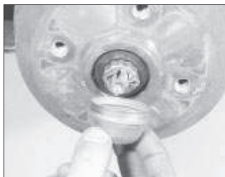
5.3a Remove the rear hub dust cap . . .
