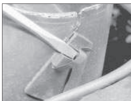
6.10a Release the retaining clips . . .
