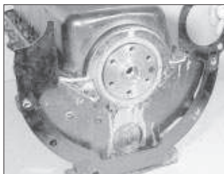
15.21a Locate the adapter plate on the dowels . . .
