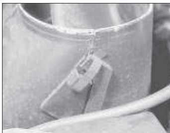
16.4a Release the retaining clips . . .
