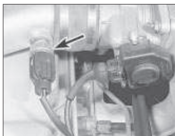
17.1 Charge air temperature sensor location (arrowed)
