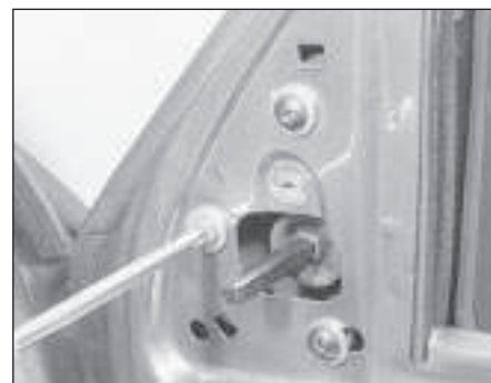
19.7 Removing the door mirror retaining screws
