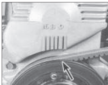
4.3a Crankshaft pulley notch (arrowed) aligned with TDC (0) mark on belt cover scale
