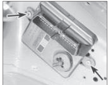
6.19 ESC module securing screws (arrowed)
