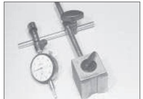
Dial test indicator ("dial gauge")
