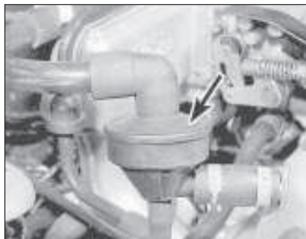
6.3 Crankcase ventilation filter location (arrowed) on KE-Jetronic fuel-injected engines
