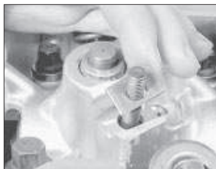
13.43a Fit the rocker arm spacer plate . . .
