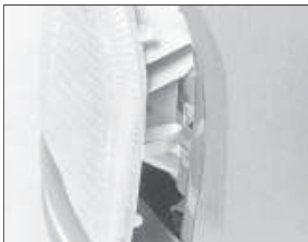
7.10 Release the direction indicator side spring clip
