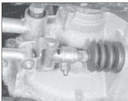
11.19 Disconnect the gearchange rod at the selector shaft clamp
