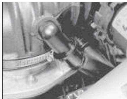
34.7 Detach the shut-off valve hose - K-Jetronic system
