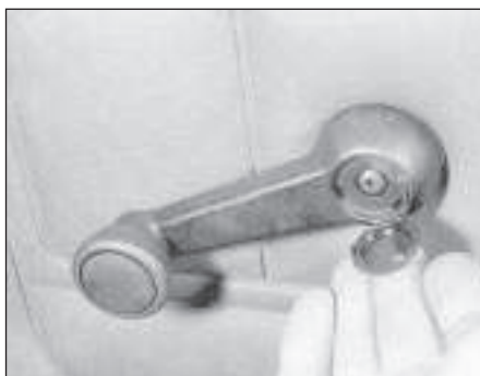
11.2a Prise out the plastic insert . . .
