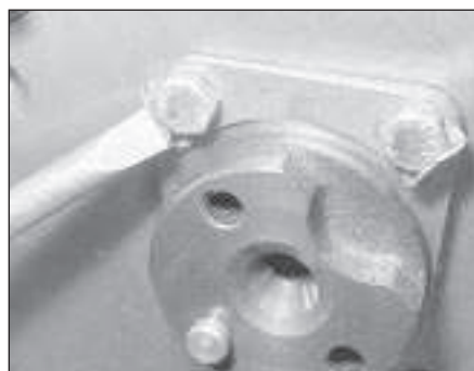
15.3 Secure the camshaft thrust plate bolts with the locktabs
