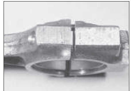
12.37 Connecting rod and big-end cap markings
