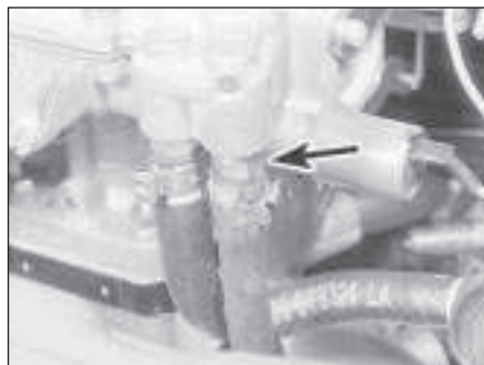
7.8 Fuel return pipe location (arrowed) - 1.4 litre carburettor engine
