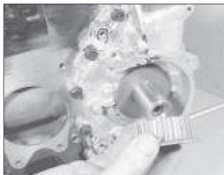
15.17 Fitting the crankshaft sprocket with the flange outward
