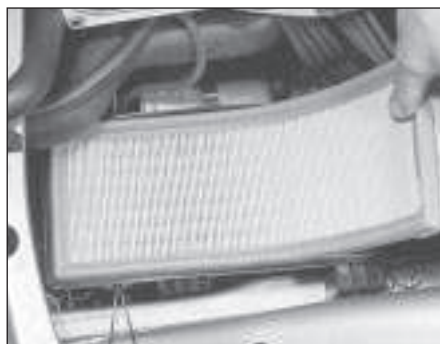
34.10d . . . and withdraw the element - K-Jetronic system
