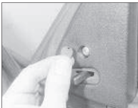
19.6a Extract the trim cover and undo the screw . . .
