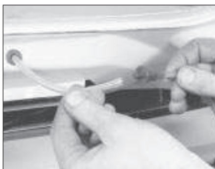
7.2 Disconnecting the windscreen washer fluid pipe
