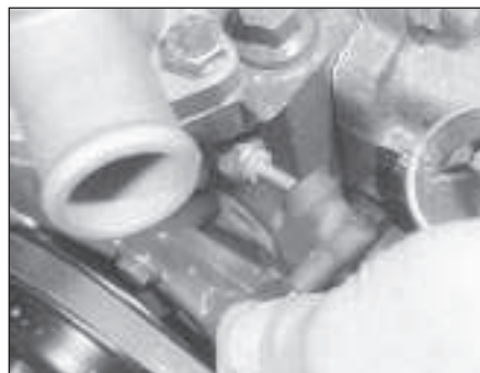
11.49b . . . and coolant temperature sender - HCS engine
