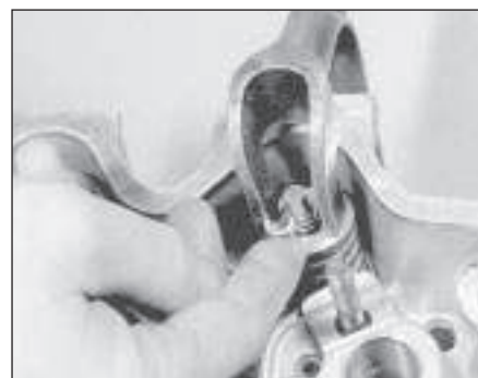
13.38 Compress the spring and fit the collets
