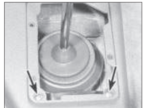
30.3a Centre console lower retaining screws (arrowed)
