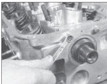
6.13a Unscrew the camshaft thrust plate bolts . . .
