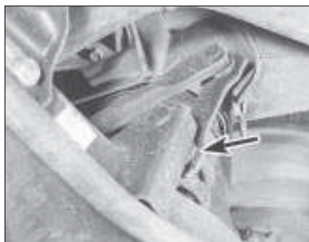
13.3 Anti-roll bar-to-lower arm shackle attachment (arrowed)
