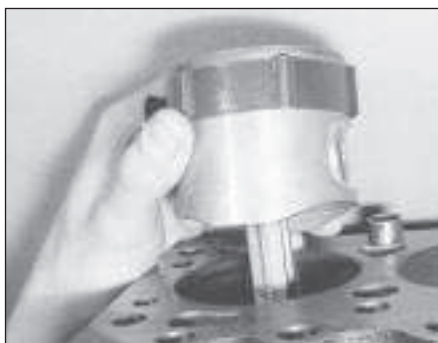
8.12 Fitting a piston/connecting rod assembly with ring compressor in position
