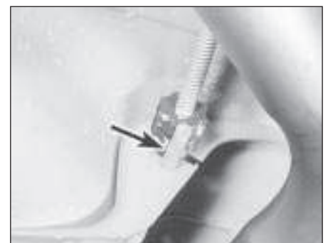
8.14 Handbrake cable adjuster nylon locking pin (arrowed)
