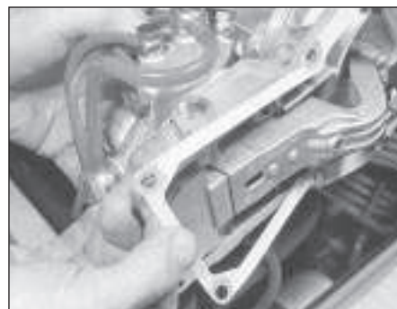
34.12 Locating the sensor unit gasket
