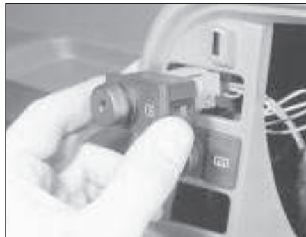
4.37 Rear foglamp switch removal - models from 1986 onwards
