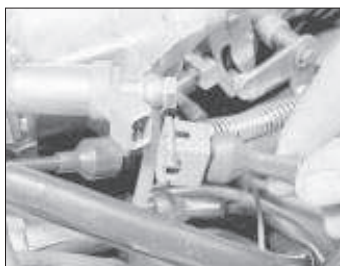
9.2 Disconnecting the cold start valve wiring multi-plug
