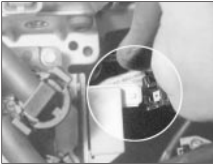
6.15A Disconnect the wiring multi-plug (arrowed) from the ignition coil ..
