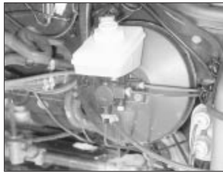
12.2A Brake master cylinder and hydraulic line connections
