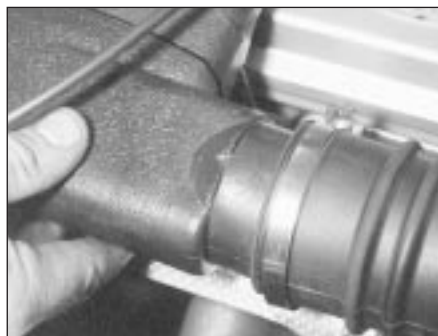
4.24 Detach the air inlet hose from the inlet duct. Note the small projection on the end of the hose which engages with a cut-out in the inlet duct
