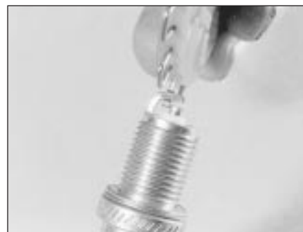
27.13 To change the gap, bend the outer electrode only, and be very careful not to crack or chip the porcelain insulator surrounding the centre electrode
