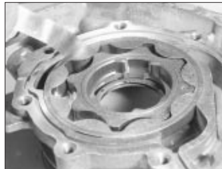
17.3A Outer rotor-to-oil pump body clearance check
