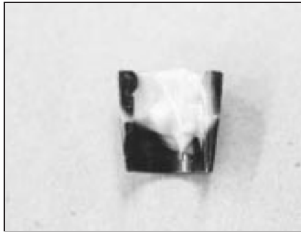
10.18 Apply a small dab of grease to each collet before installation - it will hold them in place on the valve stem until the spring is released
