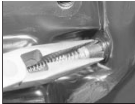
23.6A Compress the handbrake cable retaining lugs to release the cable from the brake backplate
