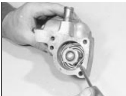
4.6A Release the retaining clip . . .
