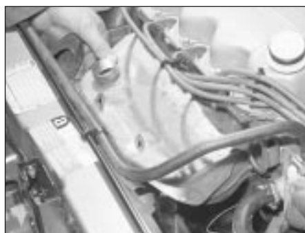
7.1A Removing the hot-air shroud from the 1.6 litre carburettor engine
