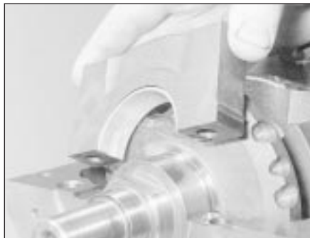
20.12 Refit the main bearing caps and tighten the bolts as specified
