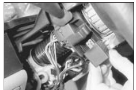
3.7 Direction indicator flasher relay removal
