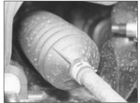
19.2C Check the condition of the steering rack gaiters
