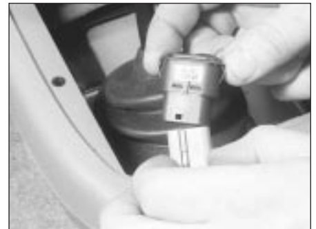
4.46 Electric window switch removal
