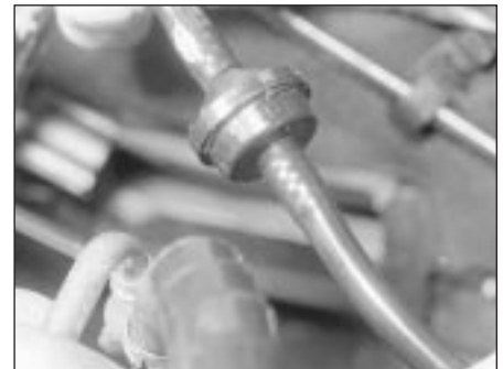
19.5 Non-return valve in the servo vacuum hose
