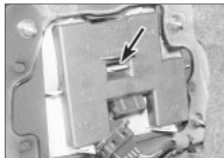
5.31B On later models, press the bulbholder retainer (arrowed) upwards and pull free the bulbholder
