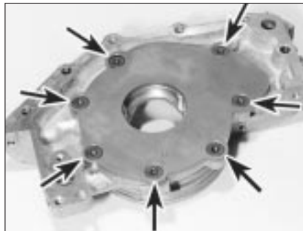
17.2 Oil pump cover plate retaining screws (arrowed)
