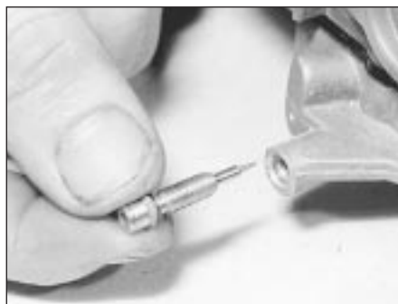
17.14 Unscrew and remove the fuel mixture screw
