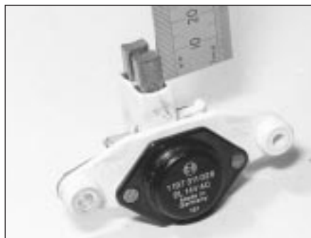
14.4 Measuring the brush lengths (Bosch K1 alternator)
