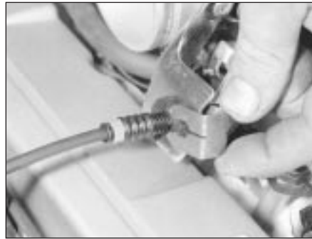
6.5B . . . then release the cable adjusting clip and withdraw the cable from the support bracket
