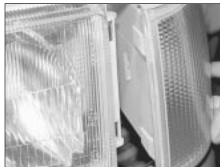
5.17 Engage the tags in their locating slots when refitting the front indicator unit
