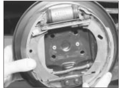
6.4 Disengage the leading brake shoe from the bottom anchor . . .
