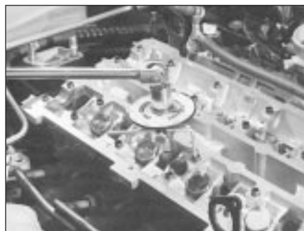
14.30C . . . and to Stage 3 using angle gauge
