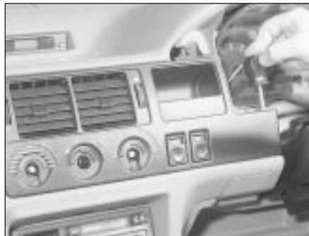
11.49B . . . undo the retaining screws . . .
