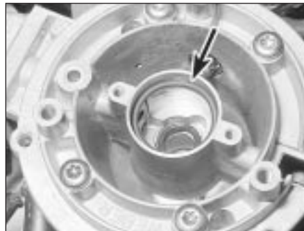
15.9D Injector seal location (arrowed) in the CFI unit
