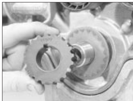
11.8 Note "FRONT" marking on outside face of crankshaft toothed pulley - note which way round thrustwasher behind is fitted
