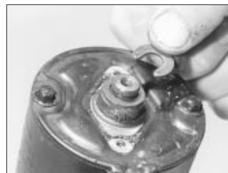
18.3 Remove the C-clip and any washers (Bosch starter motor)
