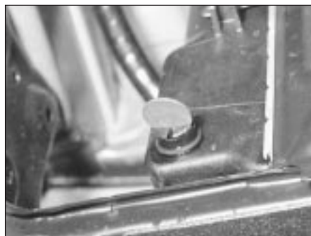
28.3 Use a small coin to unscrew the radiator drain plug
