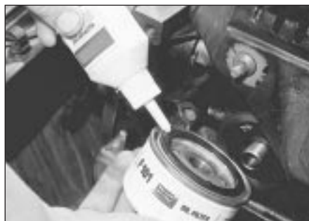
16.10A Lubricate the filter's sealing ring with clean engine oil before installing the filter on the engine
