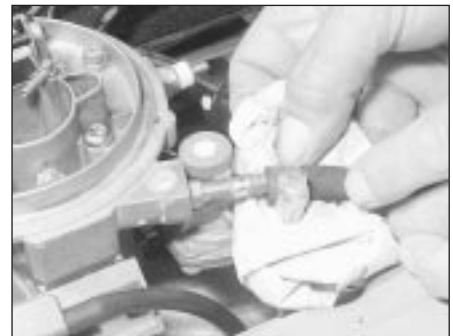
23.6 Disconnecting the fuel line at the carburettor
