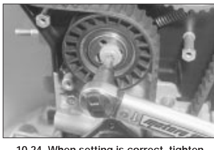
10.24 When setting is correct, tighten tensioner bolt to specified torque wrench setting
