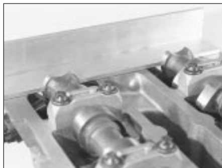
13.21B Fit camshaft-aligning tool to set TDC position while camshaft toothed pulleys are refitted
