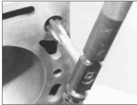
14.6 All bolt holes in the block - particularly the main bearing cap and head bolt holes - should be cleaned and restored with a tap (be sure to remove debris from the holes after this is done)
