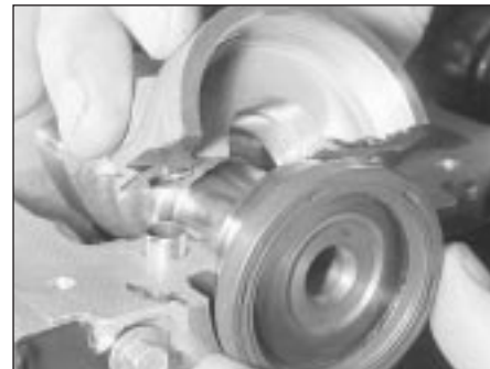
12.6 Alternatively, seal can be inserted when camshaft bearing cap is unbolted
