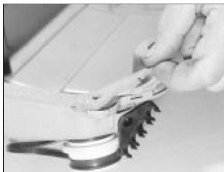
5.9A Fitting a new gasket to the rocker cover
