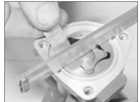
16.4C Checking the rotor endfloat
