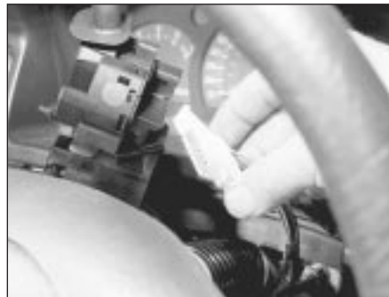
4.8B . . . lift the switch clear and detach the wiring connector
