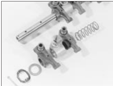
9.4B Partially-dismantled rocker shaft
