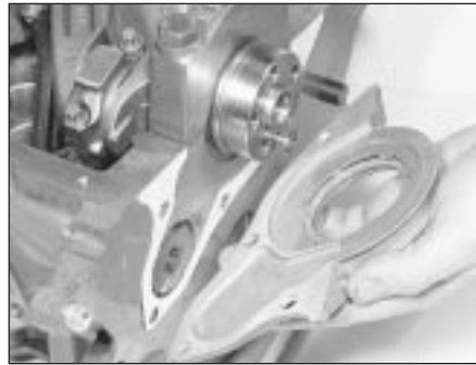
17.14B Fitting the rear oil seal housing with a new gasket in position on the rear face of the cylinder block
