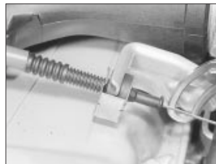
5.6 Accelerator outer cable location at the adjuster/support bracket
