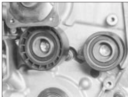
11.13 Tighten timing belt guide pulley bolts to specified torque settings on refitting
