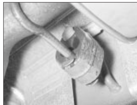
21.2 If any of the exhaust system rubber mountings are to be renewed, ensure that the replacements are of the correct type - their colour is a good guide. Those nearest to the catalytic converter are more heat-resistant than the others
