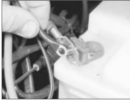
2.1 Detaching the earth leads from the stud of the battery negative (earth) terminal post
