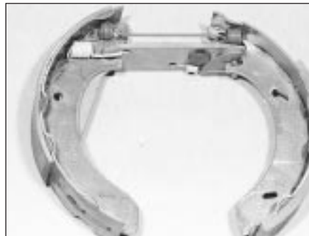
6.12B Brake shoes, strut and upper springs reconnected
