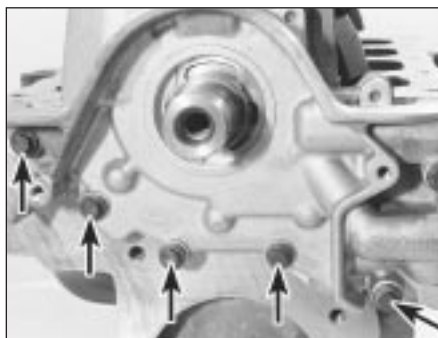
16.5 Unscrew bolts (arrowed) to remove oil pump
