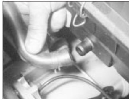
4.13 Detach the crankcase breather hose from the air cleaner housing
