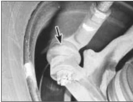
19.2A Check the condition of the track rod end balljoint dust cover (arrowed)
