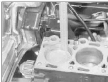
14.21 Position No 1 piston 20 mm down the bore
