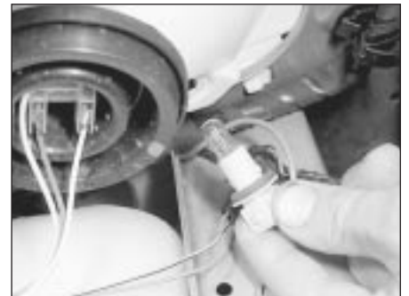
5.7 . . . and withdraw the sidelight bulbholder
