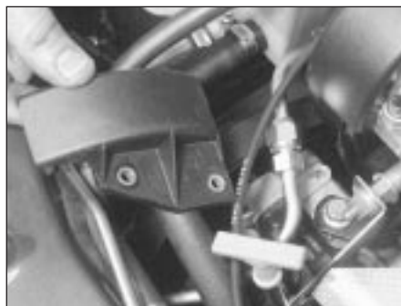
26.2 Remove the drivebelt upper guard from the top of the power steering pump on Zetec engines
