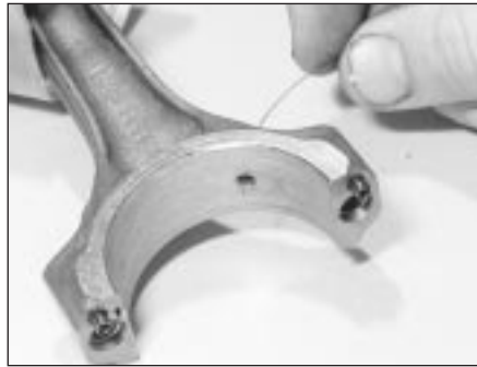
15.12 Check that the connecting rod oilway on CVH engines is clear
