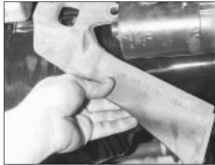
15.6B Auxiliary bracing bracket removal from the starter motor side of the engine - 1.6 litre engine only
