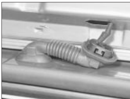
21.4 Detach the wiring connector from the tailgate
