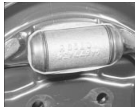
6.5B Elastic band fitted round the wheel cylinder to prevent piston ejection
