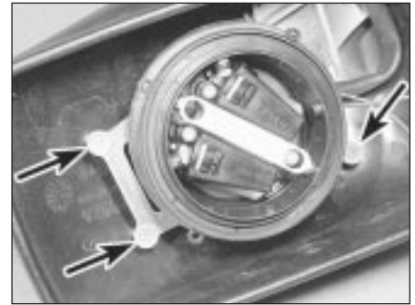
17.6 Mirror motor and retaining screws (arrowed)
