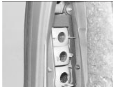
7.34 Rear light lens showing the retaining nuts
