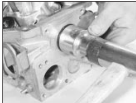
13.22 Driving a new blanking plug into position
