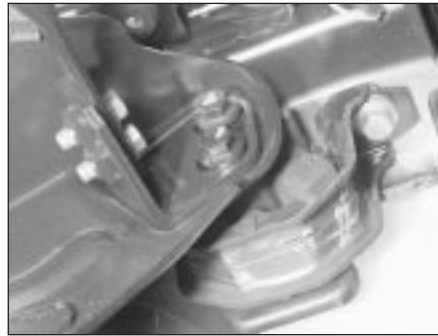
19.8 Engine/transmission left-hand front mounting attachments
