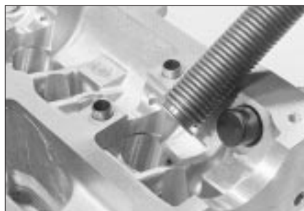
8.22B . . . can be replaced by home-made tool if suitable spring can be found
