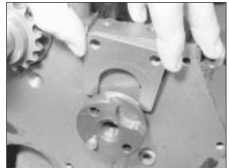
11.17 Refitting the camshaft thrust plate
