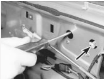
11.3 Undo the glass-to-regulator screws through apertures shown
