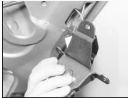
23.5B . . . and withdraw the lock from the tailgate
