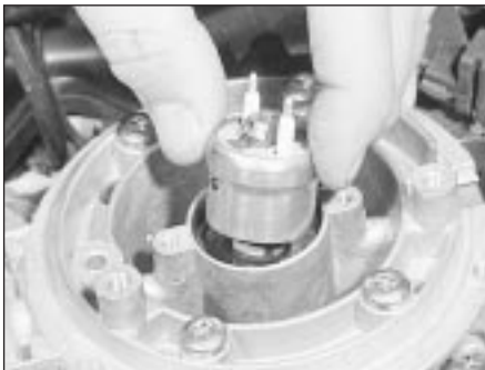
15.9C Withdraw the injector from the CFI unit
