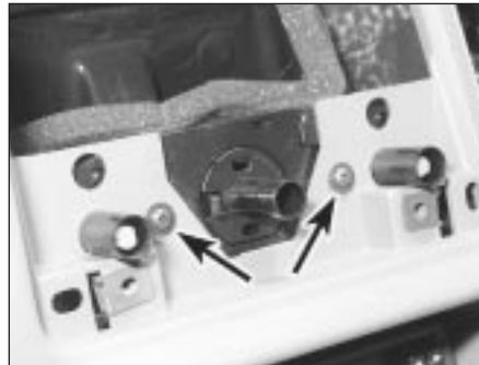
12.3A Control panel retaining screws (arrowed)
