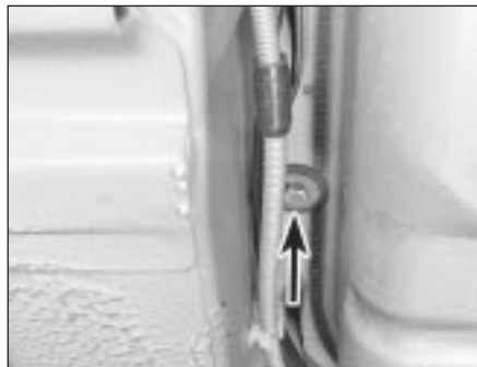
8.7B Fuel tank securing bolt at the front edge
