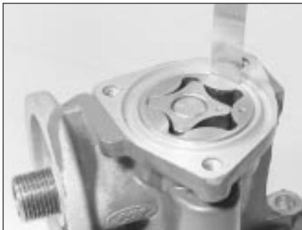
16.4A Checking the outer body-to-rotor clearance
