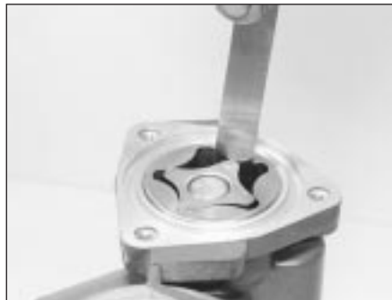
16.4B Checking the inner rotor-to-outer rotor clearance
