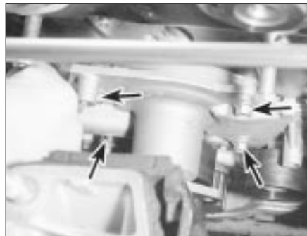
10.5 Unscrew the bolts (arrowed) to remove the water pump
