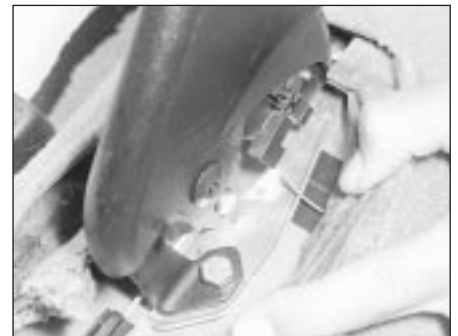
21.4 Prise back the carpet for access to the handbrake warning light switch lead connection and lever mounting bolts
