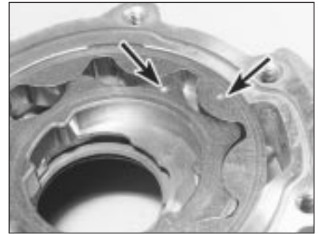
17.4 Inner and outer rotor matchmarks (arrowed)
