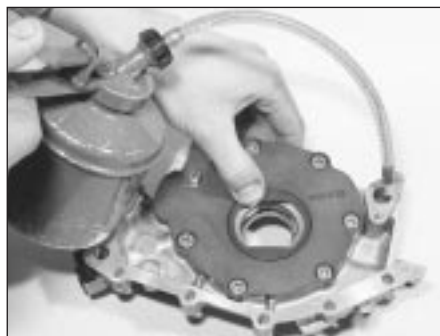
16.8 Prime the oil pump prior to fitting
