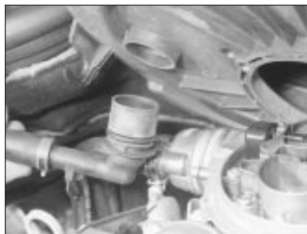
2.4A Disconnecting the oil separator/crankcase ventilation hose from the air cleaner (CVH engine)
