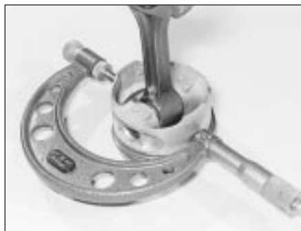
14.13 Measure the piston skirt diameter at right-angles to the gudgeon pin axis, just above the base of the skirt
