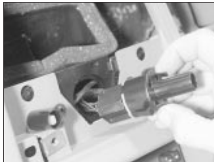
4.42 Heater blower motor switch removal
