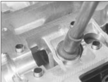
13.6A Removing hydraulic tappets
