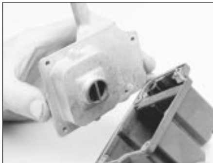
6.30A Remove the four screws to release the filter housing top from the base ...
