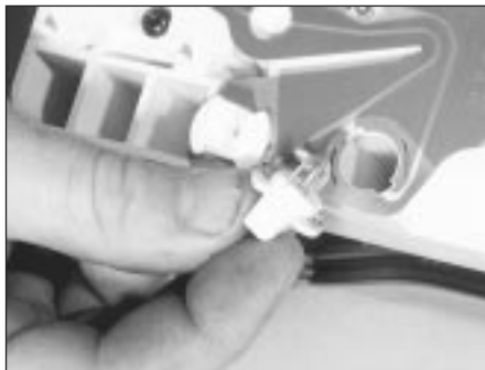
6.8 Bulbholder removal from the instrument panel
