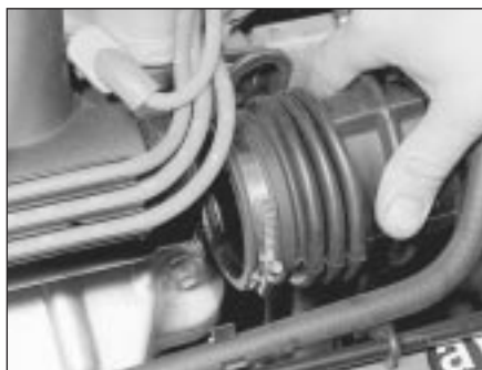
16.4 Disconnecting the hot-air duct from the exhaust manifold
