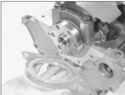
17.15 Use new gasket when refitting left-hand oil seal carrier
