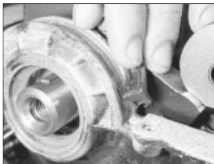
14.8B Lugs of cork gasket halves to fit under the cut-outs in the rubber gaskets
