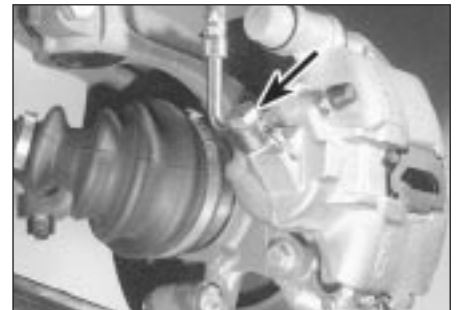
3.3 Unscrew the brake hose-to-caliper banjo union bolt (arrowed) and recover the copper sealing washers
