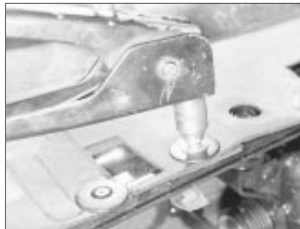
7.12 Pop-riveting the anti-splash shield to the radiator
