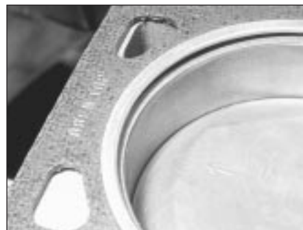
14.22A Fit the cylinder head gasket with the "OBEN/TOP" marking upwards . . .
