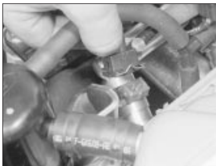
16.10A Disconnect the wiring connector from each injector . . .
