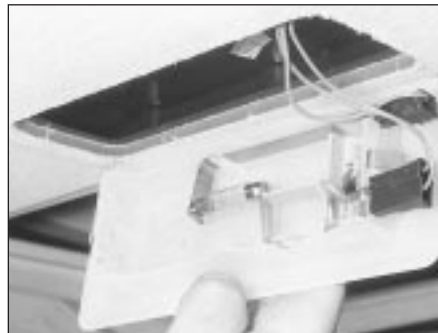
6.1 Roof-mounted courtesy light removal
