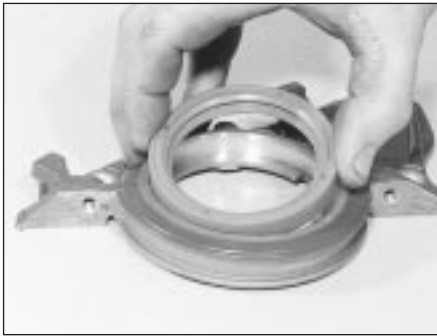
17.14A Positioning the crankshaft rear oil seal in its housing
