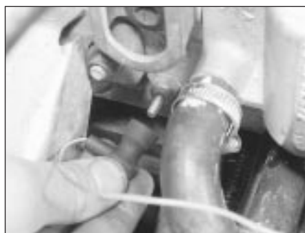
5.12A Disconnect the wiring at the temperature gauge sender unit . . .
