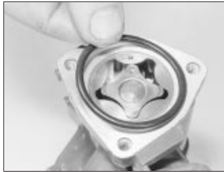
16.1 Extract the O-ring from the groove in the oil pump
