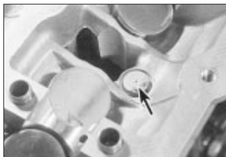
8.24 Cylinder head oil-retaining valve (arrowed)
