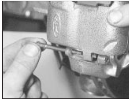
2.2B . . . and withdraw the pin from the base of the caliper
