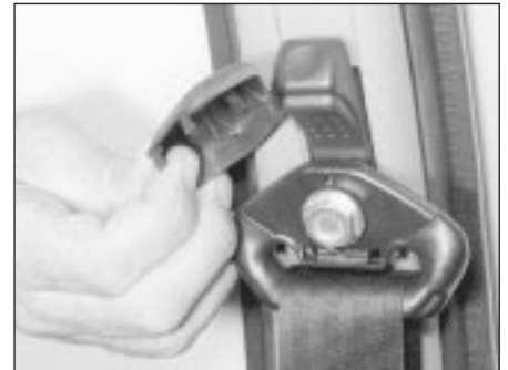
33.7 Remove the cover for access to the seat belt upper anchor bolt
