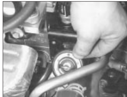
4.19 Ensure that the thermostat is fitted as shown
