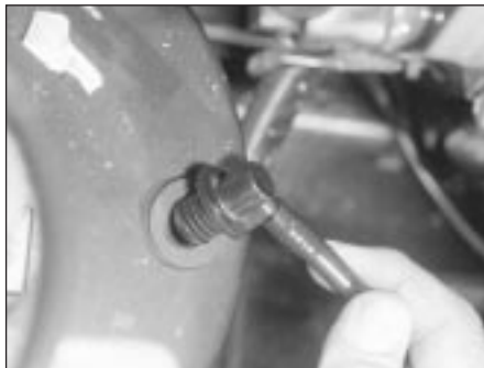
19.2 Detaching the vacuum hose from the servo unit
