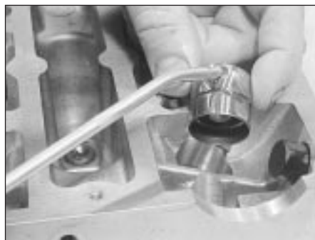
13.17 Oil liberally when refitting hydraulic tappets
