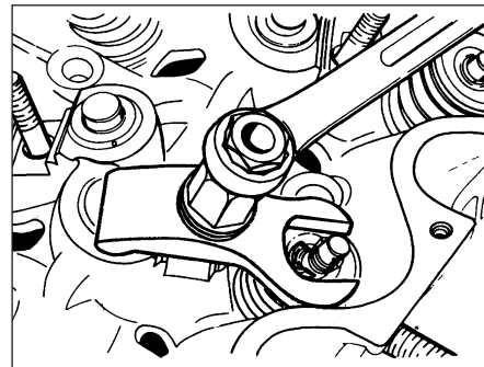
8.11 Compressing a valve spring using a forked type compressor
