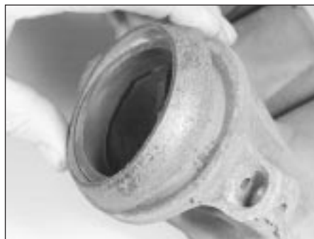
7.12B Renew exhaust system downpipe-to-manifold gasket to prevent leaks
