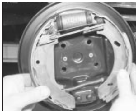
6.5A . . . then from the wheel cylinder at the top
