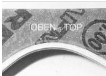
10.22A Cylinder head gasket top-face marking ("OBEN")
