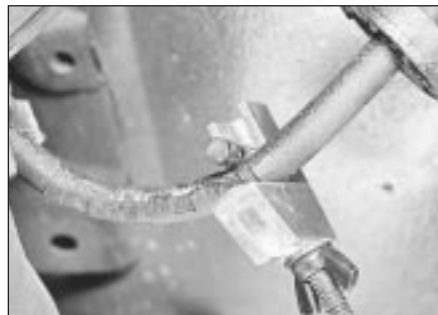
16.7A Brake hose clamp fitted to minimise fluid loss
