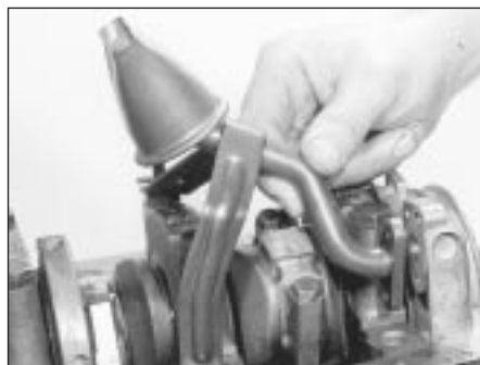
16.4 Removing the oil inlet pipe
