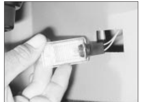
6.4 Luggage area light removed for bulb replacement
