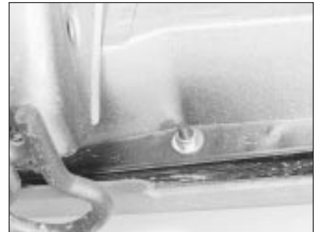
6.10C Rear (lower) bumper retaining nut (Estate models)
