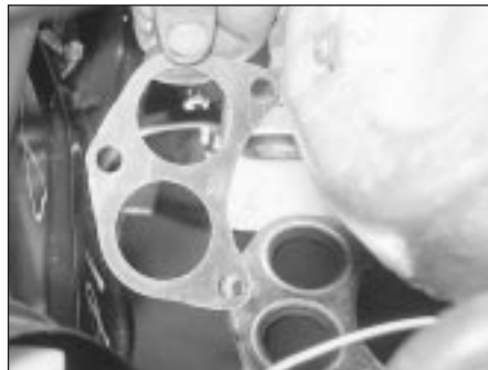
7.9B . . . and manifold-to-exhaust downpipe connection
