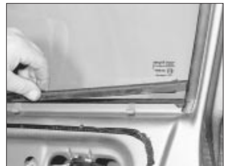
11.2 Remove the weatherstrips from the door
