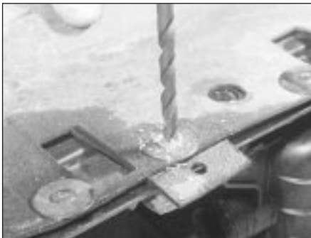
7.9B Drilling out a radiator-to-splash shield rivet
