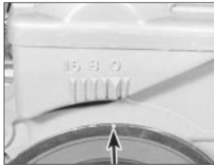
4.6A Crankshaft pulley notch (arrowed) aligned with the TDC (0) mark on the timing belt cover
