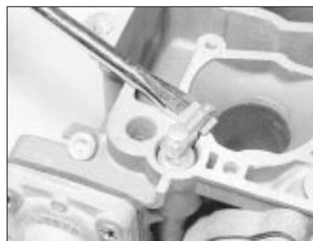
17.10 Carefully prise out the accelerator pump discharge tube assembly
