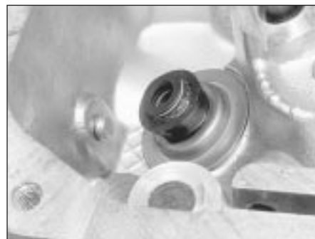
10.8 Locate the seal, and tap it into position over the guide
