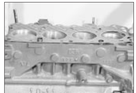
10.22B Cylinder head gasket in position on the top face of the cylinder block
