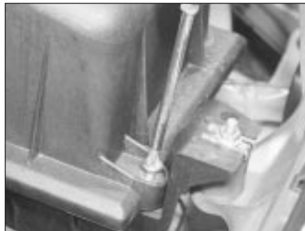
29.1D On EFI and SEFI engines, undo the air cleaner cover retaining screws . . .
