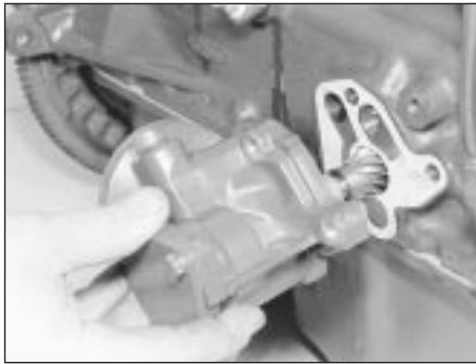
15.7 Refitting the oil pump. Note the new gasket
