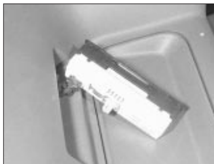
6.21B . . . for access to the bulbholder
