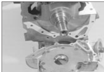
16.12 Use new gasket when refitting oil pump
