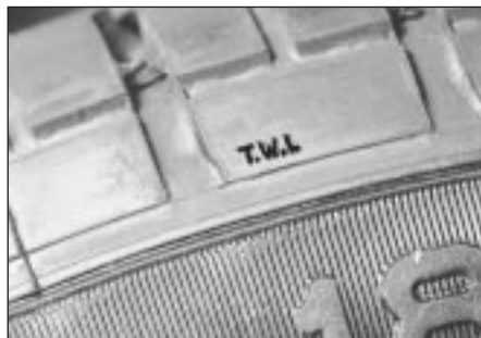
4.2 The TWI marks on the side of the tyre shows the position of the tread wear indicator bands
