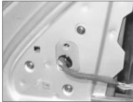
17.5 Undo the three mirror retaining screws
