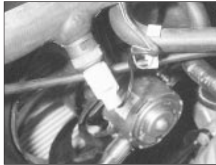
5.2B Cooling fan thermostatic switch location (arrowed) in the radiator top hose (Zetec engine)
