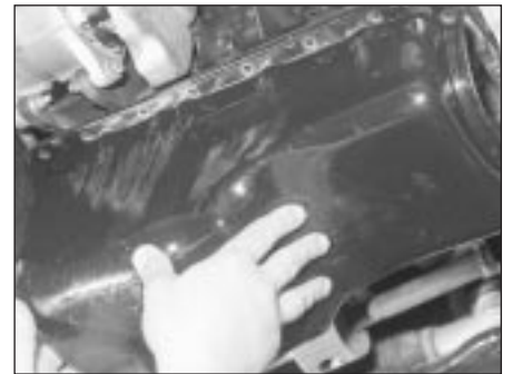
15.8 Removing the sump from the engine
