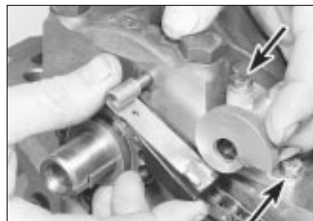
13.5 Chain tensioner arm removal from the pivot pin. Note tensioner retaining bolts (arrowed)
