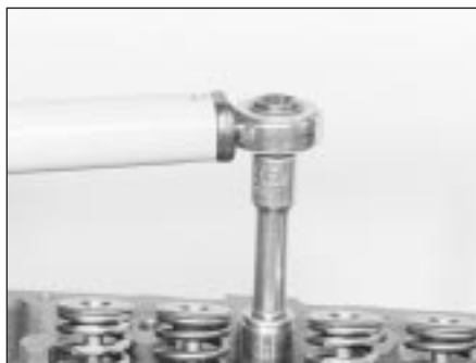
10.24B Tightening the cylinder head bolts (Stage 1)
