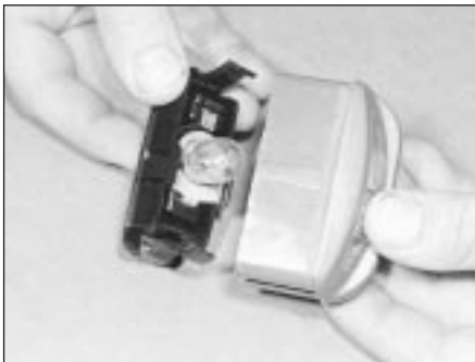
5.42B . . . and separate the number plate light unit and bulbholder
