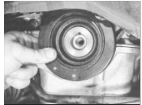
8.4B Ensure pulley is located on crankshaft Woodruff key on reassembly
