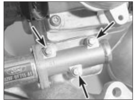
17.33 Unscrew the three retaining bolts (arrowed) and withdraw the idle speed control valve from the inlet manifold
