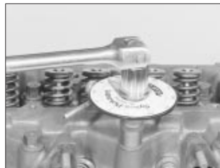
10.24C Cylinder head bolt tightening (Stages 2 and 3) using an angle gauge
