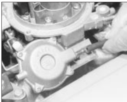
23.7 Disconnecting the vacuum hose from the secondary venturi diaphragm unit
