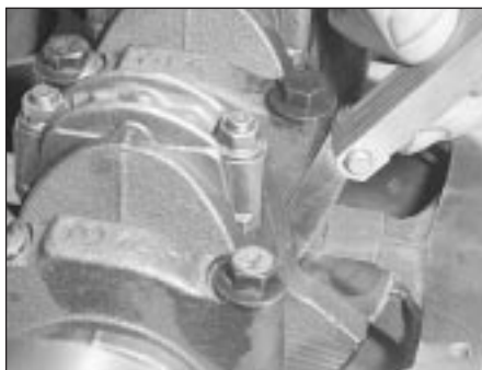
13.3 Checking crankshaft endfloat with a feeler gauge
