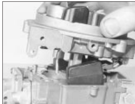
17.2B ... and remove the carburettor upper body
