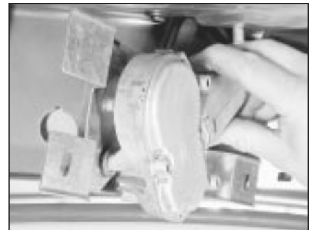
18.7C Removing the wiper motor from the tailgate (Hatchback models)
