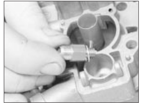
14.7 Remove the needle valve housing and its washer
