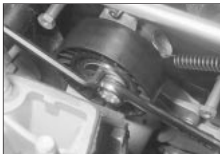
10.18 . . . then use Allen key to position tensiometer so that timing belt can be refitted
