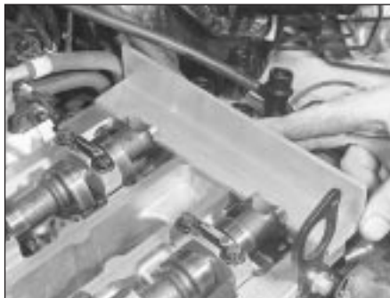
10.8 Fit camshaft-aligning tool to ensure engine is locked with Nos 1 and 4 cylinders at TDC
