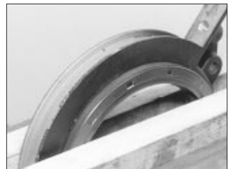
18.19 Rear oil seal installation - housing mounted in a vice with protected jaws
