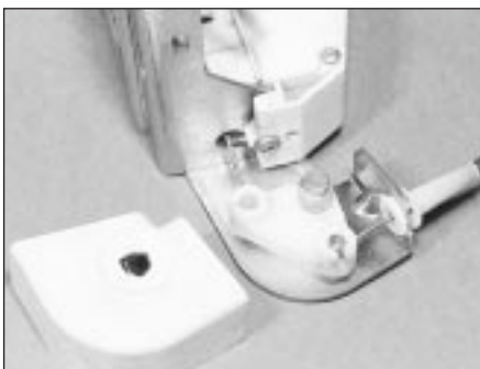
15.8C Remove cover to detach cable from the lock
