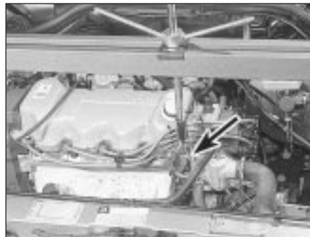
5.34 Connect a suitable lift hoist and sling to the engine, connecting to the lifting eyes
