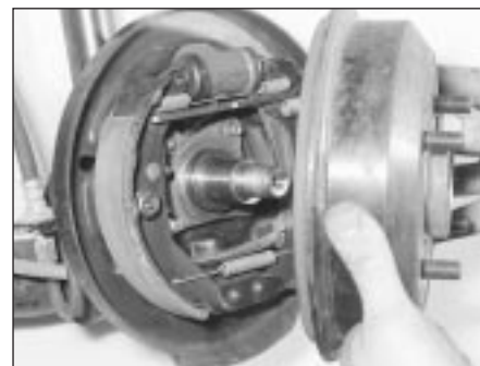
11.9 . . . and remove the brake drum
