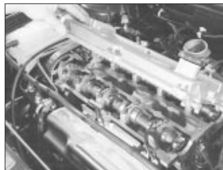
5.6 Removing cylinder head cover
