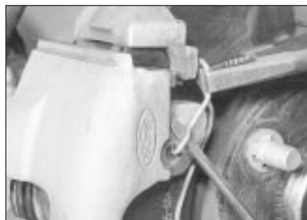
2.16 Hold the caliper support spring with a pair of pliers, and prise it out of its location in the caliper housing using a screwdriver
