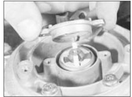
15.9B . . . and remove the injector retaining collar
