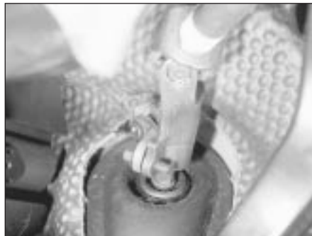
21.7 Steering column-to-pinion shaft coupling and clamp bolt
