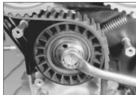
10.20 Slacken tensioner bolt to give initial belt tension
