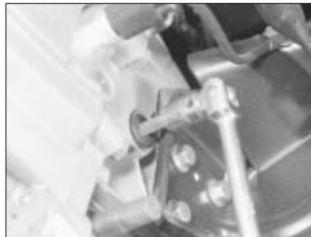
18.1 Unscrewing the manual transmission oil filler/level plug
