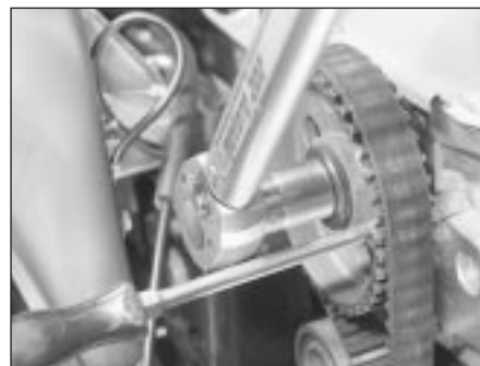
11.13B . . . and tighten the retaining bolt to the specified torque whilst retaining the sprocket as shown
