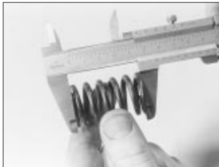
9.18 Checking the valve spring free length
