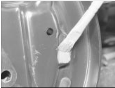
6.10A Applying high-melting-point grease to the brake backplate
