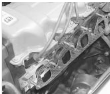
7.9A Fit a new gasket to the exhaust manifold . . .
