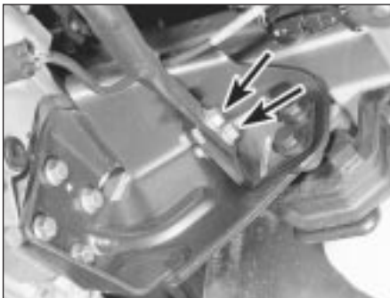
5.33 Remove the brace between the transmission left front mounting bracket and the transmission flange
