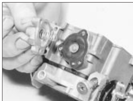
17.12B ... then detach the cover, return spring and diaphragm
