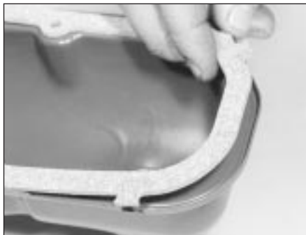
5.5A Engage tags of rocker cover gasket into the cut-outs in the cover
