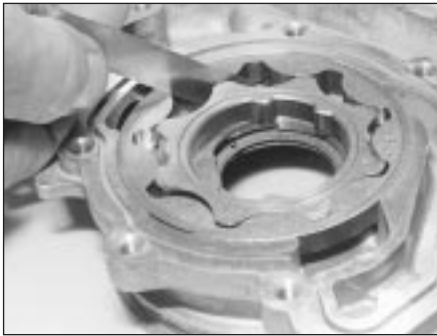
17.3B Outer-to-inner rotor clearance check
