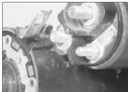
18.5 Detach the brush link lead (Bosch D-type starter motor)
