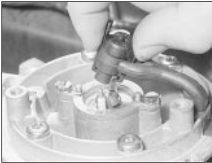
15.8 Disconnect the multi-plug from the injector
