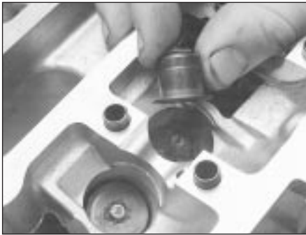
10.16 Valve spring pressure is sufficient to seat lower seat/stem oil seals on reassembly
