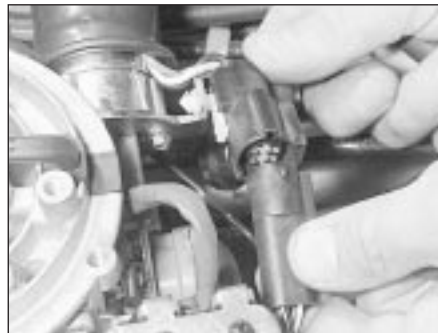
15.35A Disconnecting the throttle plate control motor multi-plug
