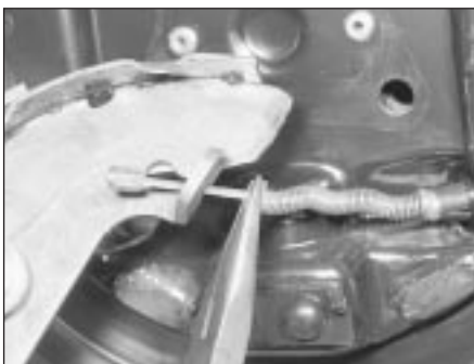
6.7A Disconnecting the handbrake cable from the trailing brake shoe
