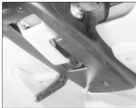
21.3B ... and lower steering column shrouds
