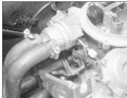
20.2 Coolant hose connections to the automatic choke unit
