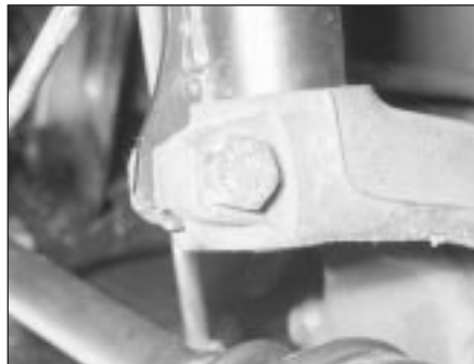
2.9A Remove the suspension strut-to-spindle carrier clamp bolt . . .
