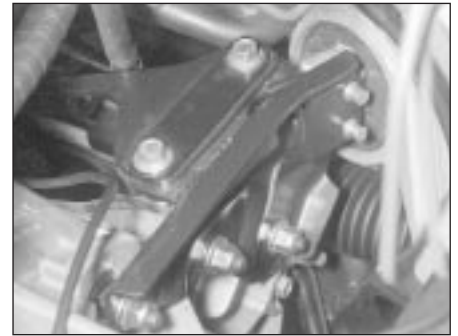
19.12 Engine/transmission left-hand rear mounting and mounting bracket attachments
