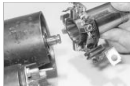
18.9 Brush plate unit assembled over a socket with the same outside diameter as the commutator to ease assembly
