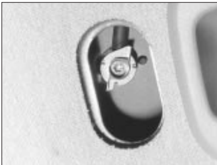
23.2 Roof-mounted aerial retaining screw
