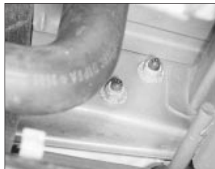
6.4 Front bumper retaining nuts
