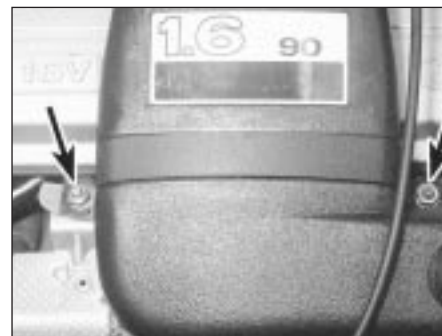
4.25 Undo the two nuts (arrowed) and lift off the air inlet duct retaining strap
