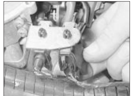
15.35B Releasing the throttle position sensor multi-plug from the retaining clip
