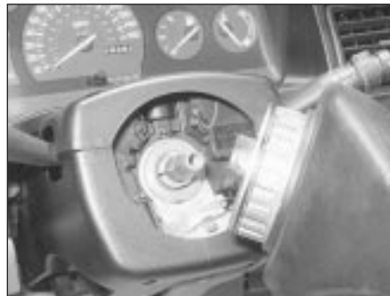
20.5B . . . and withdraw the steering wheel
