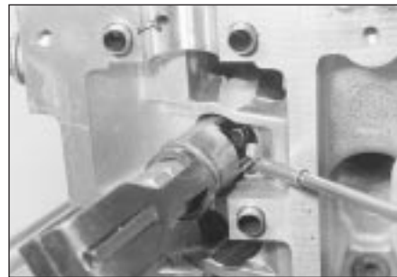
8.19C . . . so that both valve split collets can be removed from the valve's stem - small magnetic pick-up tool prevents loss of small metal components on removal and refitting
