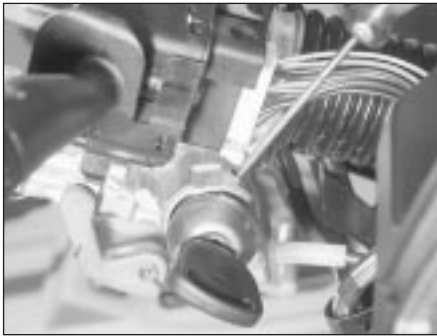
22.3 Releasing the steering lock
