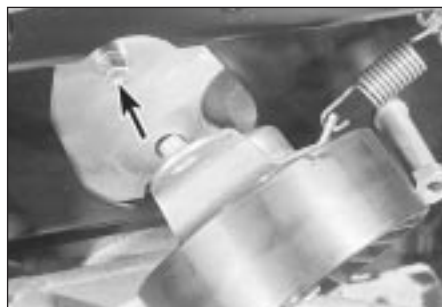
10.17B Hook spring onto tensioner and refit as shown - engage tensiometer backplate on locating peg (arrowed) . . .
