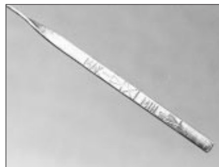
3.4 Engine oil dipstick MAXimum and MINimum level markings
