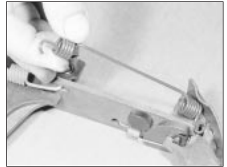
6.11 Reconnect the upper return spring to the leading . . .
