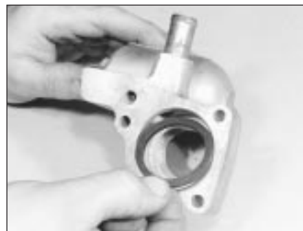
4.6C . . . and where applicable, remove the O-ring seal
