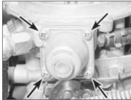
15.13 Fuel pressure regulator and retaining screws (arrowed) - shown in situ
