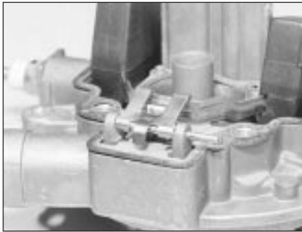
14.6A Slide out the float retaining pin ...
