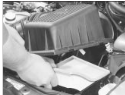
29.1F . . . then lift off the cover and withdraw the element
