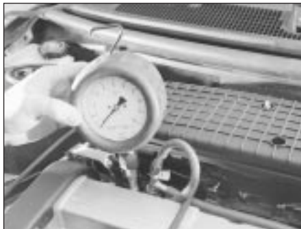
7.5 Fuel pressure gauge connected to the fuel line
