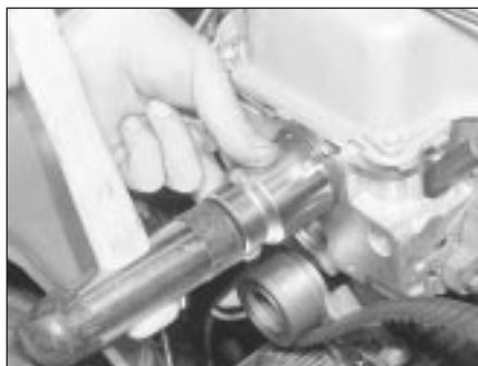
12.3 Using a socket to tap the camshaft oil seal into place
