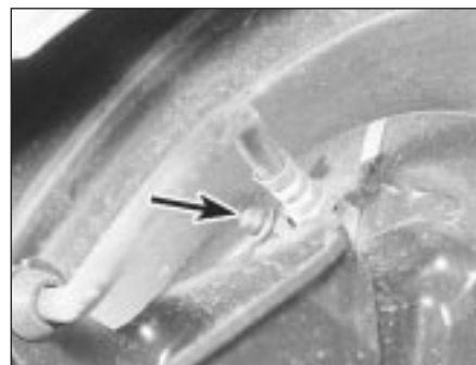
17.14 Rear brake bleed nipple and dust cap (arrowed)
