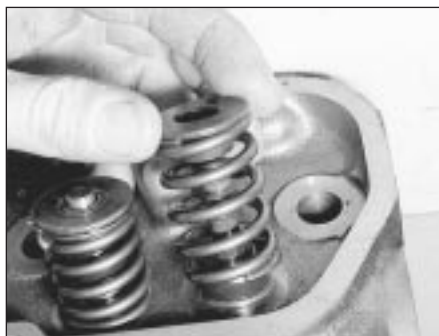
8.6A Remove the valve spring retainer and spring . . .
