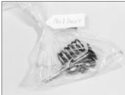
8.8 Use a labelled plastic bag to store and identify valve components
