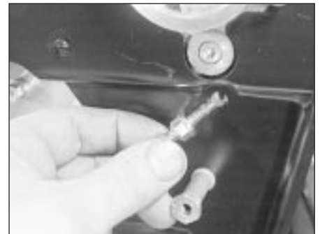
10.17A Fitting tensioner spring retaining pin
