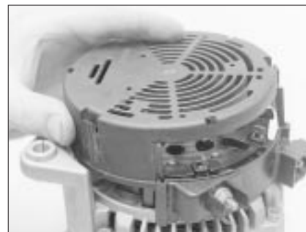
14.7 Remove the three screws, and withdraw the plastic end cover (Bosch NC alternator)
