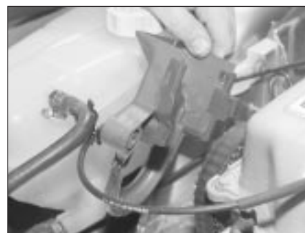
9.4 Lower timing belt cover removal
