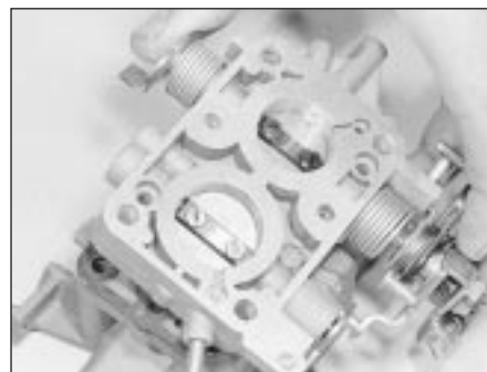
17.15 Separating the throttle housing from the carburettor main body
