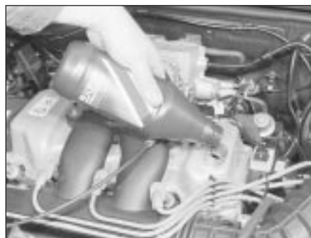
3.6B Topping-up the engine oil level (CVH engine)
