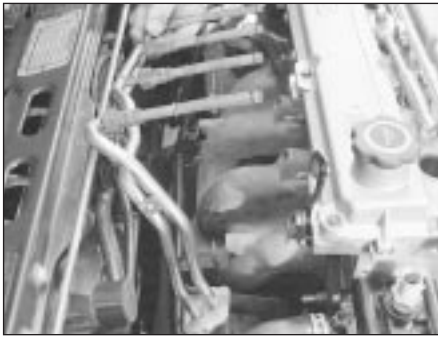
6.46 Removing the pulse-air piping on Zetec engines
