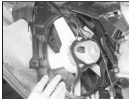
5.7 Withdrawing the cooling fan shroud and motor from under the vehicle
