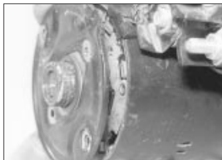
18.4 Remove the commutator endplate (Bosch starter motor)
