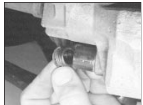
2.17A Prise free the blanking plugs from the caliper upper and lower mounting bolts
