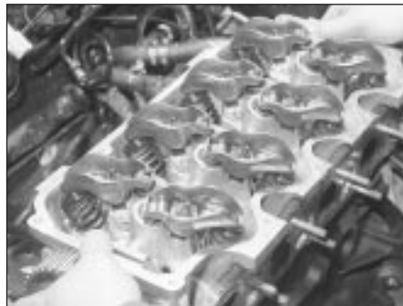
14.23A Lower the cylinder head into position
