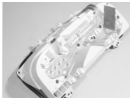
10.2 Rear face of the instrument panel showing bulbholder locations
