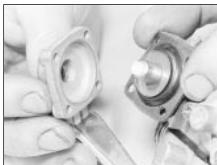
17.11A Remove the cover from the accelerator pump cover ...
