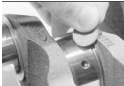
16.3 Rubbing a penny lengthwise along each journal will reveal its condition - if copper rubs off and is embedded in the crankshaft, the journals should be reground
