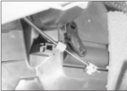
12.2 Heater temperature control cable connection on the right-hand side of the heater unit
