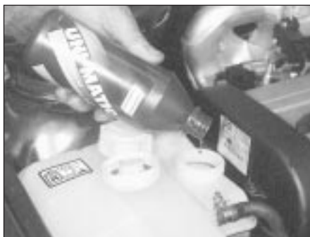
5.6 Topping-up the power steering fluid reservoir
