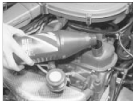
3.6A Topping-up the engine oil level (HCS engine)
