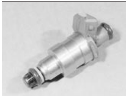
16.15 Fuel injector with new seals fitted
