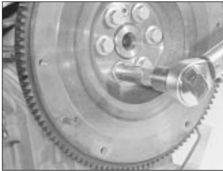
18.11 Note “peg” tool used to lock flywheel/driveplate while (new) bolts are tightened
