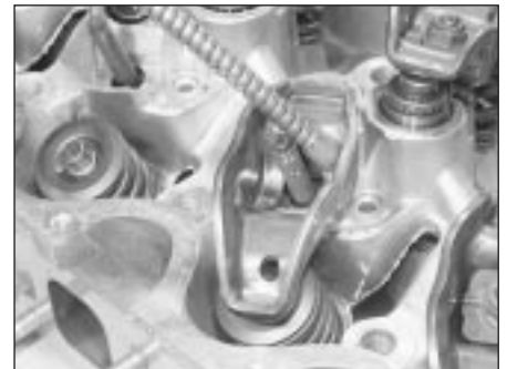
13.26 Lubricate the rocker arm assemblies as they are refitted
