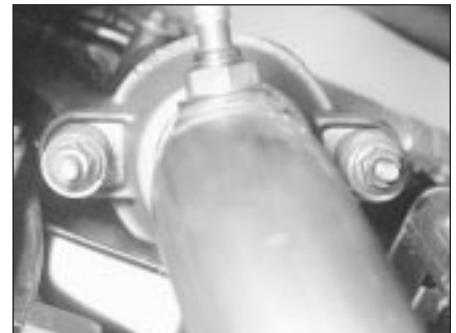
6.26 Disconnect the exhaust system front downpipe from the manifold
