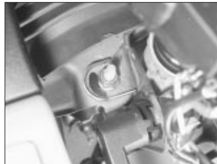
21.8 Steering column upper retaining nut (on the left-hand side of the column)
