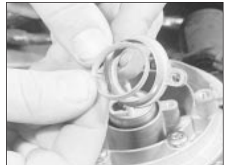
15.9E Withdrawing the seal from the injector retaining collar
