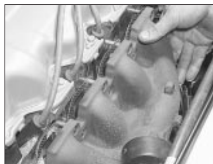
7.4 Removing the exhaust manifold
