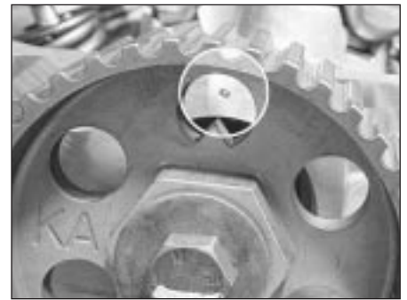
4.6B Camshaft sprocket timing mark aligned with the TDC mark on the front face of the cylinder head
