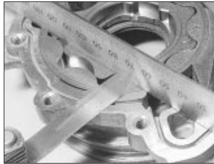
17.3C Rotor endfloat check
