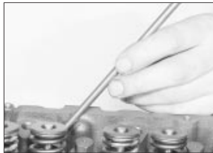
10.17 Withdraw the pushrods
