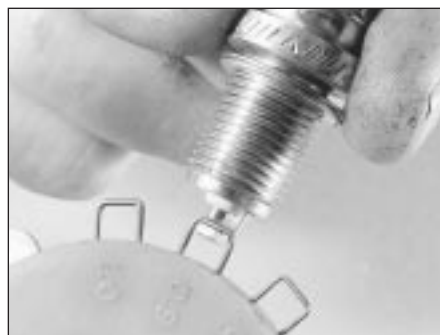
27.12B Spark plug manufacturers recommend using a wire-type gauge when checking the gap - if the wire or feeler gauge does not slide between the electrodes with a slight drag, adjustment is required
