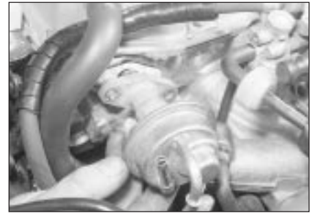
7.10 Fuel pump removal from the CVH engine
