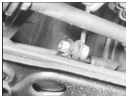
8.3 Link rod-to-bar connection
