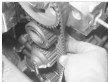
10.13 Checking the tension of the timing belt
