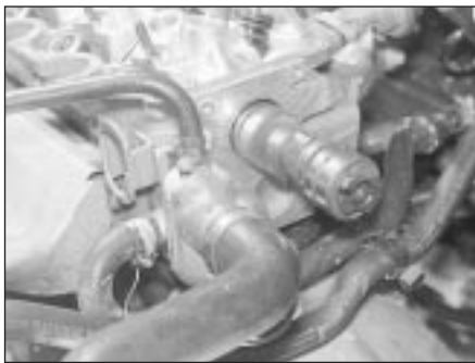
13.12 Withdraw the camshaft from the cylinder head
