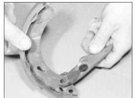
6.8 Disconnecting the strut from the leading brake shoe
