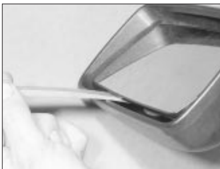
17.1A Prise free the door mirror glass...
