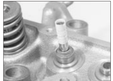
10.3A Tape the end of the valve stem before fitting the valve stem seal
