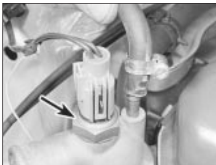
4.3A Detaching the expansion tank top hose from the thermostat housing on the HCS engine. Thermostatic switch is also shown (arrowed)
