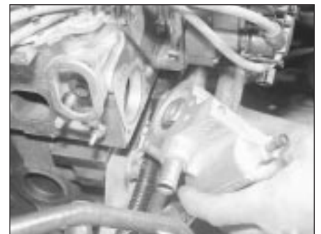
4.5 Removing the thermostat housing (CVH engine)
