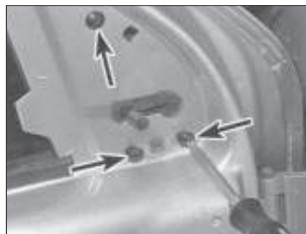
18.8 Removing the three mirror retaining screws (arrowed)
