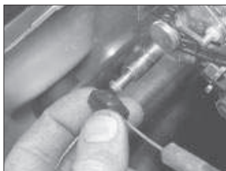
6.5a Disconnect the inner cable from the choke linkage
