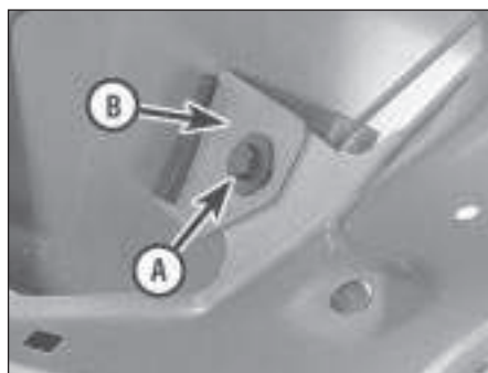
27.3 Tailgate lock retention arrangement
