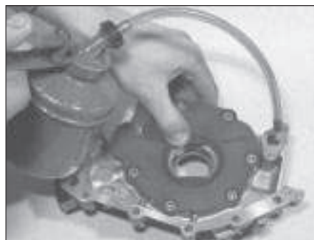
14.8 Prime the oil pump prior to fitting
