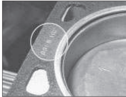
12.27 Fit the cylinder head gasket with the "OBEN/TOP" marking upwards . . .
