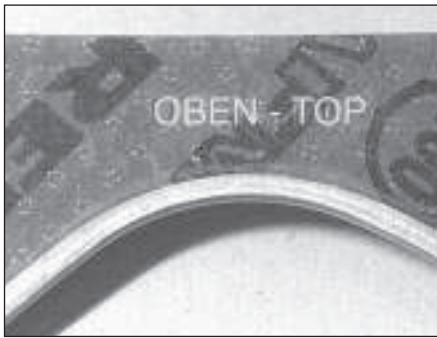
7.25 Cylinder head gasket top-face marking ("OBEN")
