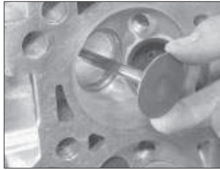
9.9 Insert the valve into its guide
