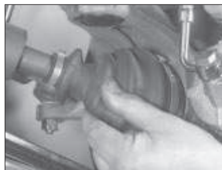
11.2 Check the driveshaft gaiters by hand for cracks and/or leaking grease
