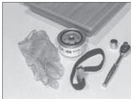
3.2 These tools are required when changing the engine oil and filter
