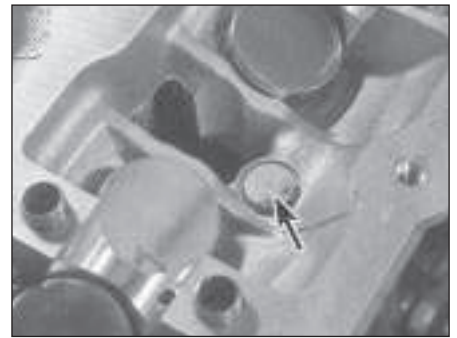
7.23 Cylinder head oil-retaining valve (arrowed)
