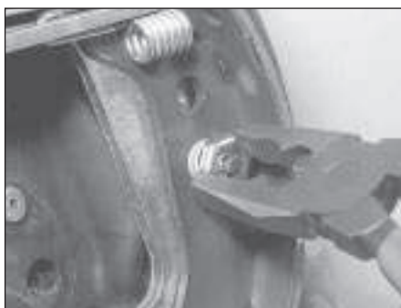
6.3 Depress and turn the cups securing the brake shoes
