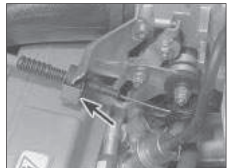
5.4 Detach the accelerator outer cable retaining clip (arrowed)
