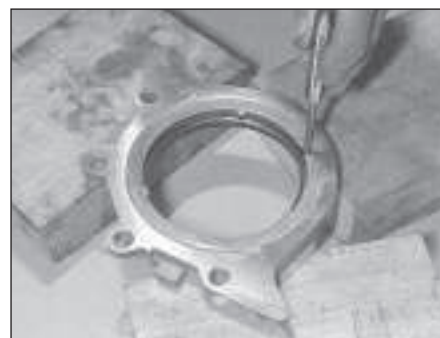
15.13 . . . and ensure that carrier is properly supported when driving out used oil seal - note notches provided in carrier for drift
