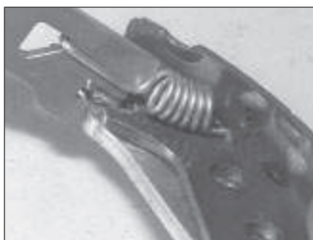
6.7b Detach the adjuster strut
