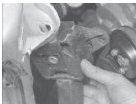
15.10 Undo the three bolts securing the mounting assembly to the cylinder block and withdraw the mounting
