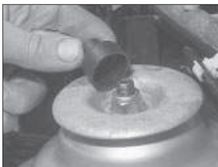
4.2a Removing cap from front suspension strut top-mount retaining nut
