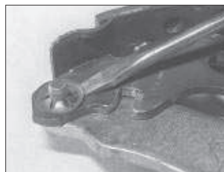
6.8 Lever off the spring clip securing the handbrake operating lever to the trailing shoe
