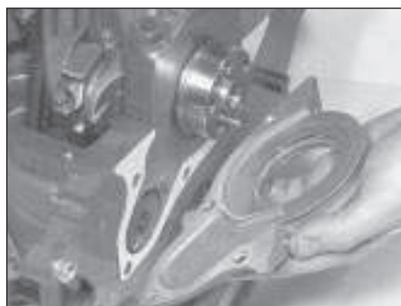
14.11b Fitting the rear oil seal housing with a new gasket in position on the rear face of the cylinder block
