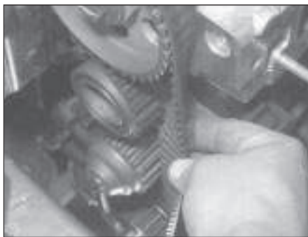
8.13 Checking the tension of the timing belt
