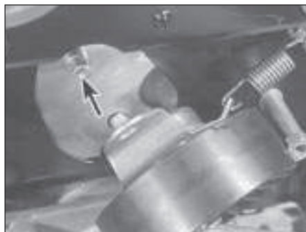
8.17b Hook spring onto tensioner and refit as shown - engage tensioner backplate on locating peg (arrowed) . . .
