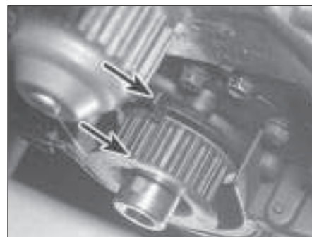
8.7 Sprocket and oil pump housing TDC marks in alignment
