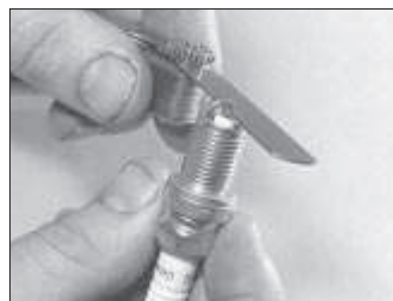
21.12a Measuring a spark plug gap with a feeler gauge
