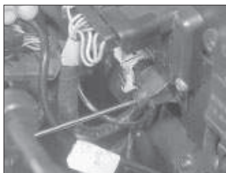
9.16 Adjusting the idle mixture CO content on the 1.6 litre EFi engine
