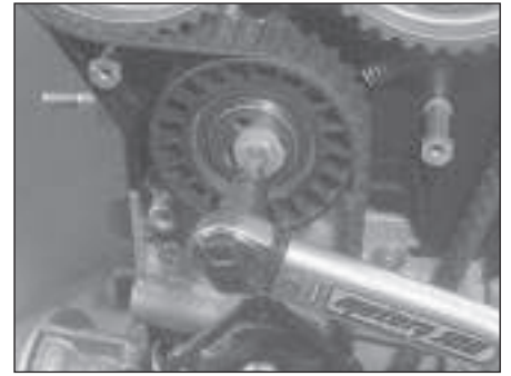
8.24 When setting is correct, tighten tensioner bolt to specified torque wrench setting
