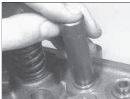
9.3b Press the seal into position using a suitable socket
