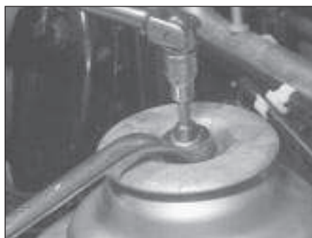
4.2b Slackening the front suspension strut top-mount retaining nut whilst preventing the piston rod from turning
