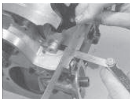
14.13 Oil pump must be positioned accurately
