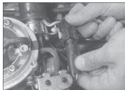
14.28b Disconnecting the throttle plate control motor multi-plug
