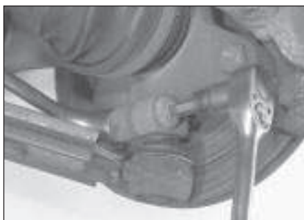
2.11a Remove the lower arm-to-spindle carrier pinch bolt and nut . . .
