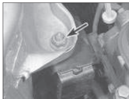
15.9 Unscrew and remove the mounting retaining nut and washer from the suspension strut cup retaining plate
