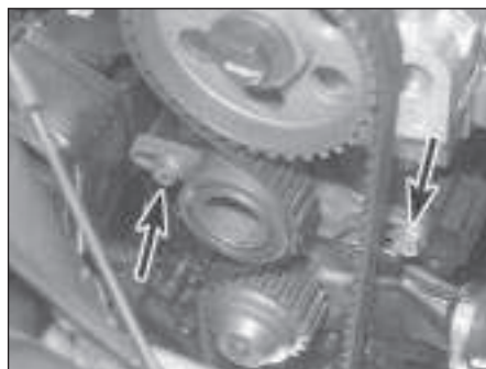
8.4 Timing belt tensioner retaining bolts (arrowed)
