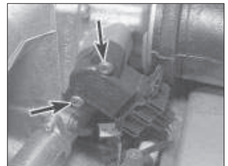
14.46 Throttle position sensor mounting screws (arrowed)
