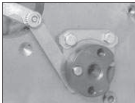
10.3 Checking the camshaft endfloat
