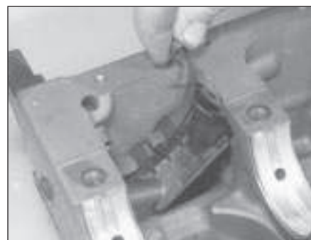
17.7 Fit the crankcase ventilation cap and its retaining spring
