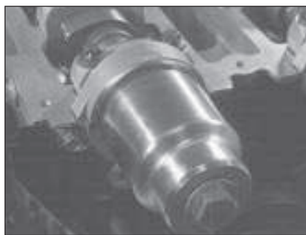
10.5 Using socket and toothed pulley bolt to install camshaft oil seal
