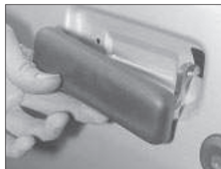
22.4b Removing the door exterior handle, guiding its operating rod out through the door skin (front door)
