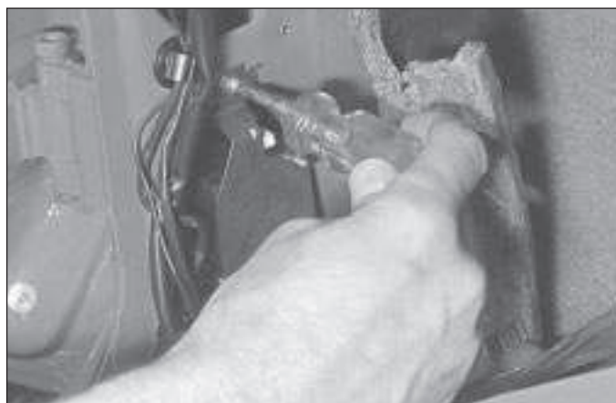
12.3a Remove the screw securing the inertia switch bracket . . .
