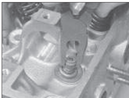
7.14 Prise off the valve stem oil seal
