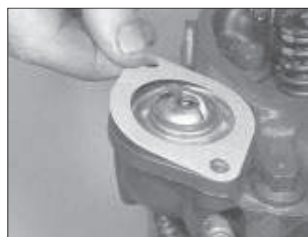
4.7a Removing the gasket and thermostat from an HCS engine
