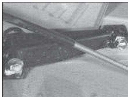
17.7 Courier rear suspension pivot brackets locate on dowels in underbody
