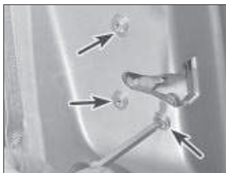
22.20 Removing the latch securing screws (arrowed)
