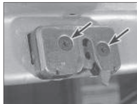
27.2 Tailgate latch and its Torx securing screws (arrowed)
