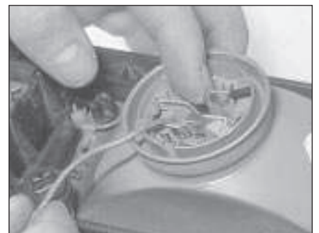
5.19 Releasing the auxiliary light bulb retainer (XR2i models)
