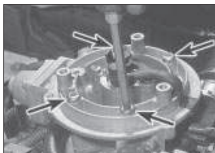
14.22 CFi unit securing screws (arrowed)
