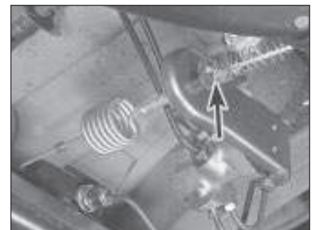
22.3 Light-laden valve linkage adjustment locknut (arrowed)
