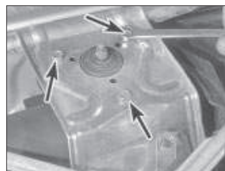
16.8a With the crank removed from the driving shaft taper, undo the three wiper motor retaining bolts (arrowed)
