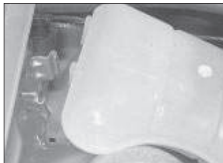
7.22b . . . and release the expansion tank from its retaining bracket
