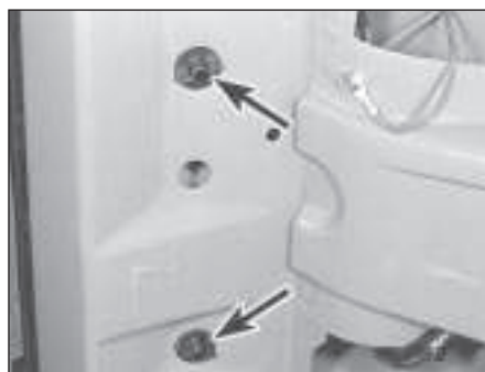
5.24a On Courier models, unscrew the two black plastic nuts securing the rear light cluster assembly . . .
