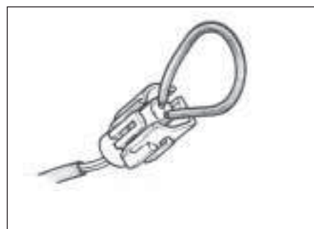
9.6 Cooling fan thermostatic switch multi-plug with temporary bridging wire connected
