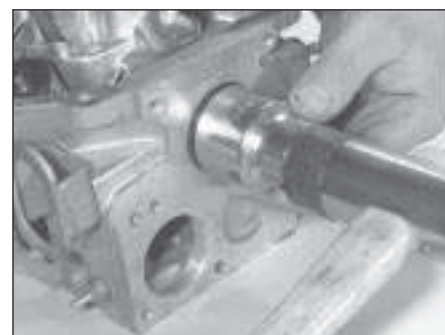
11.22 Driving a new blanking plug into position
