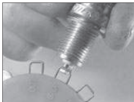
21.12b Spark plug manufacturers recommend using a wire-type gauge when checking the gap - if the wire or feeler gauge does not slide between the electrodes with a slight drag, adjustment is required
