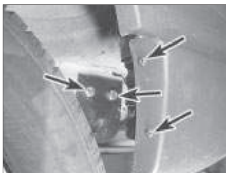
16.18 Courier rear bumper mounting screws (arrowed) at wheel arch - note also bumper mounting bracket bolts (arrowed) visible under rear of vehicle
