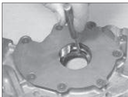
15.2 Driving out crankshaft right-hand oil seal
