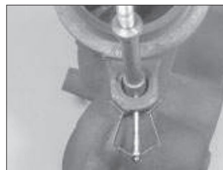
2.2e Release the spring clip to extract the securing bolt from the manifold, when required
