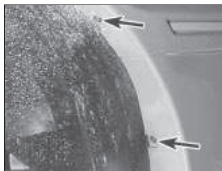
16.2 Front bumper-to-wheelarch retaining screws (arrowed)
