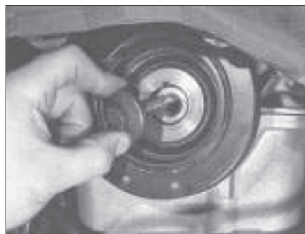
6.9 Unscrew pulley bolt to release crankshaft pulley
