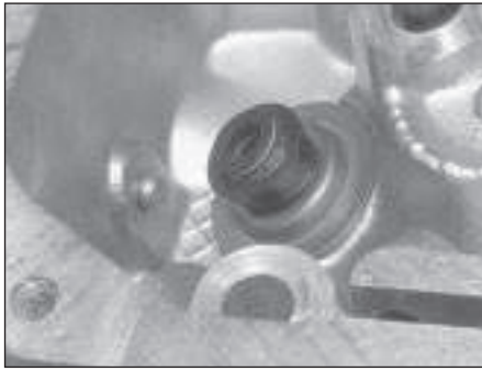
9.8 Locate the seal, and tap it into position over the guide
