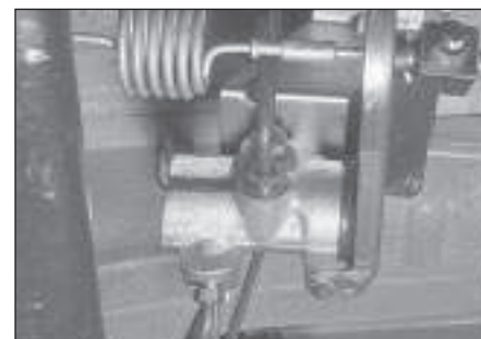
21.3 Hydraulic pipe and linkage attachments at the light-laden valve
