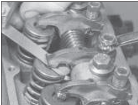
5.6 Adjusting the valve clearances
