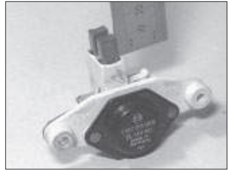
7.4 Measuring the brush lengths (Bosch alternator)
