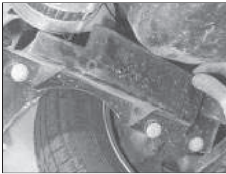
6.3 Removing the drivebelt splash guard (where fitted)
