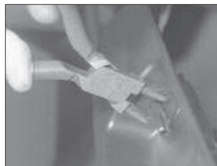
20.3 Removing the manual choke control assembly retaining collar
