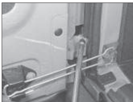
28.2 Unscrewing the bottom hinge's cap securing bolt on Courier rear door
