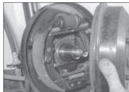
9.5 Slide off the wheel hub/brake drum unit
