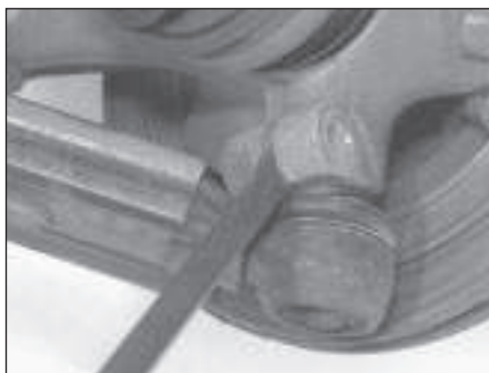
2.11b . . . prise open the joint . . .
