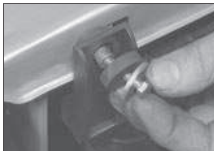
7.6a Radiator securing bolt, insulator and washer
