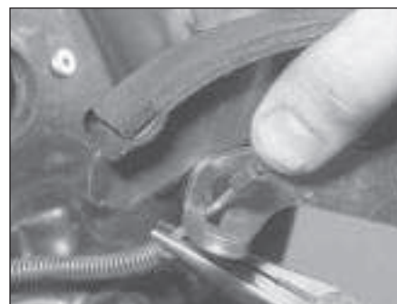
6.5 Disengage the handbrake cable from its operating lever on the trailing shoe
