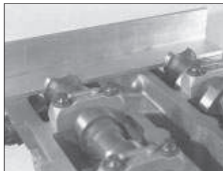
11.21b Fit camshaft-aligning tool to set TDC position while camshaft toothed pulleys are refitted
