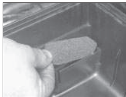
25.13 The crankcase ventilation system foam filter is located in the air cleaner housing on Zetec engines
