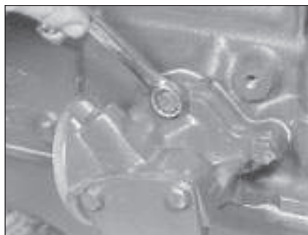
12.4 Unscrewing the oil pump retaining bolts
