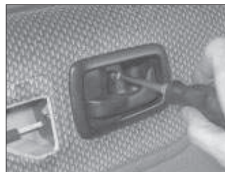
21.2 Removing the door interior release handle bezel (armrest/doorpull shown removed)
