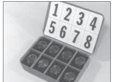
11.6b Store tappets in clearly-marked container filled with oil to prevent oil loss
