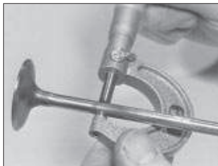
8.12 Measuring the diameter of a valve stem
