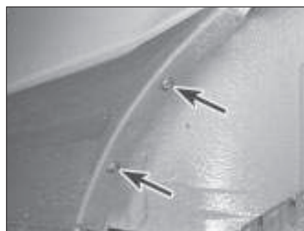
17.9a Courier rear quarter moulding mounting screws (arrowed) in wheel arch . . .
