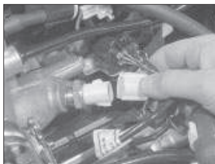
14.43 Disconnecting the intake air temperature sensor multi-plug
