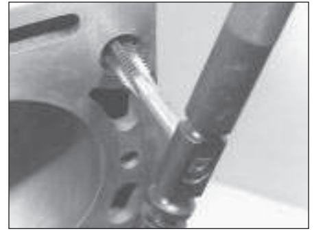
13.6 All bolt holes in the block should be cleaned and restored with a tap
