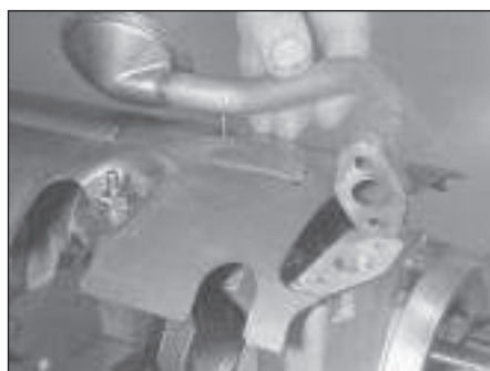
14.16 Use new gasket when refitting oil pick-up pipe to pump
