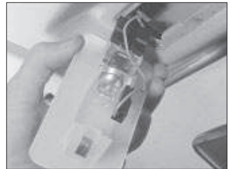
6.16b Interior (courtesy) light pivoted for access to the bulb
