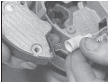
7.7b Disconnecting the field connector (Magneti-Marelli alternator)
