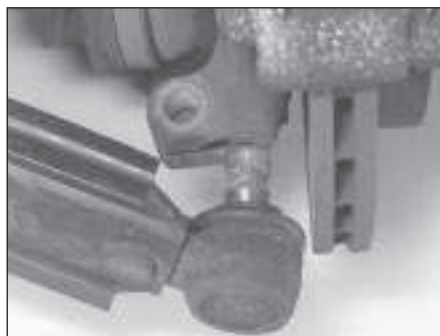
2.11c . . . and detach the lower arm balljoint from the spindle carrier
