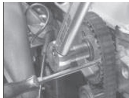
9.13b ... and tighten the retaining bolt to the specified torque whilst retaining the sprocket as shown
