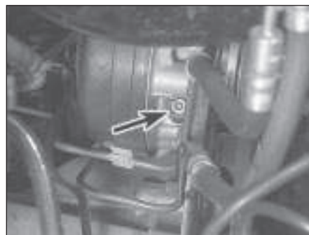
14.7 Modulator auto-bleed plunger (arrowed)
