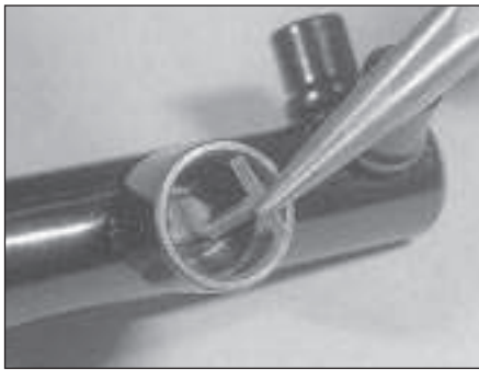
9.7 Removing the secondary piston retaining pin
