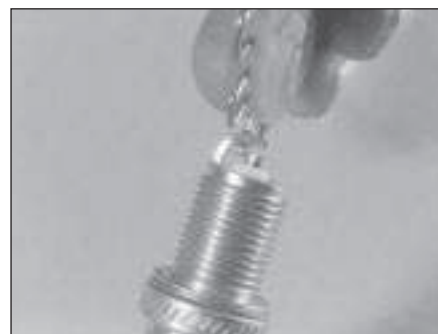
21.13 To change the gap, bend the outer electrode only, and be very careful not to crack or chip the porcelain insulator surrounding the centre electrode
