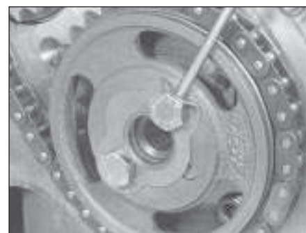
10.13 Bend locktabs against the camshaft retaining bolt heads to secure
