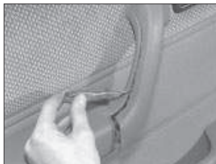
21.4a Detaching armrest/doorpull removable panel
