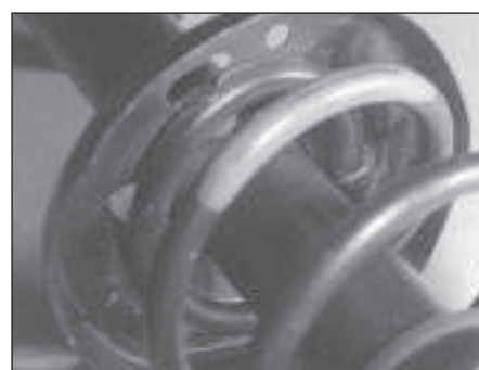
5.9 Correct spring location in its lower seat
