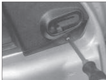
18.7 Removing the mirror trim retaining screw
