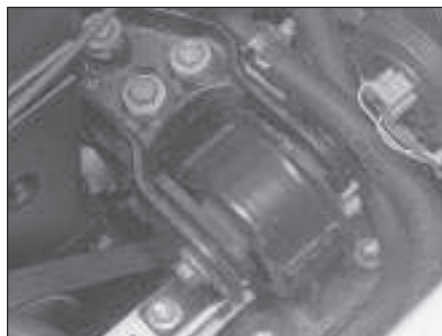
16.8 Engine front right-hand mounting
