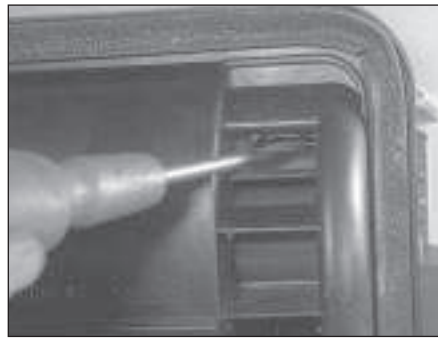
11.20a Releasing the heater fan motor retaining strap from the underside of the assembly
