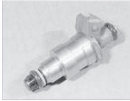
14.13 Remove the seals from the injectors
