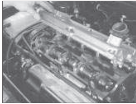
4.8 Removing cylinder head cover
