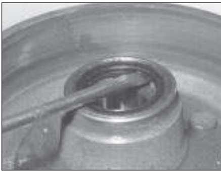
9.6 Prise the grease retainer from the hub bore
