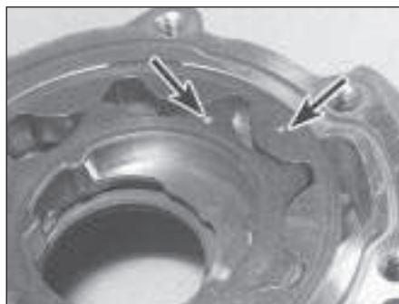
15.4 Inner and outer rotor matchmarks (arrowed)
