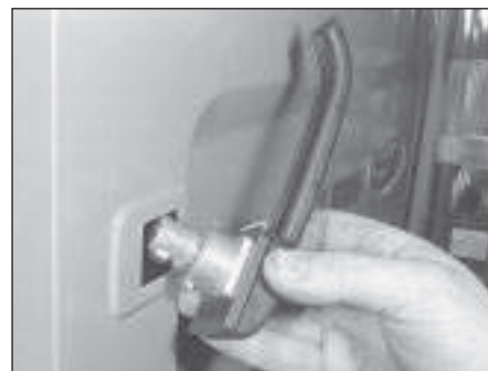
30.7b . . . to release Courier rear door exterior handle
