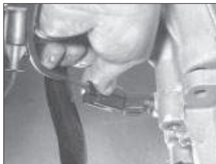
5.14c . . . and the reversing light switch
