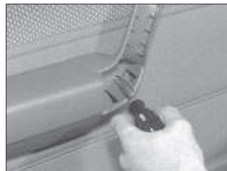
21.4b Undoing armrest/doorpull retaining screws
