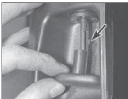
20.2 Manual choke control knob and its locating lug (arrowed)
