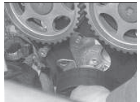
9.3 Removing timing belt tensioner
