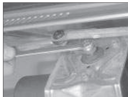
16.7 Unscrew the nut from the wiper motor driving shaft
