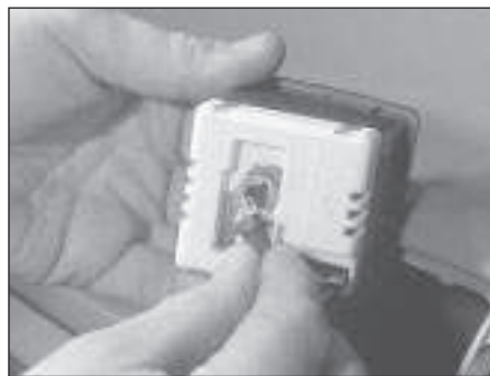
6.8 Withdrawing the clock illumination bulb and its integral holder from the rear of the clock
