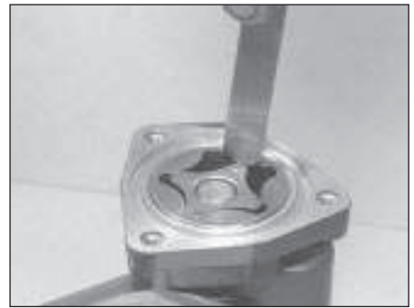
13.4b Checking the inner rotor-to-outer rotor clearance
