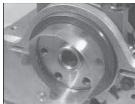
15.18 Using guide made from thin sheet of plastic to slide oil seal lips over crankshaft shoulder
