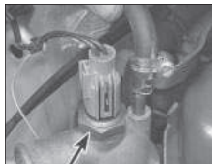
4.4b Disconnecting the expansion tank top hose from the thermostat housing (HCS engine). Radiator cooling fan thermal switch (arrowed)
