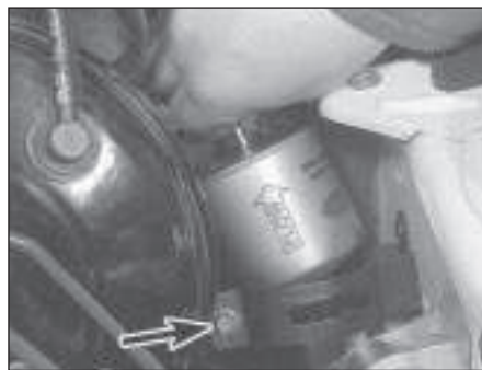
30.6b Removing the bulkhead mounted fuel filter. Clamp bolt (arrowed)
