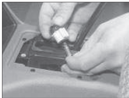
6.3a Remove the selector illumination bulb cover . . .
