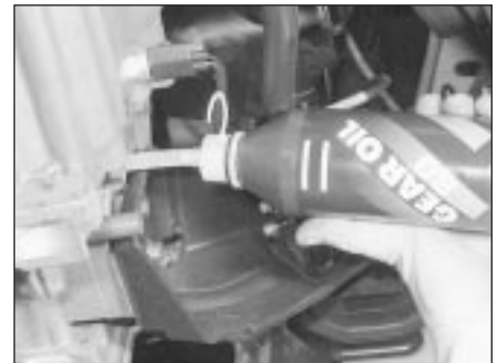
18.2 Topping-up the oil level in the BC type transmission
