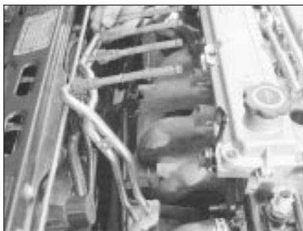
6.46 Removing the pulse-air piping on Zetec engines
