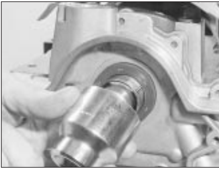
17.5 Socket of correct size can be used to replace Ford service tool, drawing new seal into place as described
