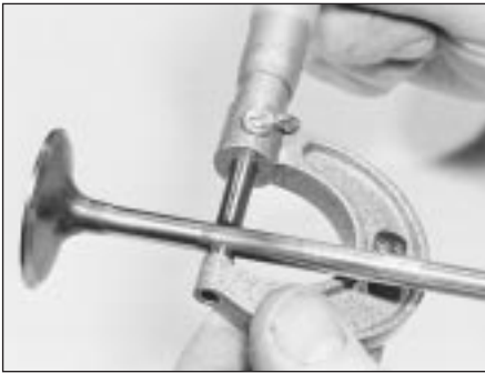
9.12 Measuring the diameter of a valve stem - if any significant difference is found in the readings obtained, excessive valve stem wear is indicated
