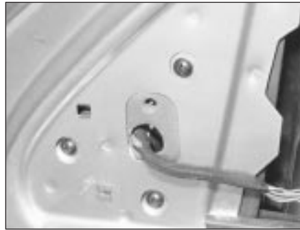
17.5 Undo the three mirror retaining screws
