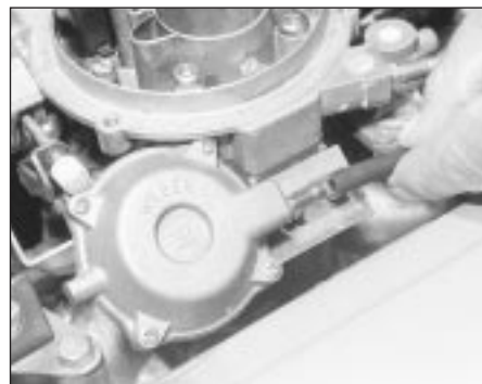
23.7 Disconnecting the vacuum hose from the secondary venturi diaphragm unit
