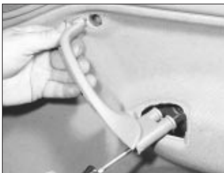
10.2B ... and undo the handle retaining screws
