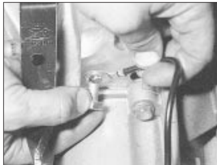
6.12 Unbolt the engine/transmission-to-body earth lead from the transmission
