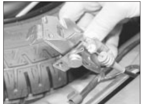
23.6B . . . withdraw the tailgate striker plate and detach the release cable
