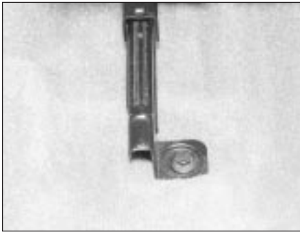
32.1A Front seat/runner rear outboard retaining bolt
