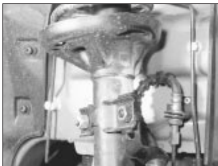
2.3 Disconnect the brake hose from the front suspension strut
