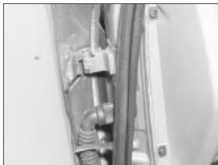
35.8A Pull free the weatherstrip for access to the outboard fascia screws
