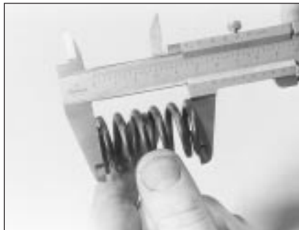
9.18 Checking the valve spring free length
