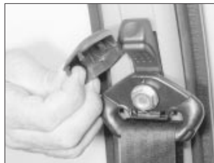
33.7 Remove the cover for access to the seat belt upper anchor bolt
