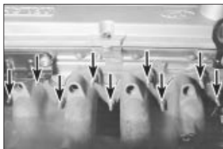
7.8A Unscrew nuts (arrowed) to remove exhaust manifold . . .
