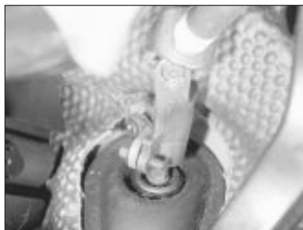
21.7 Steering column-to-pinion shaft coupling and clamp bolt
