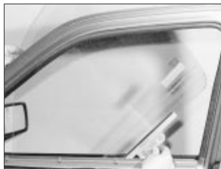
11.4 Removing a door window glass
