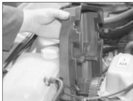
9.2 Upper timing belt cover removal
