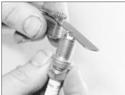
27.12A Measuring a spark plug gap with a feeler gauge
