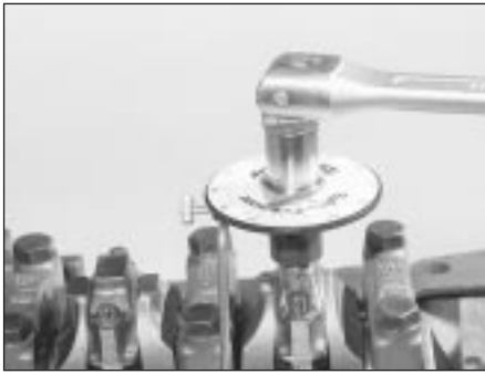
21.11A Angle-tightening the big-end bolts using the correct tool . . .
