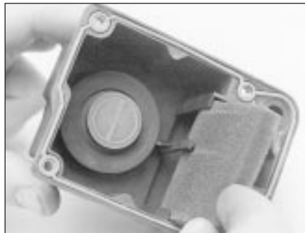
6.30B ... and withdraw the foam filter for cleaning, if required
