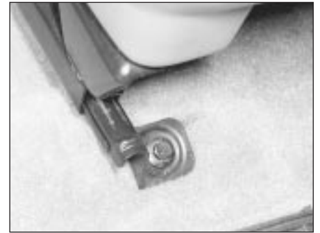
32.2 Front seat/runner forward mounting bolt
