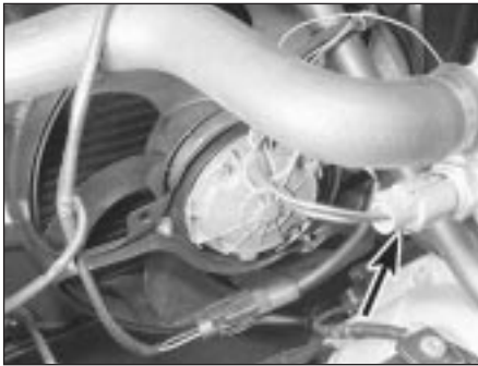
5.2A Cooling fan thermostatic switch location (arrowed) in the thermostat housing (CVH engine)
