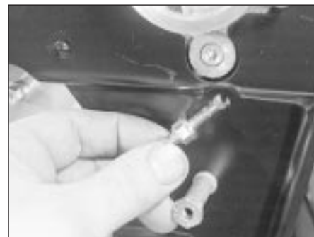
10.17A Fitting tensioner spring retaining pin
