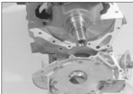
16.12 Use new gasket when refitting oil pump
