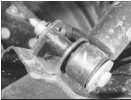
16.3 Rear shock absorber-to-axle mounting (Estate models)
