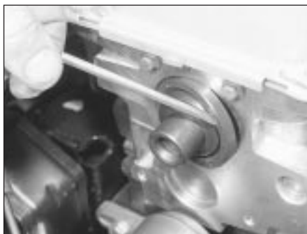
12.2 Camshaft front oil seal removal
