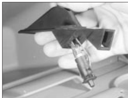
6.17 Glovebox light switch/bulbholder removal
