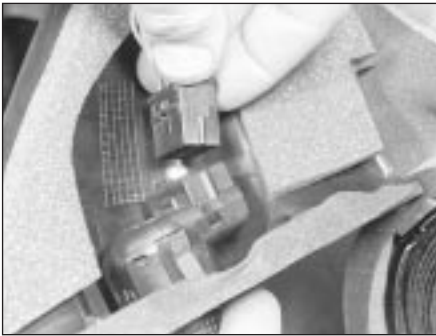
17.4 Detach the wiring multi-plug from the mirror control unit
