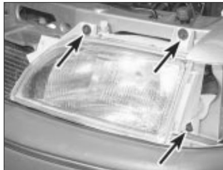
7.5 Headlight unit retaining screws (arrowed)
