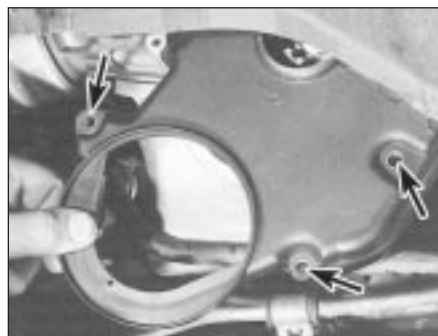
9.12 Removing timing belt lower cover - bolt locations arrowed
