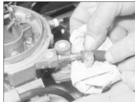
23.6 Disconnecting the fuel line at the carburettor
