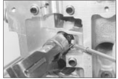
8.19C . . . so that both valve split collets can be removed from the valve's stem - small magnetic pick-up tool prevents loss of small metal components on removal and refitting
