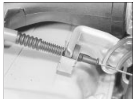
5.6 Accelerator outer cable location at the adjuster/support bracket
