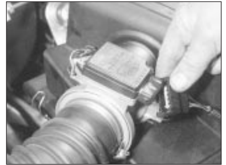
4.38 Disconnecting the air mass meter electrical connector
