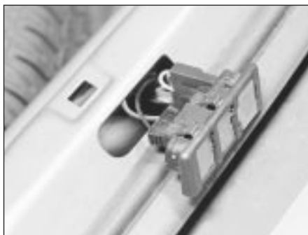
4.22 Luggage area contact switch removal from the rear panel
