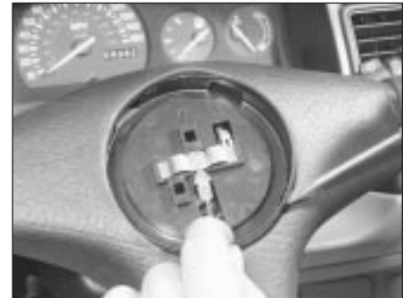
20.4 Prise free the inner horn pad and detach the wires . . .
