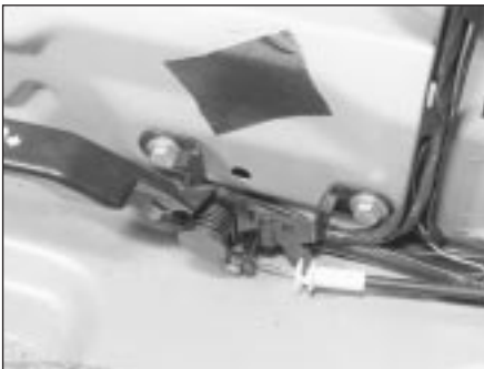
23.9 Tailgate release handle and operating cable
