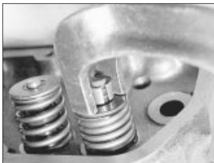
8.5 Compress the valve spring to remove the collets
