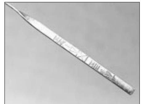
3.4 Engine oil dipstick MAXimum and MINimum level markings
