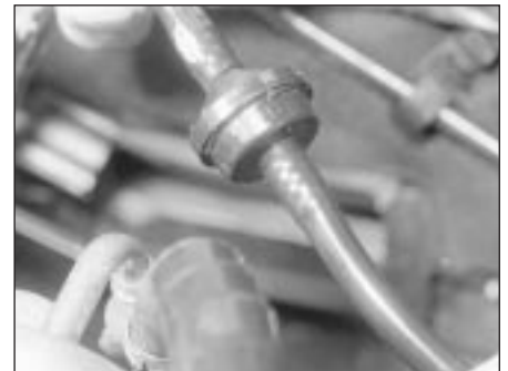
19.5 Non-return valve in the servo vacuum hose
