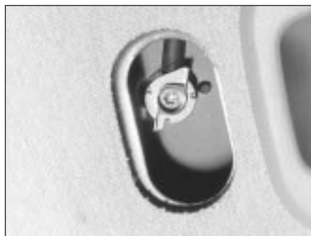
23.2 Roof-mounted aerial retaining screw
