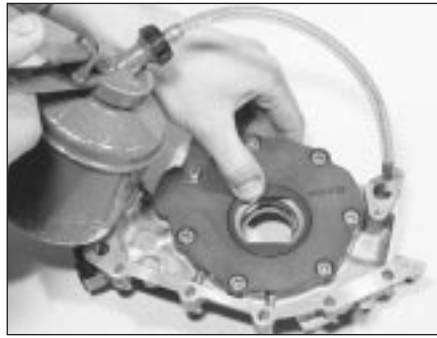
16.8 Prime the oil pump prior to fitting
