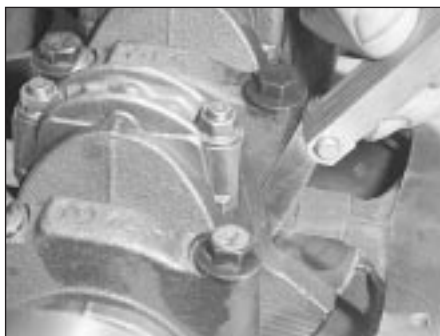
13.3 Checking crankshaft endfloat with a feeler gauge
