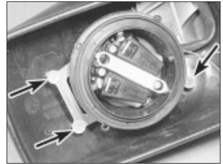
17.6 Mirror motor and retaining screws (arrowed)
