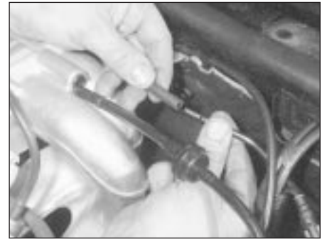
6.10 Disconnecting the vacuum hoses from the inlet manifold
