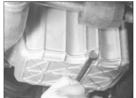
16.7B Removing the engine oil drain plug on the Zetec engine
