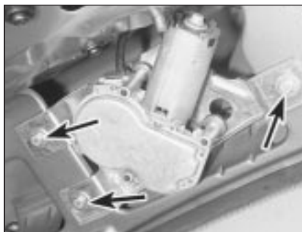
18.7A Tailgate wiper motor and mounting bolts (arrowed) on Hatchback models
