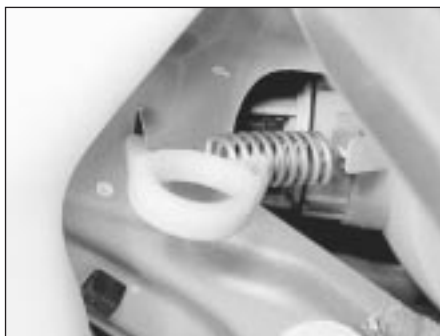
5.14 Front indicator unit retaining spring
