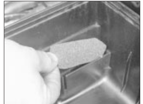
30.8 The PCV system foam filter is located in the rear right-hand corner of the air cleaner housing on Zetec engines
