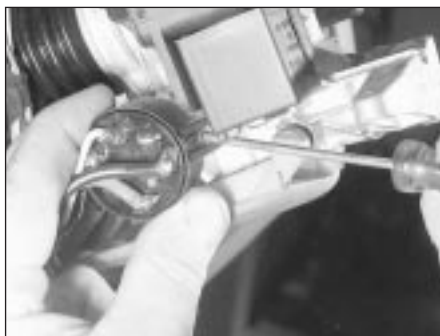
4.3A Depress the lock tabs . . .
