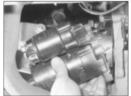
17.5B Starter motor removal (CVH engine shown)
