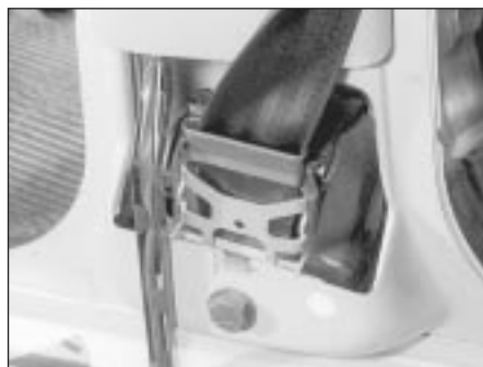
33.11 Inertia reel unit and retaining bolt
