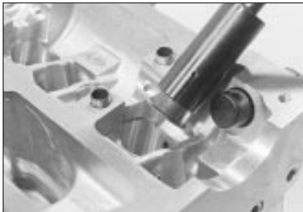
8.22A Ford service tool in use to remove valve spring lower seat/stem oil seals . . .
