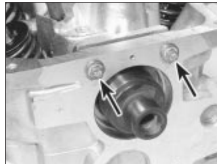
13.10A Undo the two retaining bolts (arrowed) ...
