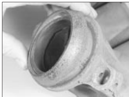
7.12B Renew exhaust system downpipe-to-manifold gasket to prevent leaks
