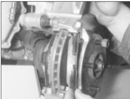
2.5 Withdraw the inner and outer brake pads from the anchor bracket
