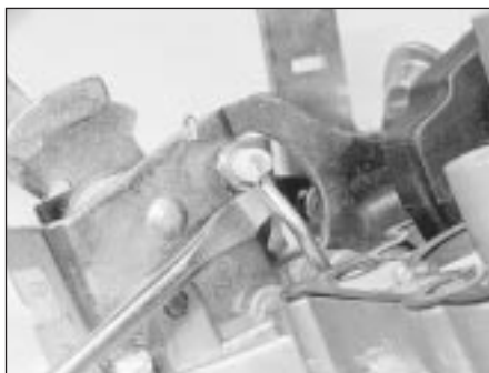
17.5A Detach the choke plate operating link ...
