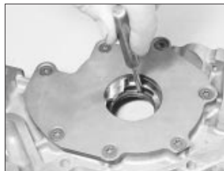
17.2 Driving out crankshaft right-hand oil seal
