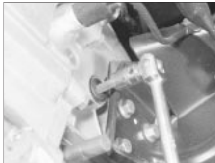
18.1 Unscrewing the manual transmission oil filler/level plug
