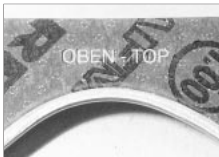
10.22A Cylinder head gasket top-face marking ("OBEN")
