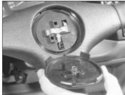
20.3 Remove the outer horn pad from the centre of the steering wheel
