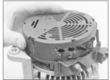
14.7 Remove the three screws, and withdraw the plastic end cover (Bosch NC alternator)
