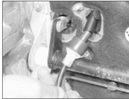
11.4 Withdrawing the speedometer cable through the bulkhead
