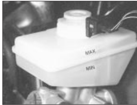
3.19 Brake master cylinder showing "MAX" and "MIN" marks
