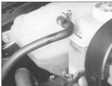
3.10 Coolant reservoir MAXimum and MINimum level marks
