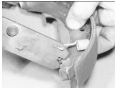
6.7B Disconnecting the support spring from the strut
