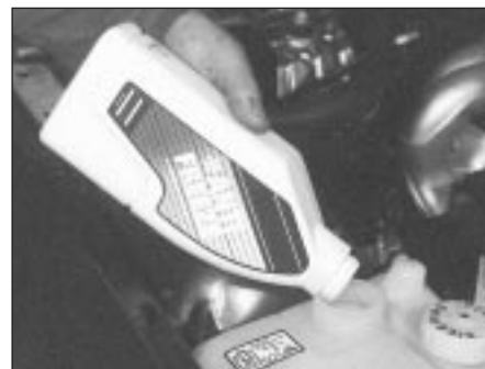
3.13 Topping-up the coolant level with specified antifreeze mixture
