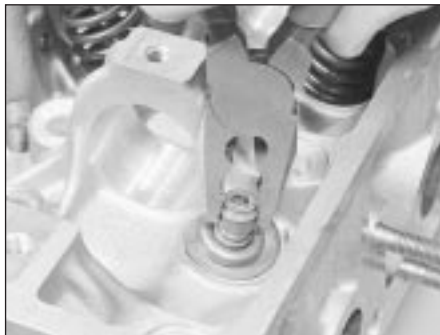
8.7 Prise off the valve stem oil seal
