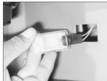
6.4 Luggage area light removed for bulb replacement
