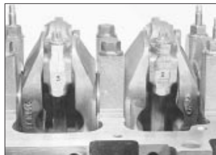
12.11 Each connecting rod and big-end bearing cap will have a flat-machined surface visible from the front (exhaust) side of the engine, with the cylinder number etched in it
