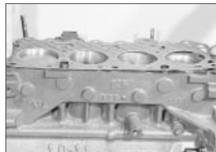
10.22B Cylinder head gasket in position on the top face of the cylinder block
