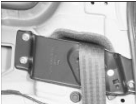
33.48 Rear seat backrest catch mounting (Estate models)
