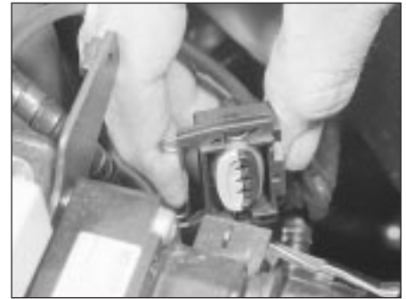
6.7 Disconnecting the multi-plug from the ignition coil
