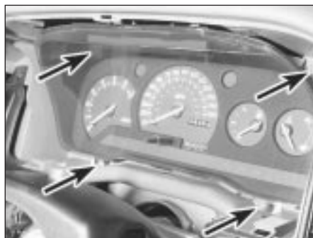
9.4A Instrument cluster retaining screws
