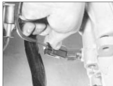
6.15C ... and the reversing light switch
