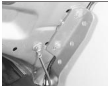
7.4 Bonnet hinge and earth lead connection
