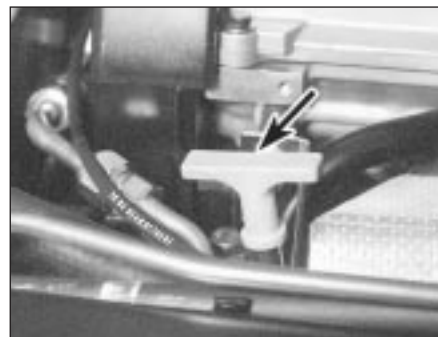
3.2 Engine oil dipstick location (arrowed) on Zetec engines
