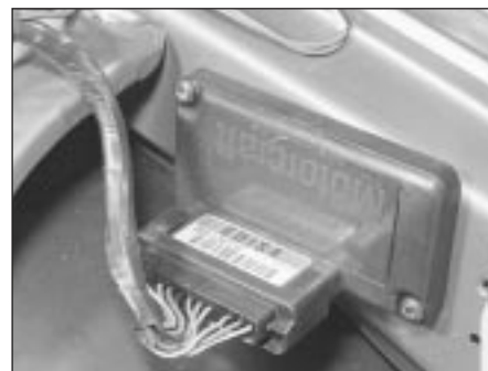
8.3 Ignition module and wiring connection on the 1.6 litre EFi fuel-injected engine
