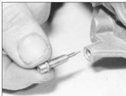
17.14 Unscrew and remove the fuel mixture screw
