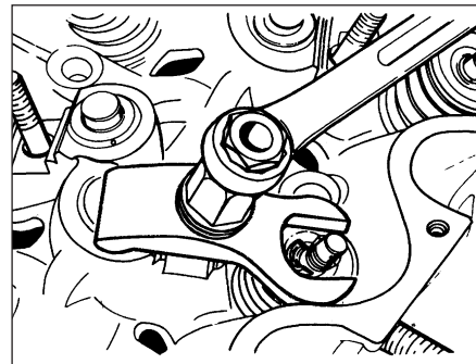
8.11 Compressing a valve spring using a forked type compressor
