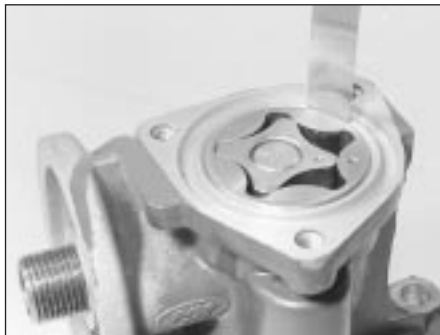
16.4A Checking the outer body-to-rotor clearance
