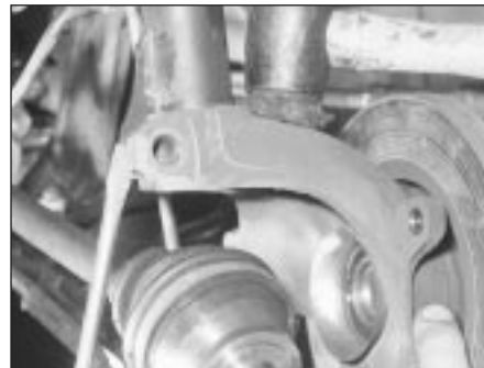
2.9B . . . and separate the spindle carrier from the strut
