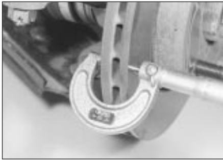
4.3 Checking the brake disc thickness using a micrometer
