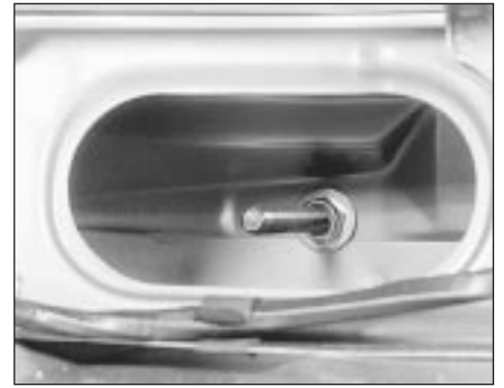
6.10B Rear (upper) bumper retaining nut (Estate models)
