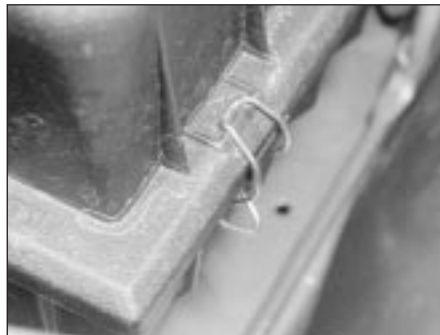
29.1E . . . and release the clips . . .
