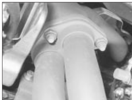
5.19 Exhaust downpipe-to-manifold flange and securing bolts
