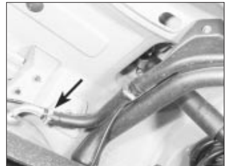
8.6 Fuel tank sensing hose-to-pipe connection (arrowed)
