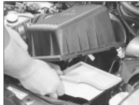
29.1F . . . then lift off the cover and withdraw the element
