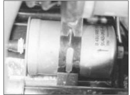
35.7 Fuel filter as fitted to 1.6 litre EFI engines showing direction of flow arrow
