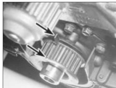
10.7 Sprocket and oil pump housing TDC marks in alignment
