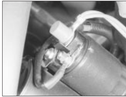
17.4B Starter motor and wiring connections on a CVH engine
