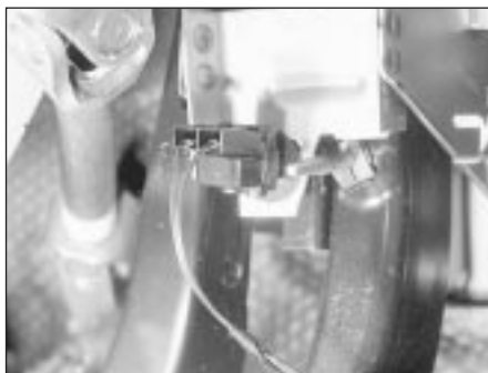
4.34 Brake stop-light switch location
