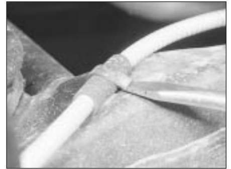
23.6B Release the handbrake cable from its locating clips
