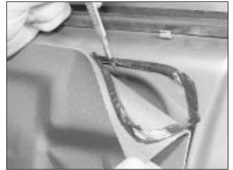
10.6B Cut through the adhesive to remove the door insulation sheet
