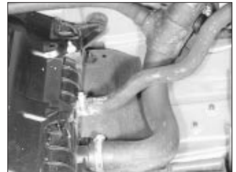
7.6B . . . the bottom hose and expansion tank hose from the radiator
