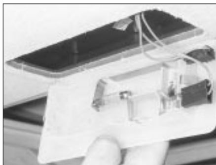
6.1 Roof-mounted courtesy light removal
