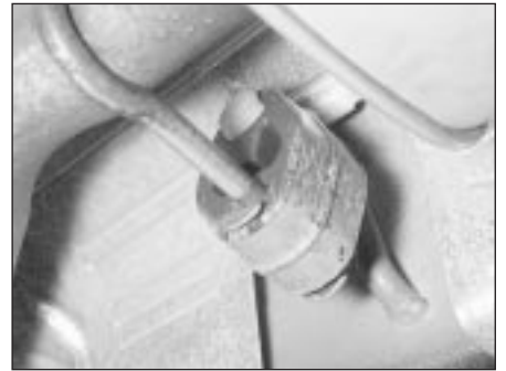
21.2 If any of the exhaust system rubber mountings are to be renewed, ensure that the replacements are of the correct type - their colour is a good guide. Those nearest to the catalytic converter are more heat-resistant than the others
