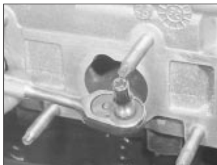
7.8B . . . studs can be unscrewed also, if required, to provide additional working space
