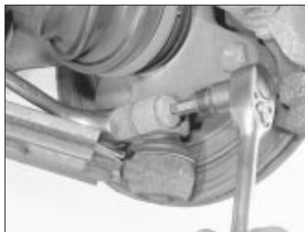
2.6A Removing the lower arm-to-spindle clamp bolt and nut
