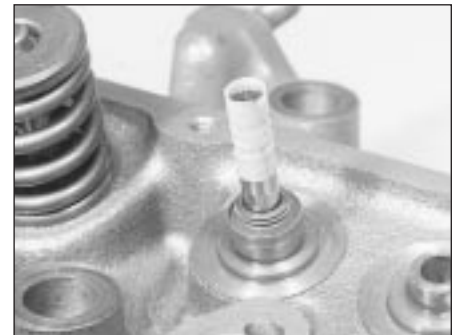
10.3A Tape the end of the valve stem before fitting the valve stem seal
