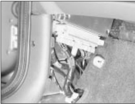
4.35 ECU location behind the side cowl kick panel in the passenger's footwell
