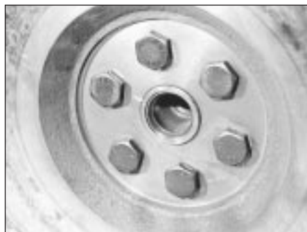
20.2 Flywheel retaining bolts
