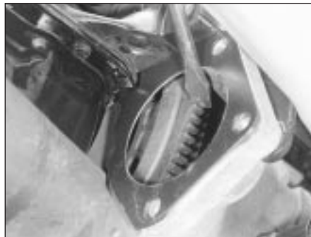
8.6 Using a suitable bar to lock the flywheel ring gear
