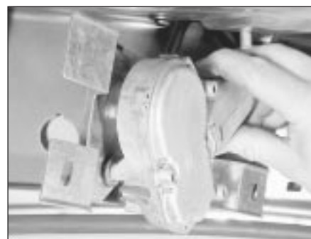
18.7C Removing the wiper motor from the tailgate (Hatchback models)
