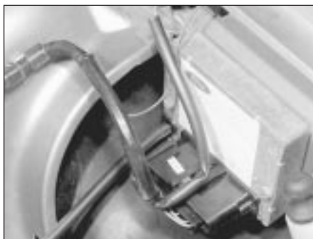
7.3 Ignition module showing vacuum hose and multi-plug arrangement (CVH carburettor engine shown)
