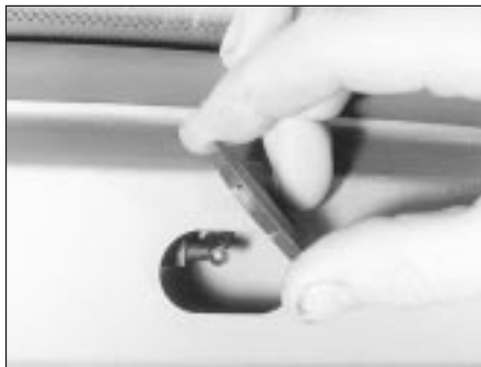
19.9 Remove trim for access to the tailgate washer nozzle
