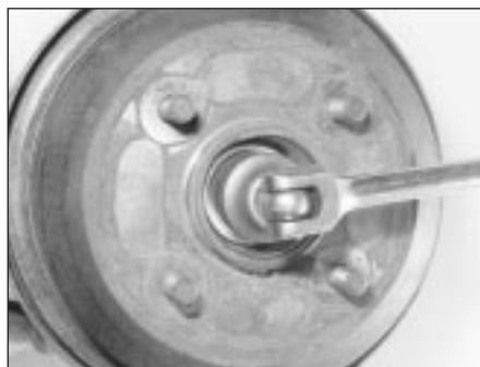
11.8 . . . unscrew the hub nut . . .
