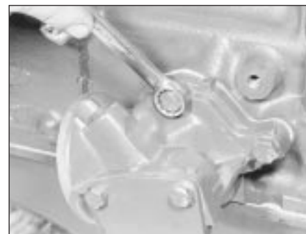
15.4 Unscrewing the oil pump retaining bolts
