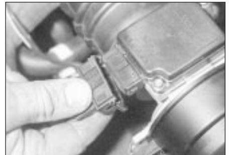
4.14 Disconnect the air mass meter wiring multi-plug, then release the two clips and withdraw the air mass meter, complete with inlet hose
