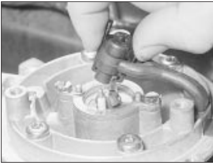
15.8 Disconnect the multi-plug from the injector
