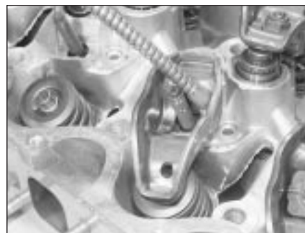
13.26 Lubricate the rocker arm assemblies as they are refitted
