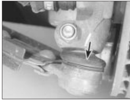
19.2B Check the condition of the lower arm balljoint dust cover (arrowed)
