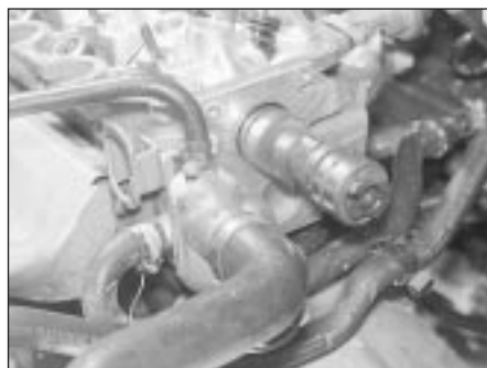
13.12 Withdraw the camshaft from the cylinder head
