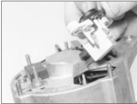
14.3C ... withdraw the brush box/regulator unit (Bosch K1 alternator)
