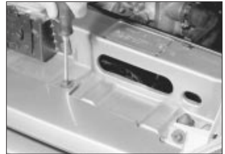
38.1 Radiator (front) grille panel retaining screw removal - pre-1993 models
