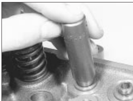
10.3B Press the seal into position using a suitable socket
