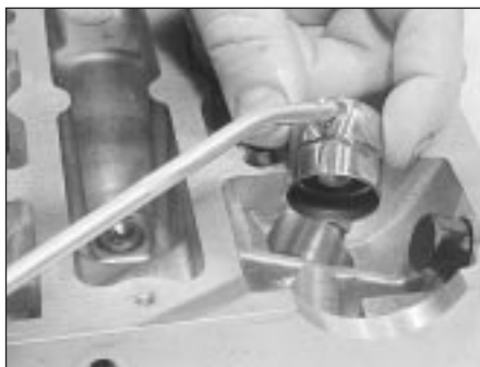
13.17 Oil liberally when refitting hydraulic tappets
