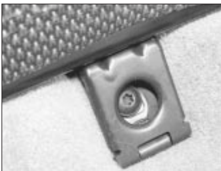
32.3 Rear seat cushion retaining screw (Saloon)
