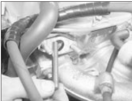
7.11 Withdrawing the fuel pump pushrod from the CVH engine
