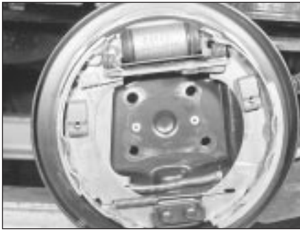
6.2 General view of the rear brake assembly with the drum removed
