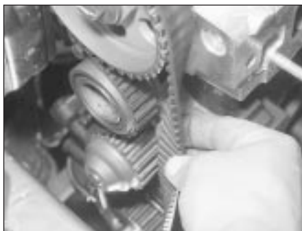
10.13 Checking the tension of the timing belt
