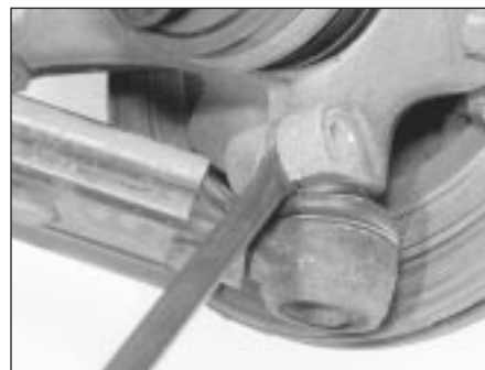
2.6B Prise open the joint . . .
