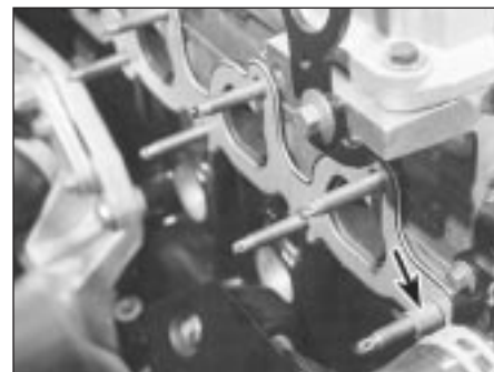
7.14 Fit plastic guide sleeve to stud (arrowed) when refitting exhaust manifold
