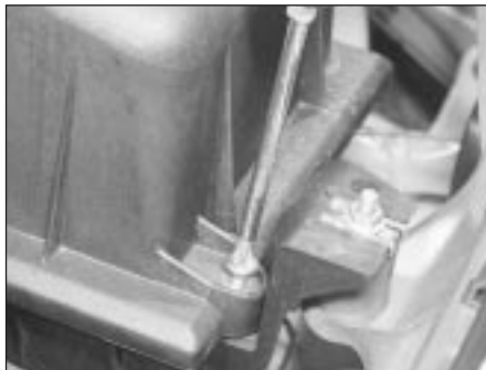
29.1D On EFI and SEFI engines, undo the air cleaner cover retaining screws . . .
