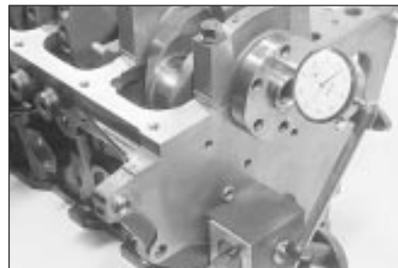
13.1 Checking crankshaft endfloat with a dial gauge
