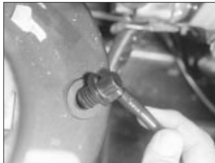
19.2 Detaching the vacuum hose from the servo unit
