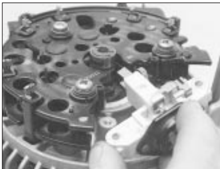
14.9 Remove the regulator/brush holder from the end frame (Bosch NC alternator)
