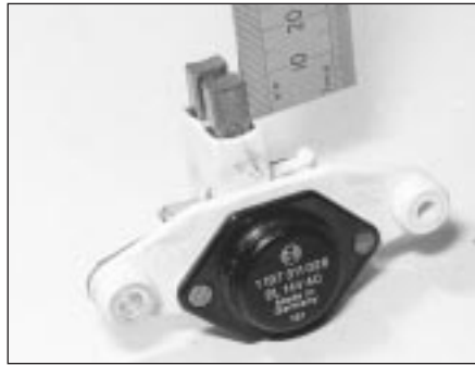
14.4 Measuring the brush lengths (Bosch K1 alternator)
