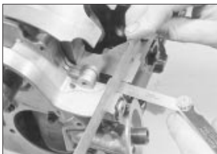
16.13 Oil pump must be centred on crankshaft, and square to cylinder block/crankcase-to-ump mating surface - use straight edge and feeler gauges to check that pump surface is an equal amount (within permissible limits) below crankcase surface on both sides of crankshaft
