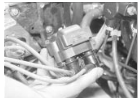
6.10B Removing the ignition coil from the CVH engine (leaving the HT leads attached)
