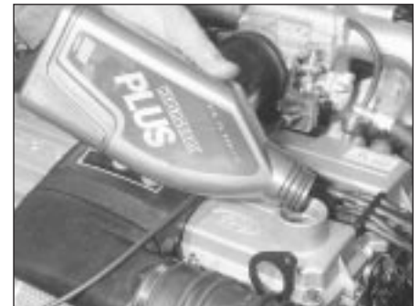
3.6C Topping-up the engine oil level (Zetec engine)
