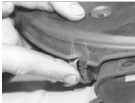
29.1B . . . and release the clips . . .
