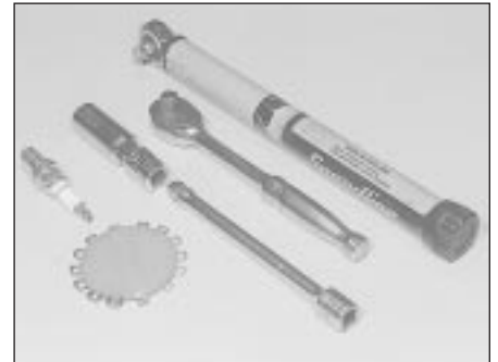
27.2 Tools required for changing spark plugs
