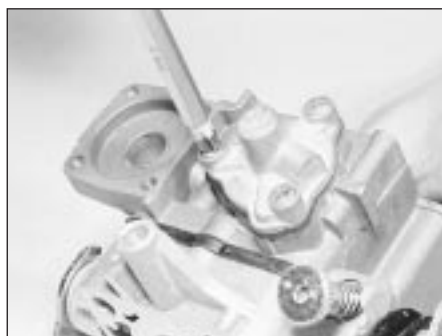
17.12A Undo the power valve assembly securing screws ...
