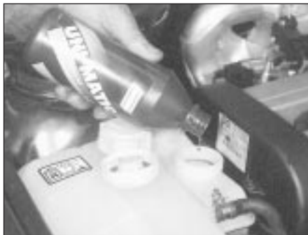
5.6 Topping-up the power steering fluid reservoir
