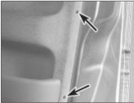
10.4 Door trim retaining screws (arrowed)
