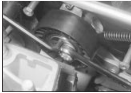
10.18 . . . then use Allen key to position tensioner so that timing belt can be refitted
