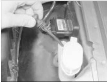
3.17 Checking the level of fluid in the washer reservoir
