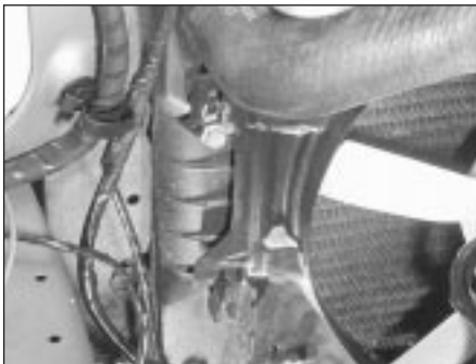
5.6 Cooling fan shroud-to-radiator retaining nut
