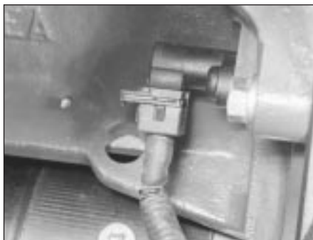
4.11B Engine crankshaft speed/position sensor and multi-plug
