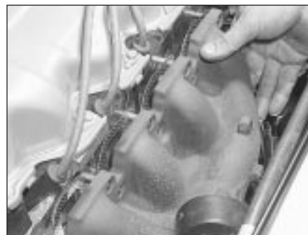
7.4 Removing the exhaust manifold
