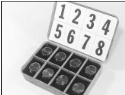
13.6B Store tappets in clearly-marked container filled with oil to prevent oil loss
