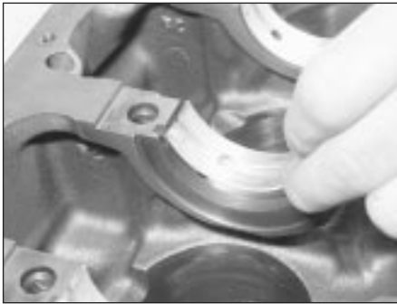
20.6 Fit the bearing shells to the main bearing housings in the crankcase
