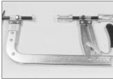
8.19B . . . or purpose-built special version, is required to compress valve springs without damaging cylinder head . . .
