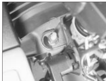
21.8 Steering column upper retaining nut (on the left-hand side of the column)
