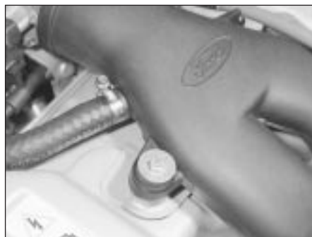
5.3 Air inlet duct-to-rocker cover attachment bolt on 1.6 litre EFi fuel-injected engine
