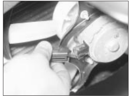
5.5A Detach the cooling fan motor wiring connector . . .
