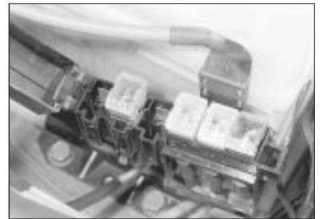
3.4 Additional "main" fuses at the front of the battery
