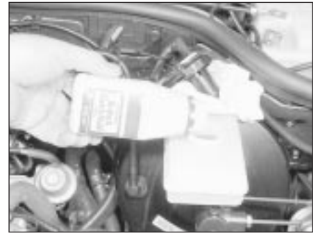
3.22 Topping-up the fluid level in the brake master cylinder reservoir
