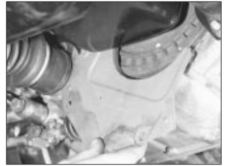
15.7 Removing the clutch cover plate
