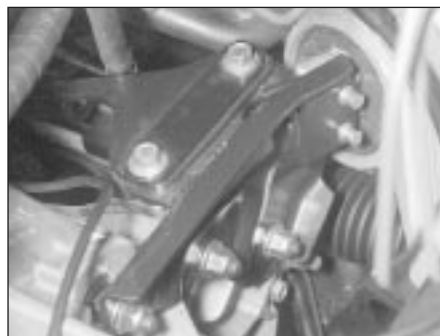
19.12 Engine/transmission left-hand rear mounting and mounting bracket attachments
