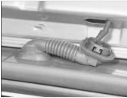
21.4 Detach the wiring connector from the tailgate
