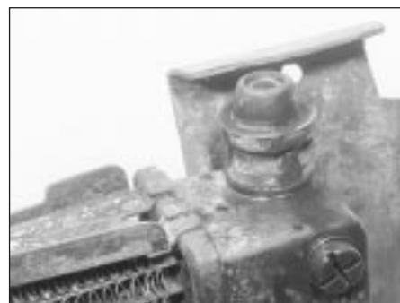
7.9A Radiator mounting rubber
