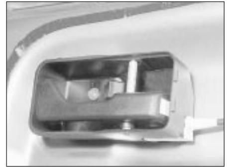
15.5 Inner door release and retaining screw
