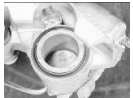
3.19 Piston and dust seal in position in the caliper
