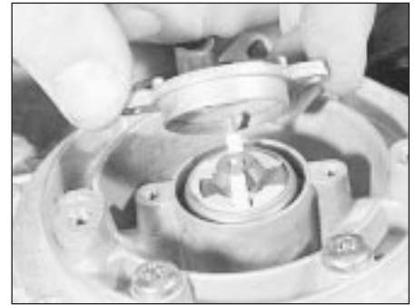
15.9B . . . and remove the injector retaining collar
