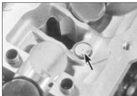
8.24 Cylinder head oil-retaining valve (arrowed)
