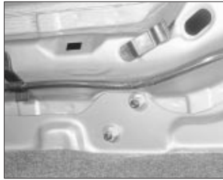
6.10A Rear bumper retaining nuts (Hatchback and Saloon models)
