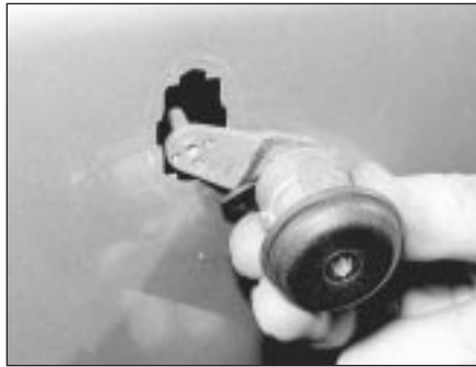
15.2B . . . and withdraw the lock barrel from the door
