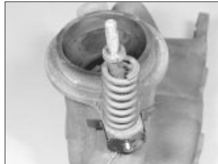
7.12A Showing exhaust downpipe-to-manifold securing bolts - note coil spring, and shoulder on bolt
