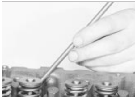
10.17 Withdraw the pushrods
