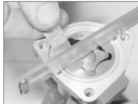
16.4C Checking the rotor endfloat
