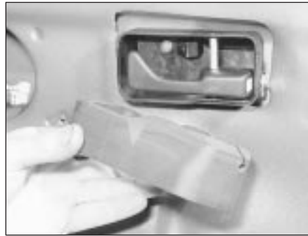
10.6A Remove the insulation surrounding the inner release handle
