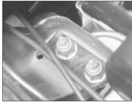
19.18 Engine right-hand mounting-to-body retaining nuts
