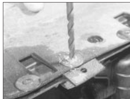
7.9B Drilling out a radiator-to-splash shield rivet
