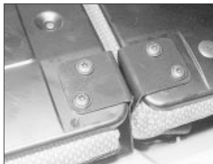
32.4 Rear seat backrest-to-cushion hinge screws
