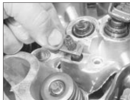
13.5D ... and spacer plate
