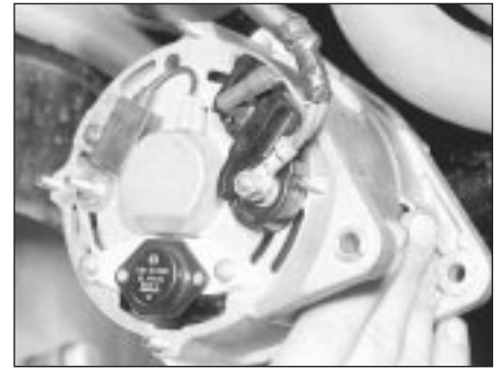
13.9 Alternator removal (CVH engine shown)
