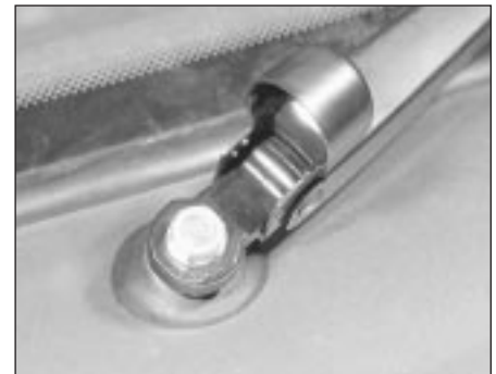
15.2 Windscreen wiper arm retaining nut
