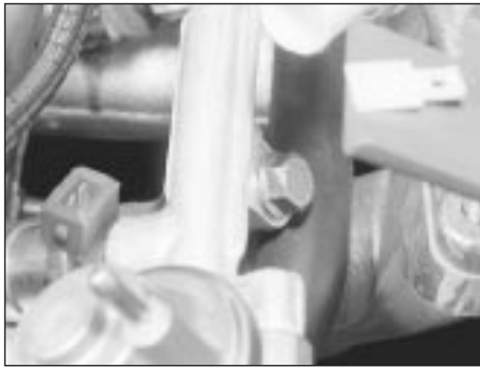
16.13A Remove the injector rail retaining bolts . . .
