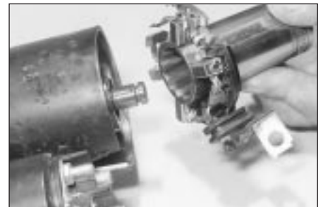
18.9 Brush plate unit assembled over a socket with the same outside diameter as the commutator to ease assembly
