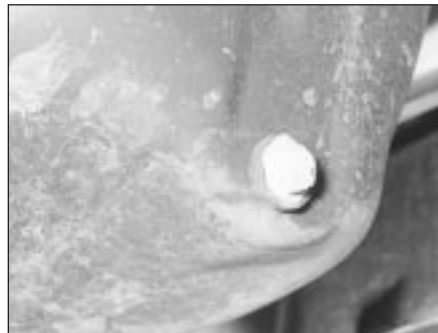
16.7A Engine oil drain plug location in the sump on HCS and CVH engines
