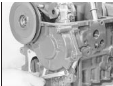
12.7 Fitting the timing chain cover. Crankshaft pulley used as aid to centring
