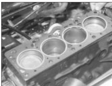
14.22B . . . and locate it over the dowels
