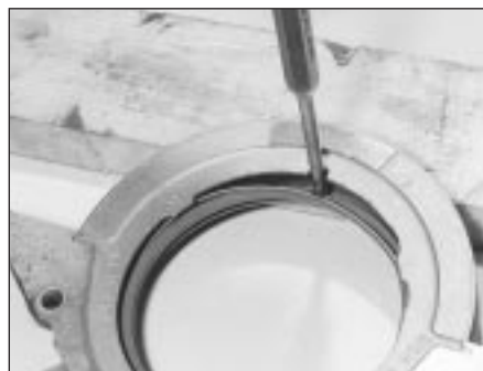
18.18 Rear oil seal removal
