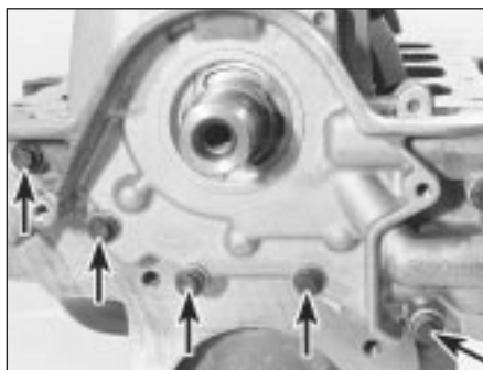
16.5 Unscrew bolts (arrowed) to remove oil pump
