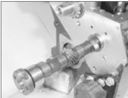
11.7 Withdrawing the camshaft from the front of the engine
