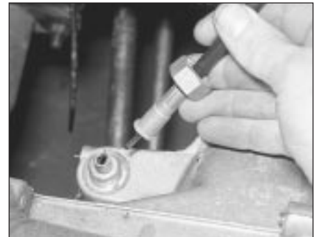
11.50 Disconnecting the speedometer cable - HCS engine
