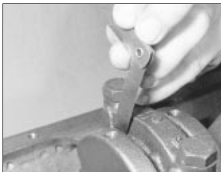
15.9 Using feeler blades to check crankshaft endfloat
