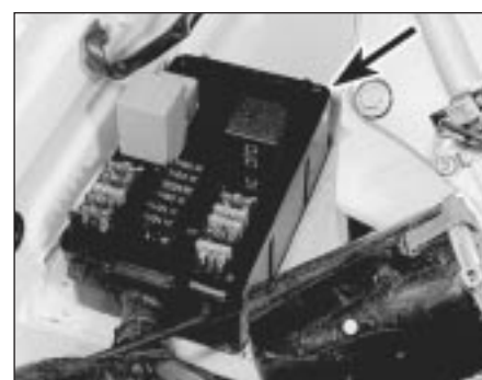
3.2b Fusebox location (arrowed) on engine compartment bulkhead - cover removed to show fuses and relays
