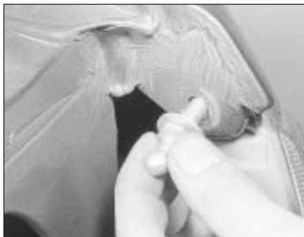
7.8b . . . and the ball-headed bolt
