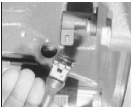
7.4 Disconnecting the engine speed sensor wiring plug - DIS
