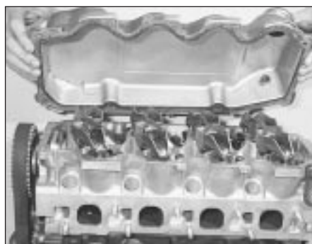
12.13 Remove the rocker cover
