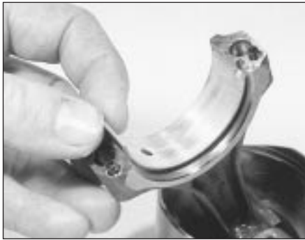
9.11 Fitting the bearing shell in the connecting rod
