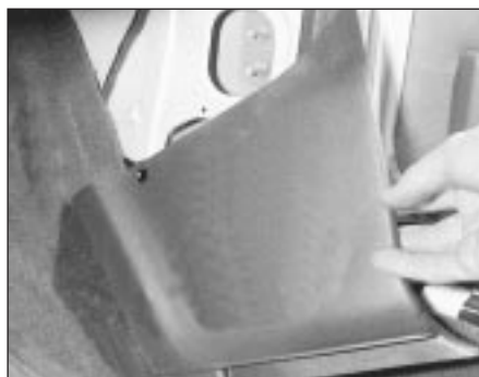
32.8 Removing cowl side trim panel
