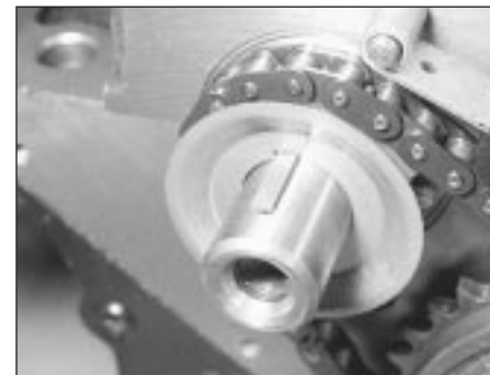
15.15 Fit the oil slinger with its convex side against the sprocket
