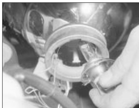
5.3 Headlamp bulb removal
