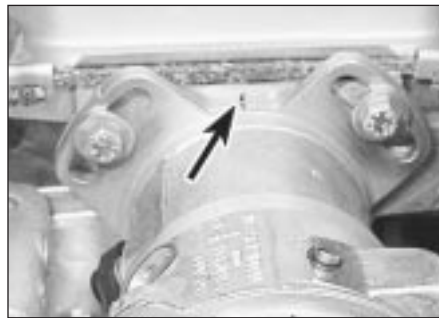
5.45a Distributor mounting flange and cylinder head punch marks (arrowed) - CVH engines (electronic breakerless system - early type distributor shown)
