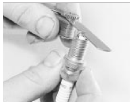
15.9 Measuring the spark plug gap with a feeler blade
