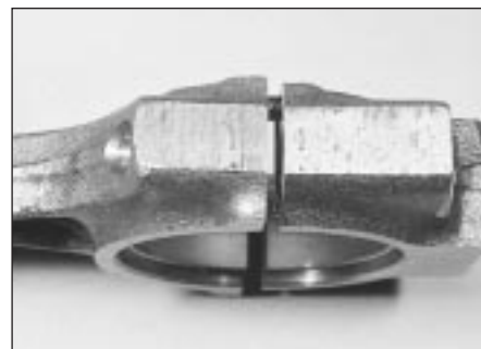
12.37 Connecting rod and big-end cap markings
