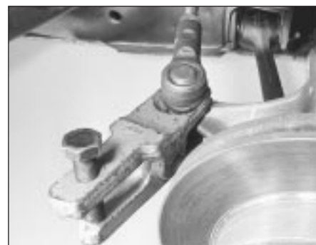
20.6 Releasing tie-rod balljoint using separator tool
