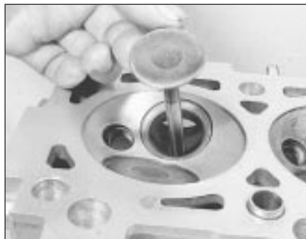
13.36 Inserting a valve into its guide
