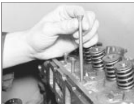
12.13 Keep the pushrods in strict order after removal
