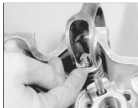
13.38 Compress the spring and fit the collets
