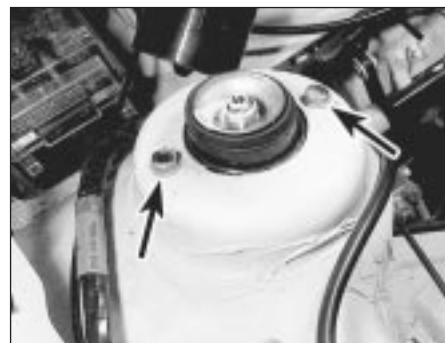
7.4a Suspension strut-to-turret mounting bolts on pre-1983 models
