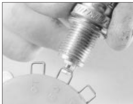
15.10a Measuring the spark plug gap with a wire gauge . . .
