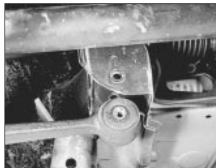
3.3 Suspension lower arm disconnected at inboard end
