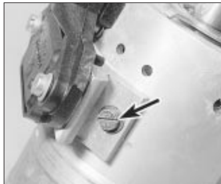
6.3a Electronic amplifier securing screw (arrowed) - later type Bosch distributor
