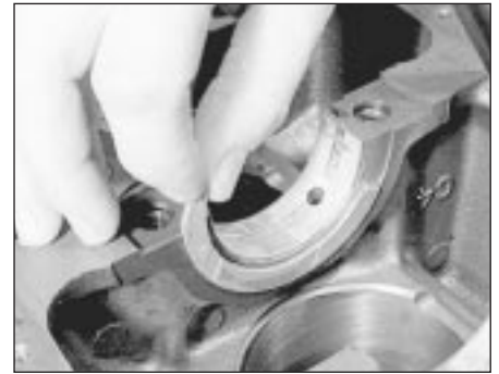
15.3 Locating the crankshaft thrustwashers on the centre main bearing
