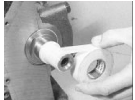
15.11 Using masking tape to eliminate the step on the crankshaft
