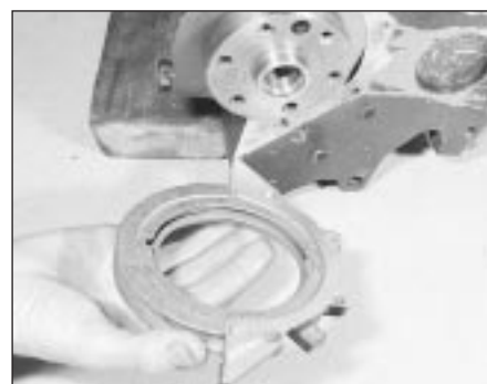
15.20 Crankshaft rear oil seal retainer with new seal prior to fitting
