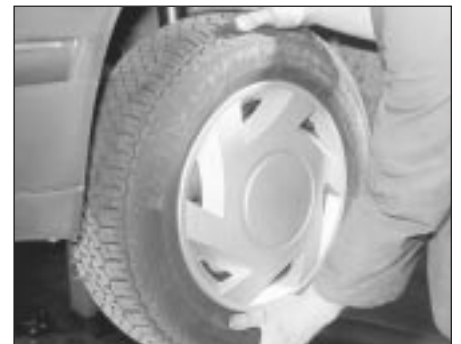
18.3 Rocking the roadwheel to check steering/suspension components
